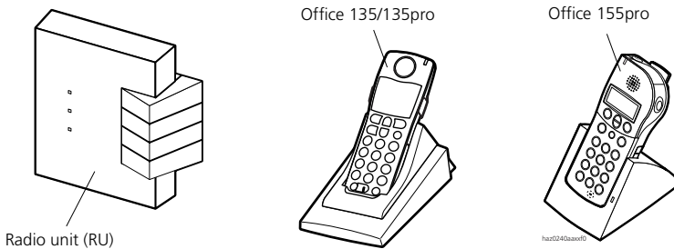
Fig. 1.41: DECT radio unit and Office handsets
