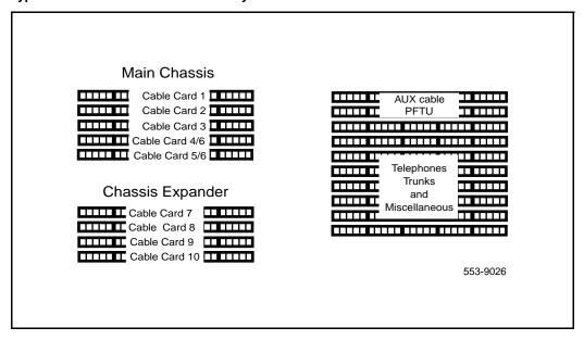
*Note:* One 25-pair cable contains Card 4 and Card 6 (units 0-7). Another 25-pair cable contains Card 5 and Card 6 (units 8-15).
