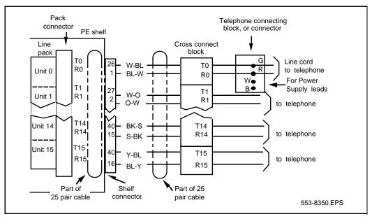
Figure 67 48-port Digital Line Card cross connections
