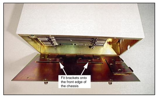
**b** Move the faceplate down so that it fits over the raised edge at the bottom of the chassis. See Figure 17.
