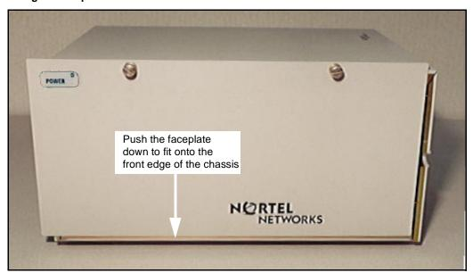
**c** Slide the faceplate to the right, and tighten the quick-release screws into the two holes at the top of the chassis. See Figure 18.
