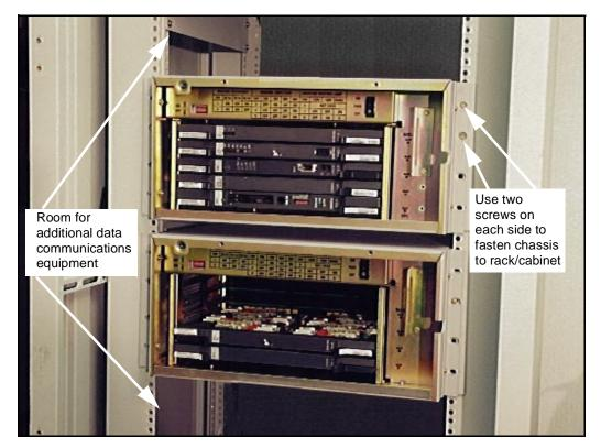
7 If you want to add a Chassis Expander, follow the above steps. You only need to leave a small space between the Main Chassis and the Chassis Expander. The air circulates from the side of the chassis. To install the Chassis Expander, start in the next 5u pattern of mounting holes. This results in the Chassis Expander being approximately 1/4 inch from the first chassis.
