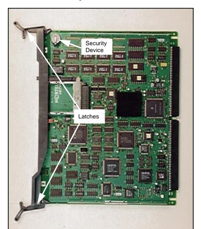
Figure 43 MSC card with the security device installed
