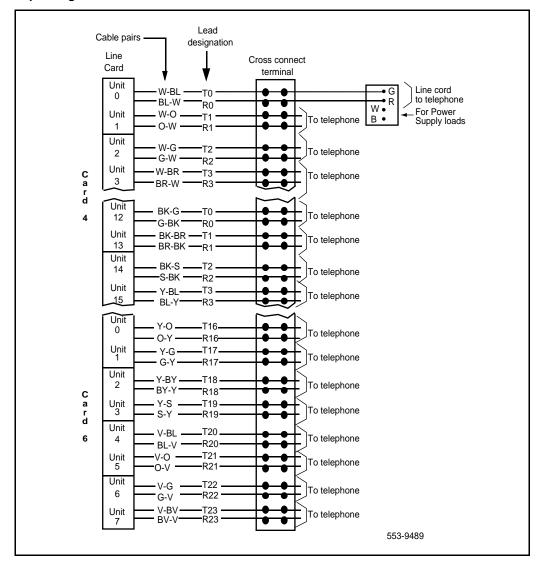
*Note:* Figure 67 is an example which shows the cross connections for the Card 4/Card 6 connector. The Card 5/Card 6 connector provides cable pairs for Card 5 units 0-15 and Card 6 units 8-15.
