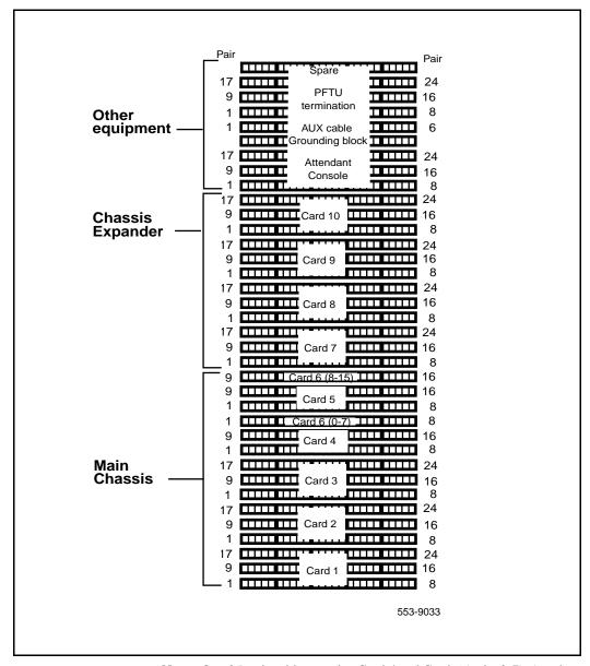
*Note:* One 25-pair cable contains Card 4 and Card 6 (units 0-7). Another 25-pair cable contains Card 5 and Card 6 (units 8-15).
