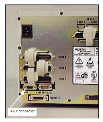
Terminate the AUX cable at the cross connect terminal, according to Table 34.
