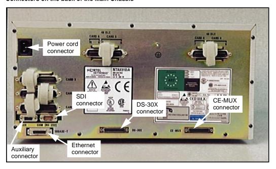
Figure 4 shows the connectors on the back of the Chassis Expander.
