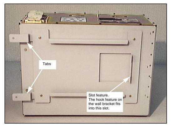
4 Lift the chassis into place so that the slot on the chassis bracket engages the hook feature on the wall bracket.
