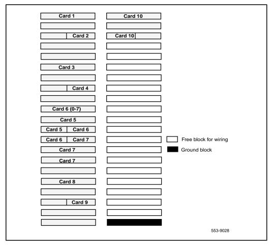
*Note:* One 25-pair cable contains Card 4 and Card 6 (units 0-7). Another 25-pair cable contains Card 5 and Card 6 (units 8-15).
