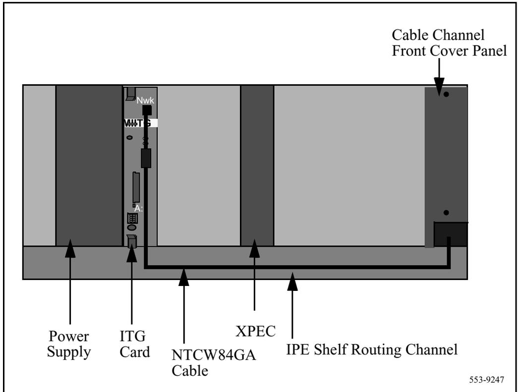
Once the cable has been routed around to the back of the IPE shelf, the RJ45 end of the cable should be inserted into one of the two available shielded RJ45 coupler on the I/O Mounting Bracket as indicated in Figure 48 on page 183.
