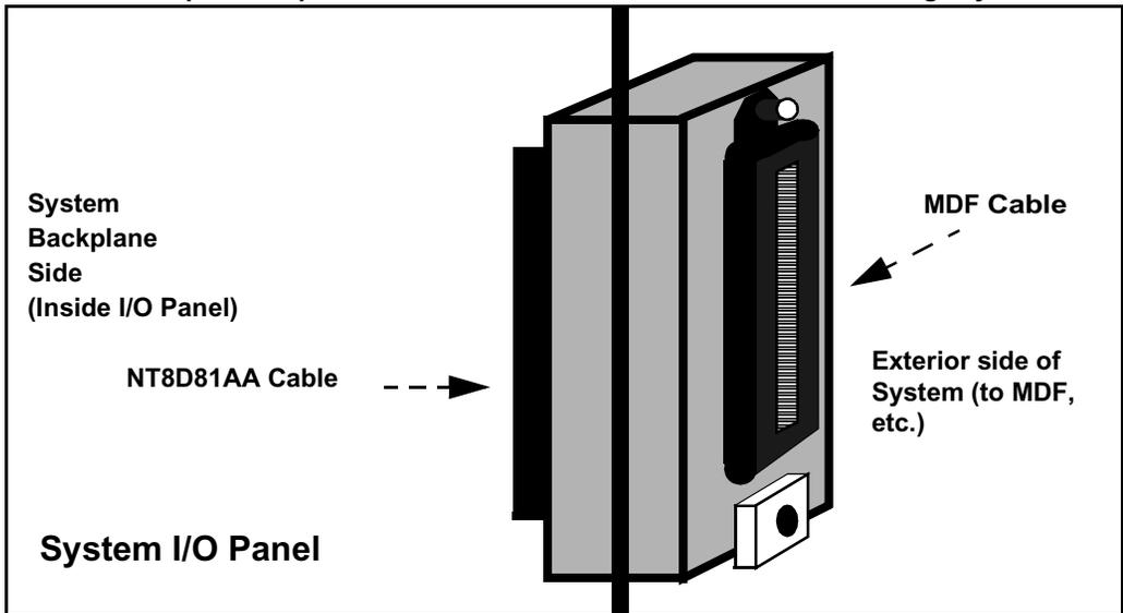
**Install the NTMF94EA ELAN, TLAN, serial interface cable**
