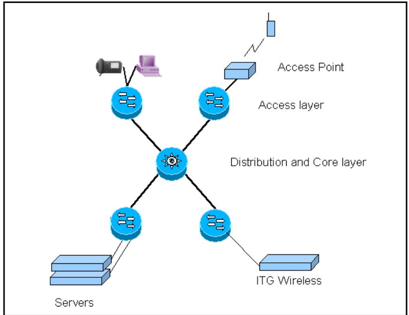
Figure 7 on page 48 is an example of a mid-size campus network design.
