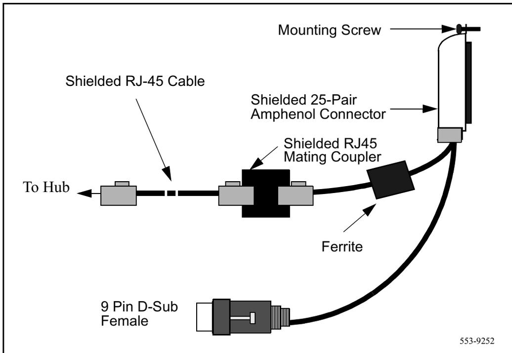
It is very important that the 50-pin connector of the NTMF94BA cable be secured to the I/O connector using the mounting screw provided on the top of the 50-pin connector, as well fasteners on the bottom, in order to tie the shield of the LAN cable to the Meridian 1 and Succession CSE 1000 frame ground for EMC compliance.
