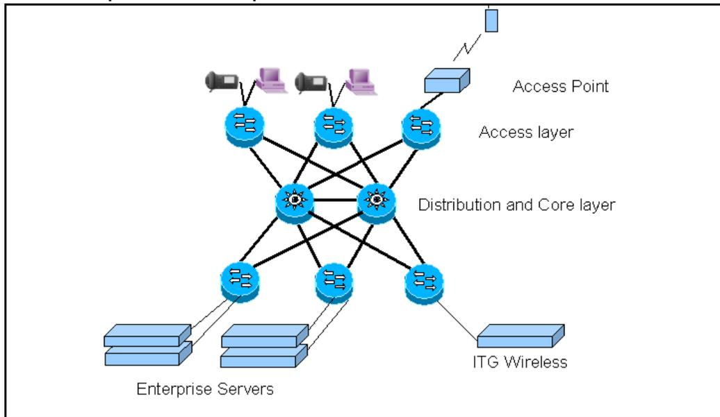
Figure 8 on page 49 is an example of a large campus network design.
