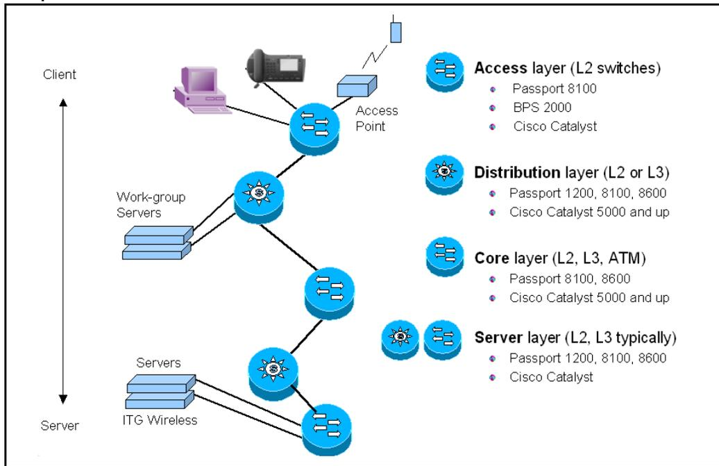
The following figures provide examples of logical connection diagrams for small, medium, and large campus networks. Other network designs can also be used. The actual design that is implemented depends on many factors, including physical locations, size, and scalability.
