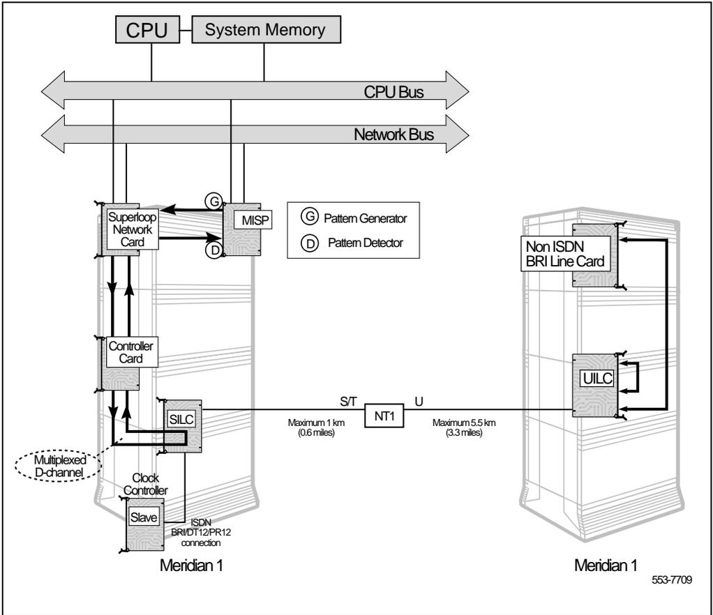
The following steps are used to perform the remote loopback test for a ISDN BRI trunk DSL provisioned as a MCDN Tie configuration:
