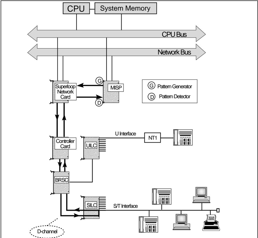
Before starting loopback testing at the SILC or UILC, disable the card to be tested; when the card is disabled, the system disconnects all the calls handled at the time by that card. Perform the following steps:
