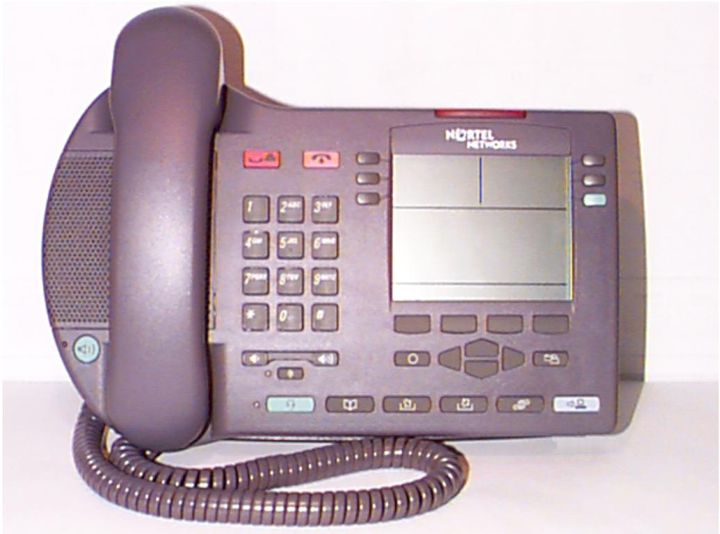
The i2004 Internet Telephone allows you to make calls using your company's existing data network. It connects directly to the LAN over a single Ethernet connection. This gives you a direct connection to the LAN, which in turn connects your telephone to your existing data network. The i2004 Internet Telephone translates voice into data packets for transport using the Internet Protocol (IP).
