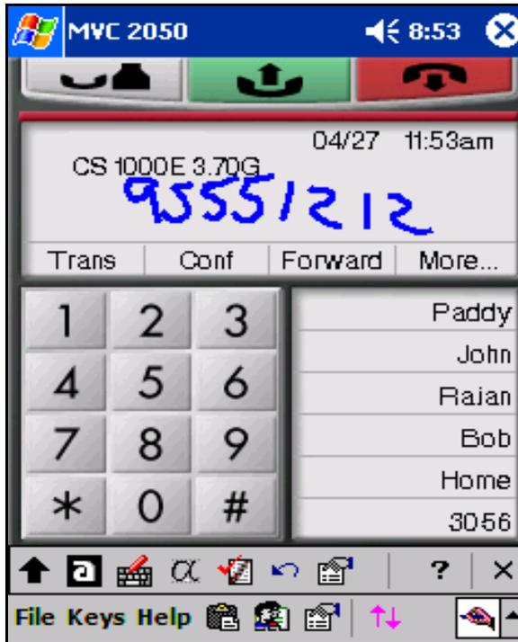
Using the MVC 2050 application, the keyboard can act like a dialpad, interpreting the alphabetical keys as numbers. For instance, if you type a J, K, or L, it is interpreted as a number five (5). Keys which are not alphanumeric are ignored.
