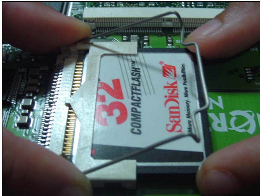
Figure 39 Insert CompactFlash
