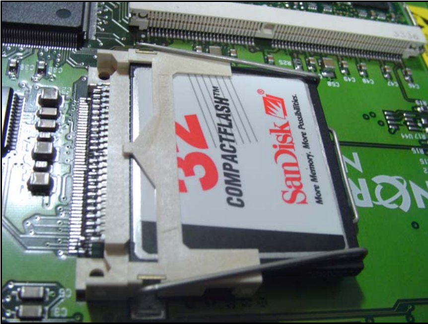
Figure 42 CompactFlash card locked into position
