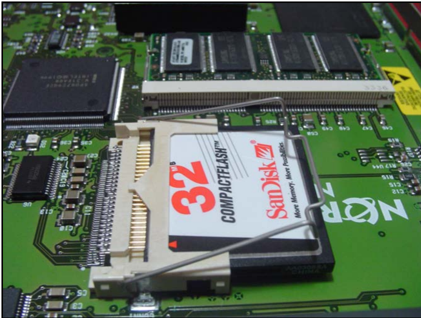
Figure 201 Lift the metal clip on the CompactFlash card
