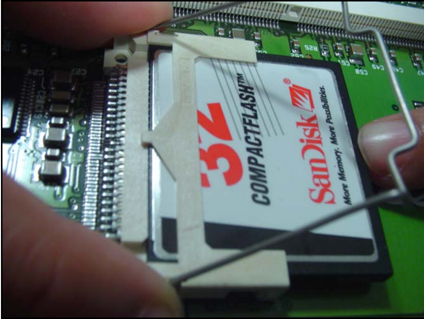
Figure 40 Seat CompactFlash card
