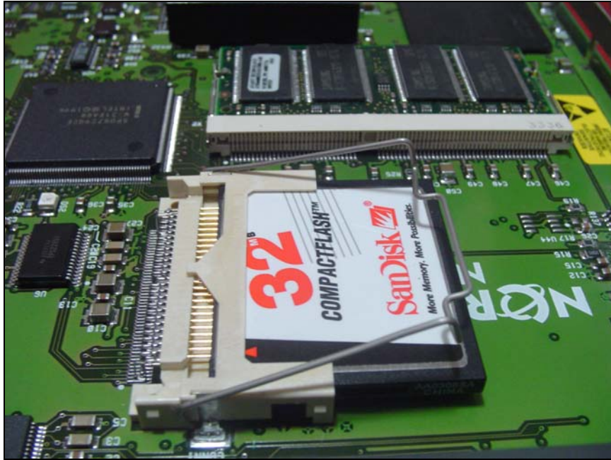
Figure 38 Position the CompactFlash in socket
