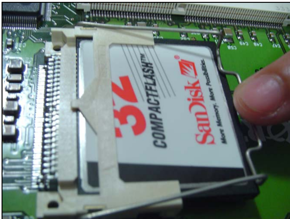
Figure 41 Lock card into place
