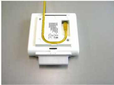
Figure 50 Cable at rear side of the cabinet
