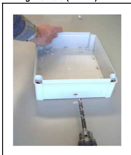
Figure 62 Drilling the hole (12 mm)
