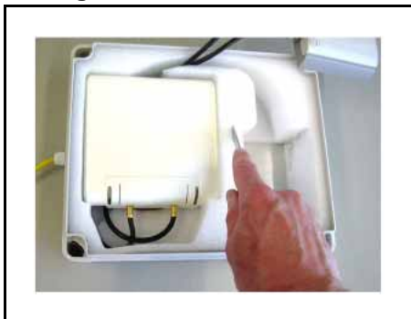
Figure 84 Cutting the foam to allow the antenna to fit into it, in the required position
