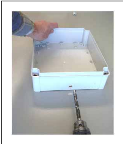
Figure 73 Drilling the hole (12 mm)
