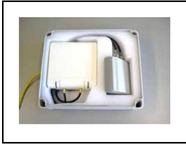
Figure 82 Antenna does not fit into the hole
