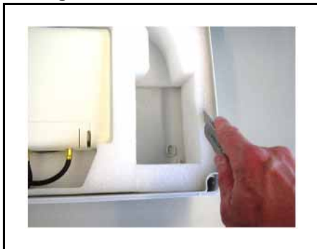
Figure 84 Cutting the foam to allow the antenna to fit into it, in the required position
