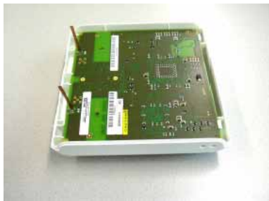
Figure 44 Bend Antennas carefully into vertical position
