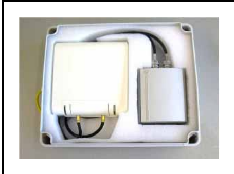
Figure 85 4720 DAP and directional antenna in their positions
