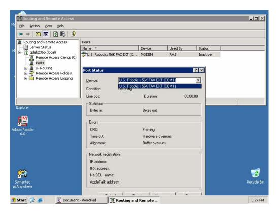
The only method of removing the incorrect modem (e.g. Standard 33600 modem) from RRAS is to remove it from the system.
