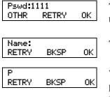
PARTRIDGE RETRY BKSP OK This is an example of a display with fewer than 16 characters, where the command line prompt remains on the display.
