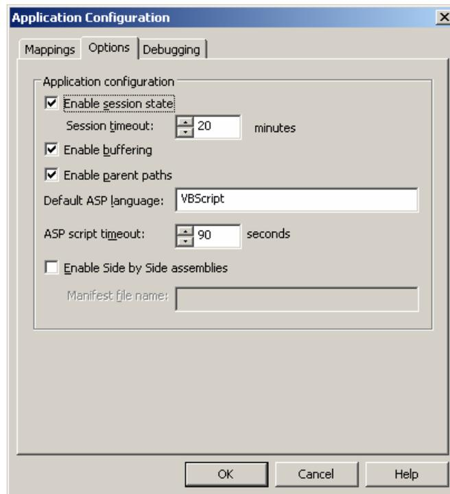
Figure 22: Options Page with the Enable parent paths option selected
