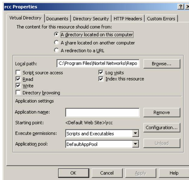
**Figure 30: RCC Properties - Application Pool**
