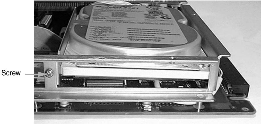
**Note:** On some versions of the 200i server, the SCSI cable is routed around the outside edge of the stiffener. In this situation, lift the SCSI cable over the top of the stiffener so that you can access the screws that secure the hard drive.
