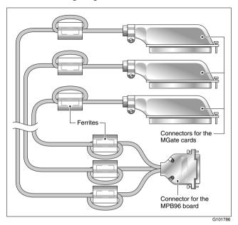
**Note:** The ferrites on this cable control EMC emission levels. Do not remove them.
