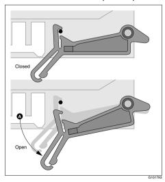
**3** Slide the MGate card into the assigned slot on the switch.
