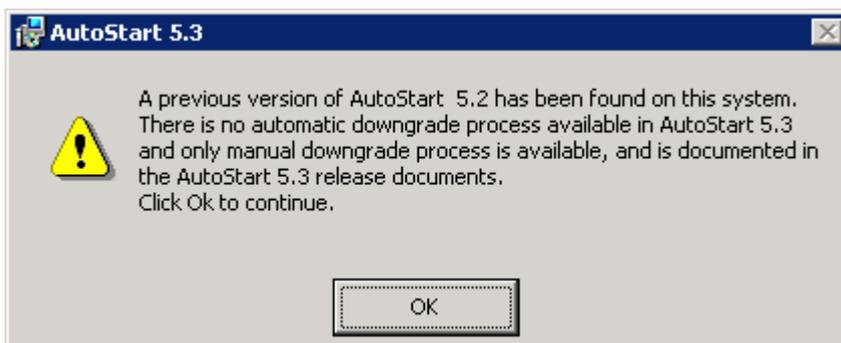
3.7. AutoStart installation will inform us about manual downgrade process. Press the “OK” button to close pop-up window.
