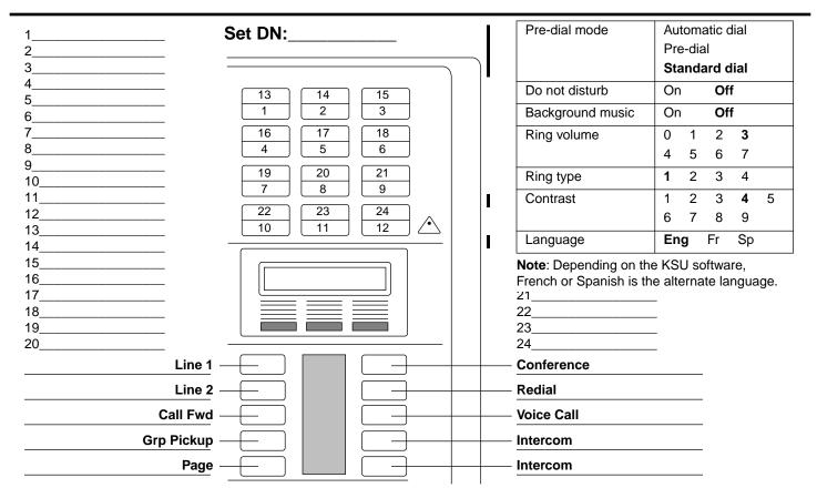
Note: Dual memory buttons (1 through 24) can be programmed with features, or internal and external autohold numbers.
