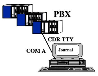
The PC running the Journal application uses one COM port (Default COM 1, baud 1200, 7 bit, even parity and 1 stop) to connect to the PBX Call Detail Record TTY port. The two ports likely need a null modem adapter between them since the PC is normally a male 9 pin DTE (Data Terminal Ready) and the PBX TTY is a male 25 pin DTE. The cables to connect the two must be provided by the installer. The PC COM port software settings must match the PBX CDR port settings.
