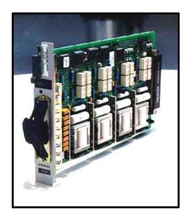
This circuit card is new with the Option 11C Compact. The NTMW44 is a 4 port analog trunk mini peripheral card. This card is based on the NTMW07 4UT/4MLC combo card. It has one printed circuit board which holds 4 analog trunk units and unlike the combo card it does not have a Message Waiting Line Card daughterboard. This card can be located in any card slot location of any cabinet.
