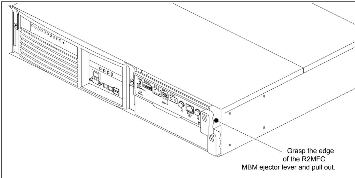
**Figure 10** How to remove a BCM400 R2MFC MBM
