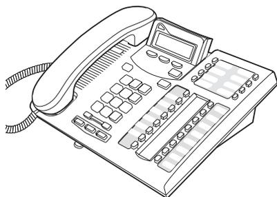
**7316E** — two-line display, three display buttons, 16 memory buttons with indicators, eight memory buttons without indicators.
