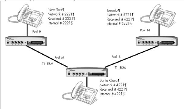
Each system must be running BCM software. Each system must be equipped with target lines and a BCM expansion unit with a DTM with at least one T1 E&M line.
