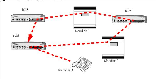
Figure 7 Call loop on system without ICCL
