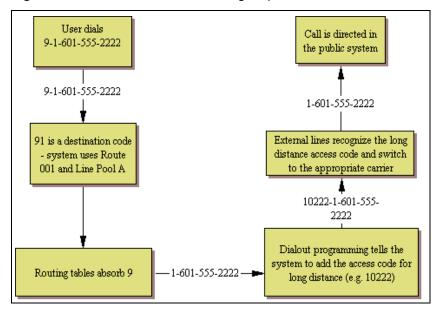
Figure 72 Carrier code call numbering sequence
