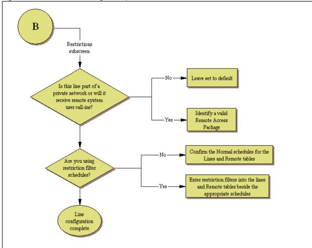
Figure 43 PRI line feature configuration process — Part B
