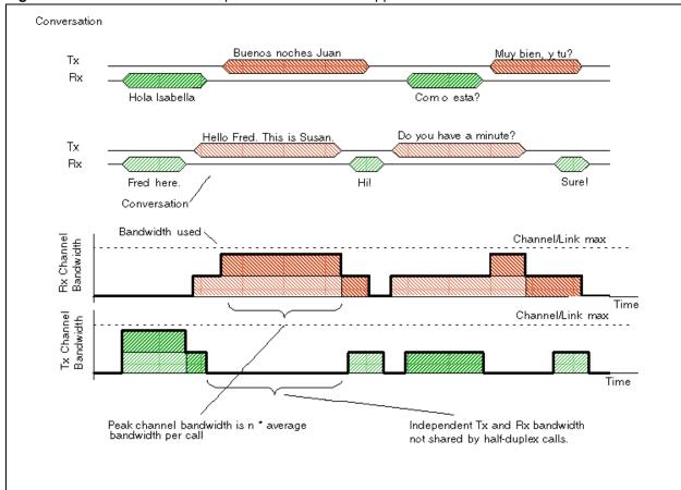
Figure 150 Two calls on a full-duplex link with silence suppression
