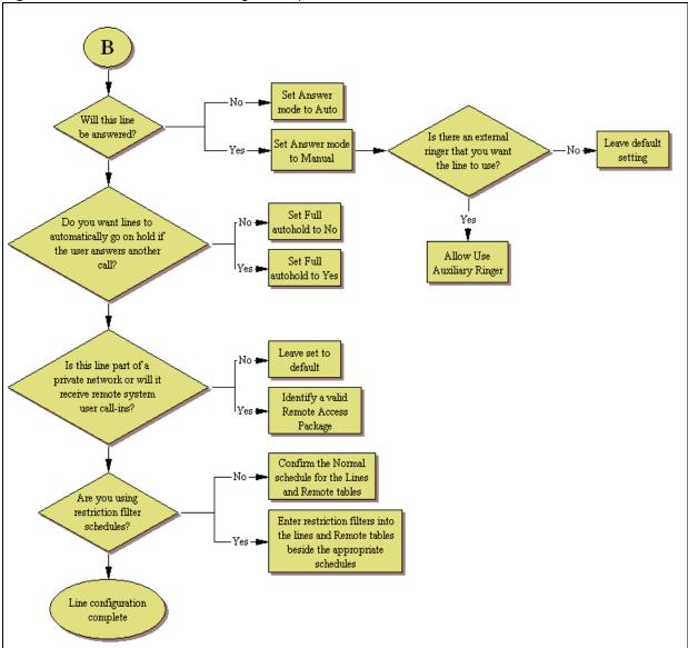
Figure 55 DASS2 line feature configuration process — Part B
