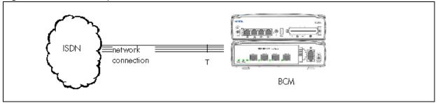
A T loop can be used in combination with an S loop to provide D-packet service for a point-of-sale terminal adapter (POSTA) or other D-packet device. D-packet service is a 16 kbps data transmission service that uses the D-channel of an ISDN line. The T and S loops must be on the same physical module.
