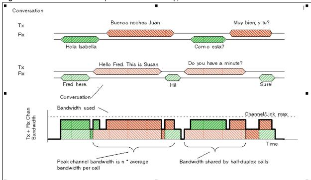
Figure 147 Two calls on a half-duplex link with silence suppression
