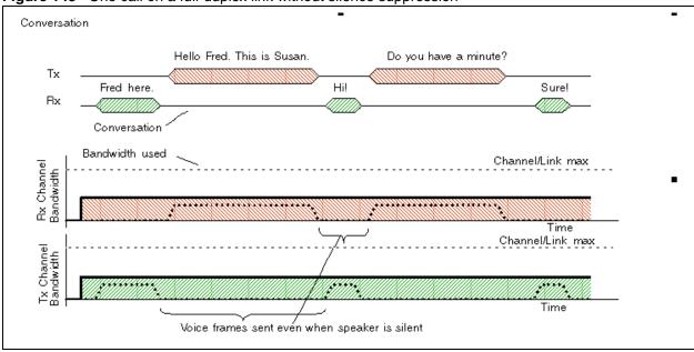
Figure 148 One call on a full-duplex link without silence suppression
