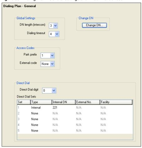
Figure 85 Dialing Plan - General settings and Direct Dial devices
