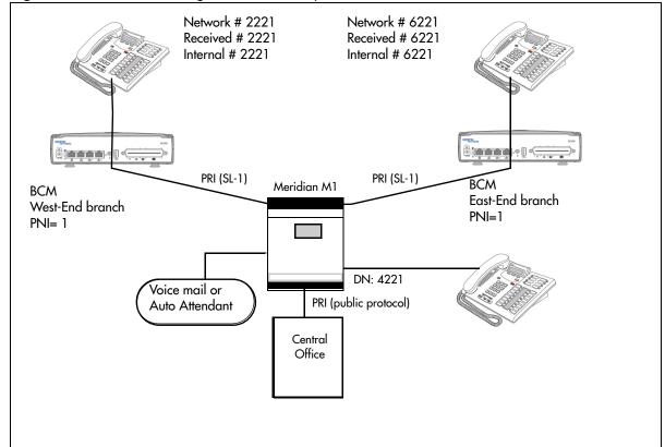
Figure 98 MCDN networking, with a common public network connection
