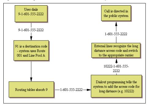
Figure 71 Using destination codes to access another system
