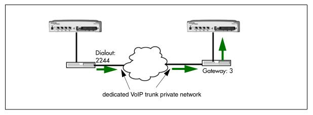
**4** System B recognizes the code as its own, and uses a local target line to route the call to the correct telephone.
