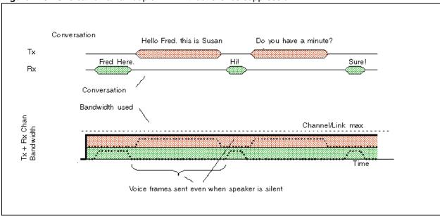
Figure 145 One call on a half-duplex link without silence suppression
