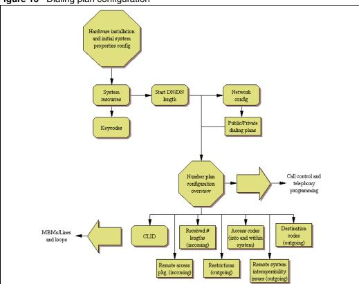
Figure 13 Dialing plan configuration
