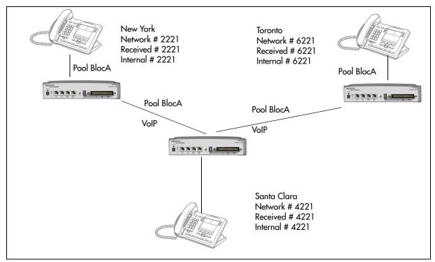
Each system must be running BCM software. Each system must be equipped with target lines and a VoIP keycodes with at least one IP Trunk line. Programming information for this network is shown in Table 72.
