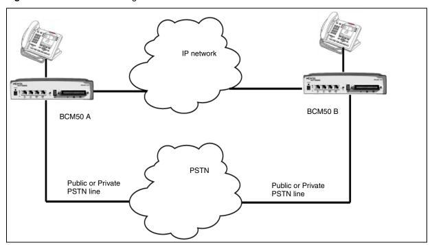
In a network configured for PSTN fallback, there are two connections between a BCM and a remote system.
