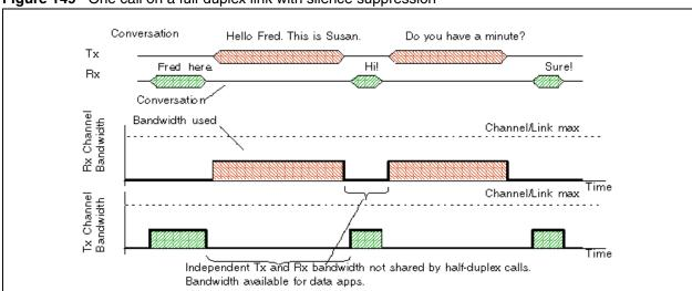
Figure 149 One call on a full-duplex link with silence suppression
