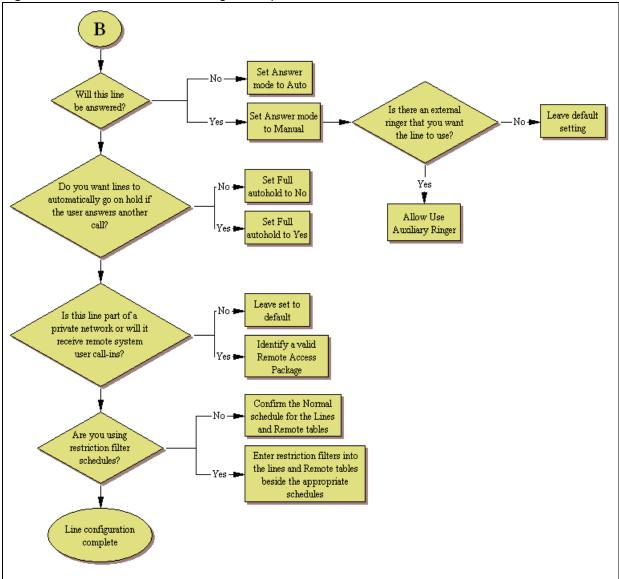
Figure 57 DPNSS line feature configuration process — Part B
