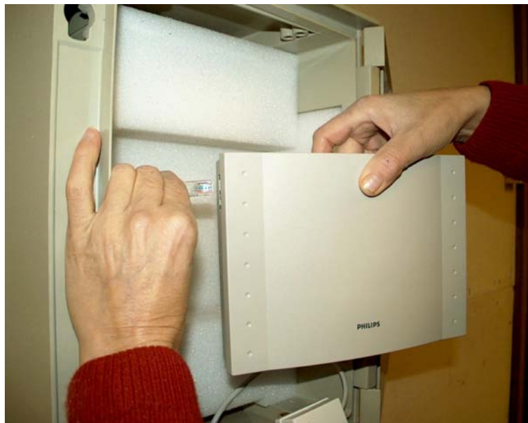
Figure 113 External housing: connect Ethernet CAT5
