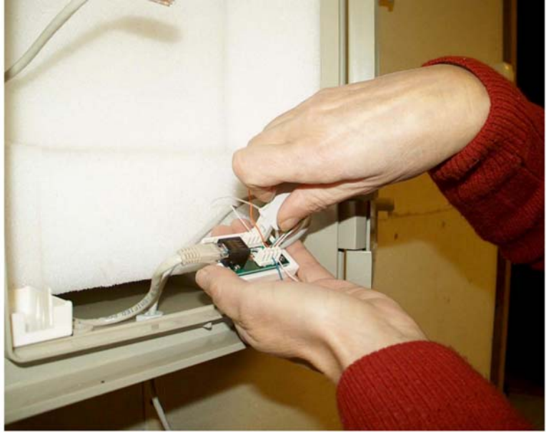
Figure 110 External housing: connect cables
