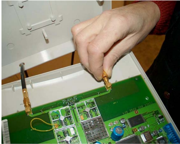
Figure 117 External housing: connection inside the C4010E basestation cabinet
