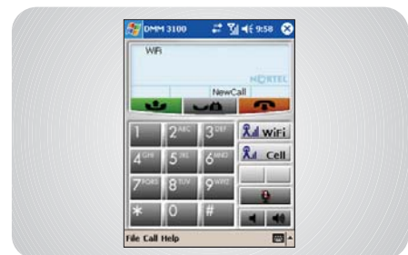
Figure 5. Dual-mode (WLAN and cellular) client for mobile device
