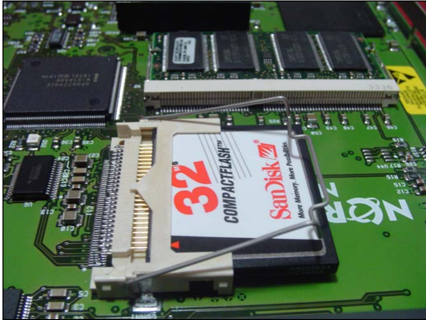
Figure 61 Position the CompactFlash in socket
