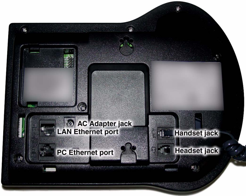
Figure 4: IP Phone connections
