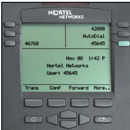
Figure 6: Logged on to an IP Phone 2002 using an IP Phone 2004
