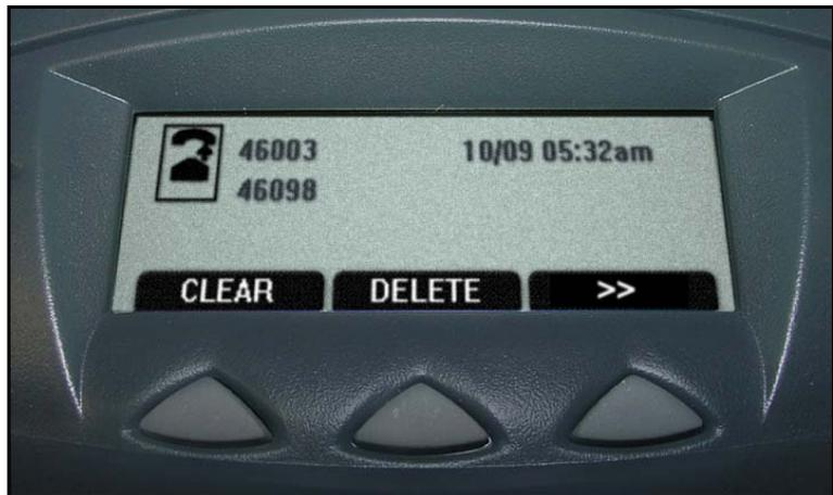
The soft key label has a maximum of six characters. Each soft key includes the soft key label and an icon. When a soft key is in use, a flashing icon displays at the beginning of the soft key label, and the label shifts one
