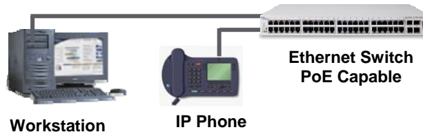
Figure 2: Workstation/phone separate drops to edge switch
