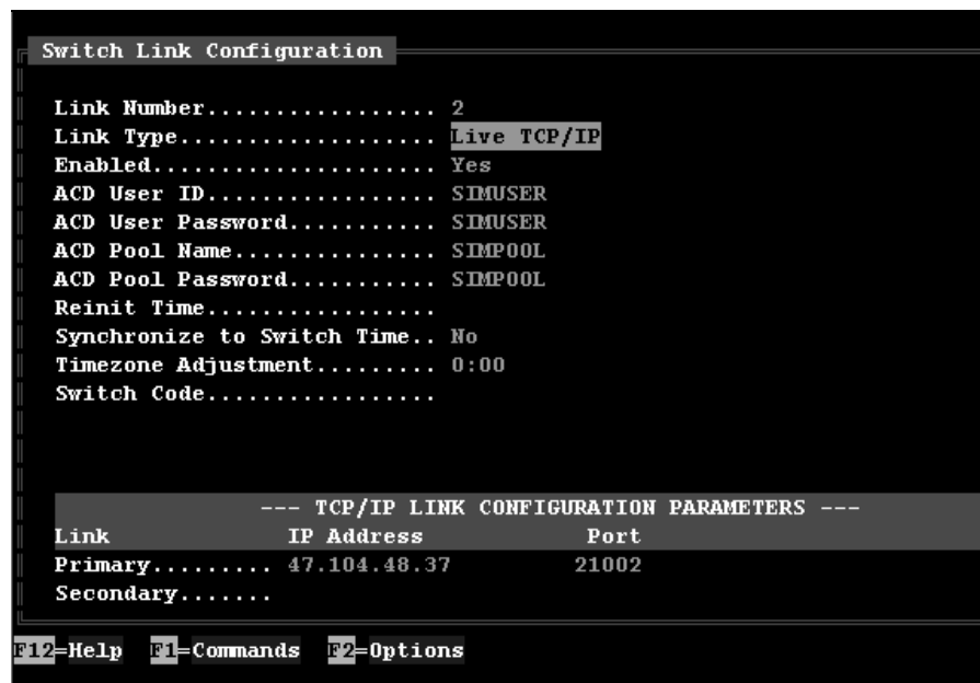
Figure 6.5 Switch link configuration screen - live link
