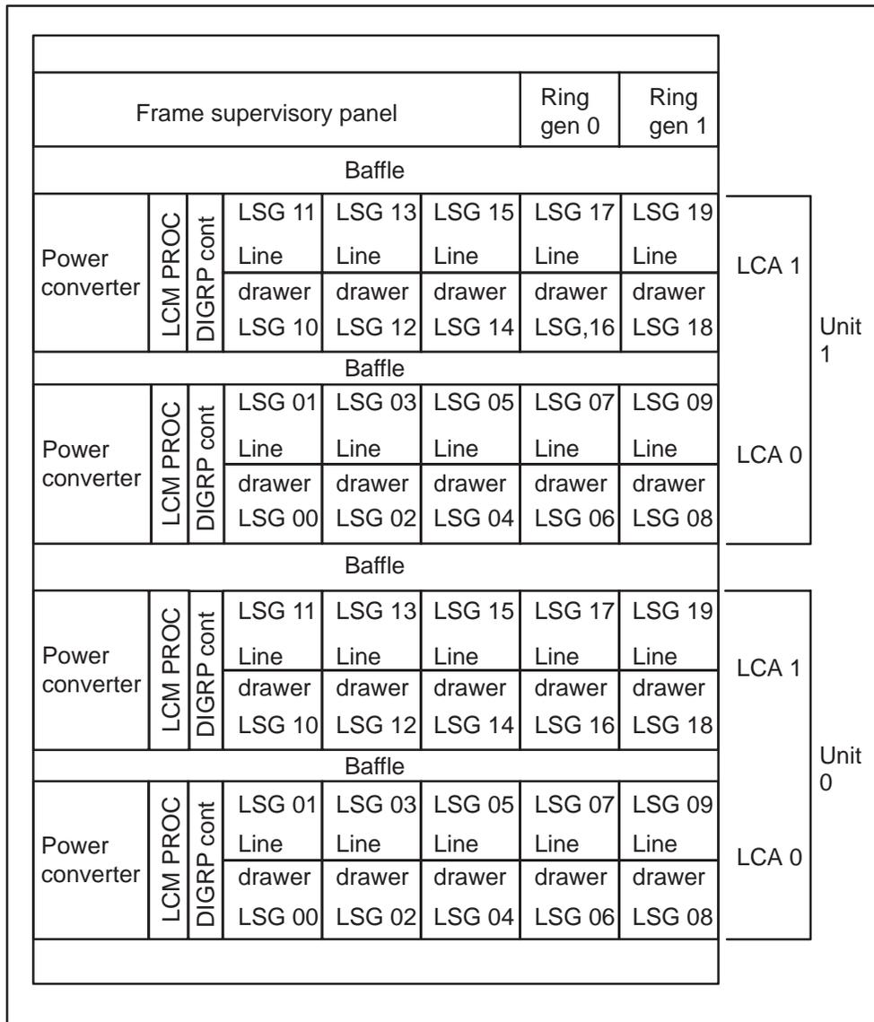
Each digroup control has eight C-side ports. Six of these ports are connected by means of DS30A links to the host line group controller (LGC). Three are in the active mode and three are normally inactive, used only if
