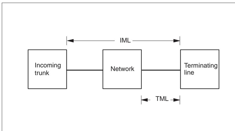
Incoming matching loss is the failure to find a path from an incoming trunk to an idle line. The line concentrating equipment frame table below lists the operational measurements and any associated logs that can be used to evaluate incoming matching loss.
