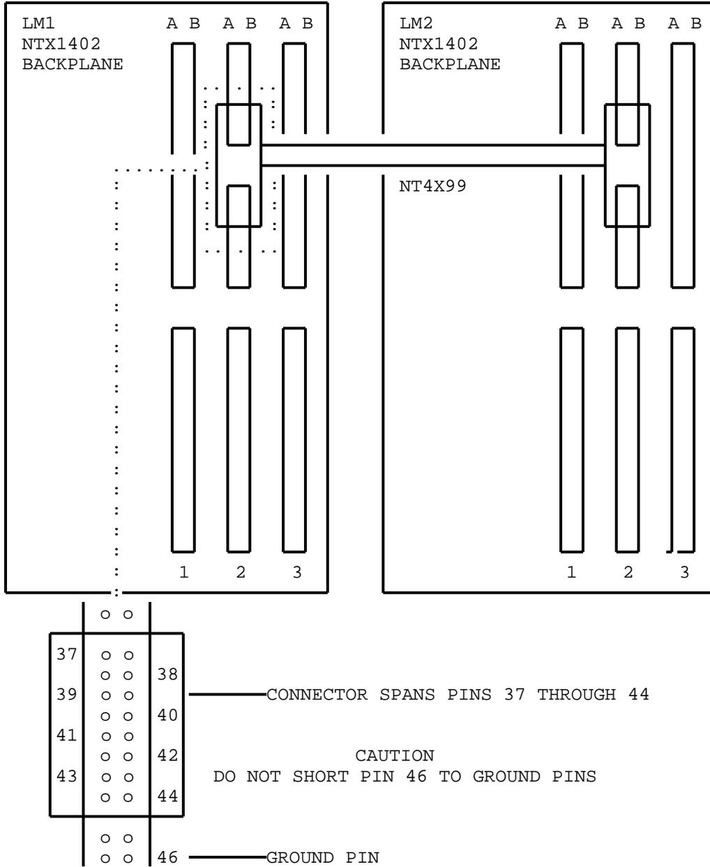
Fig. 7 - Diode Fixture Installation
