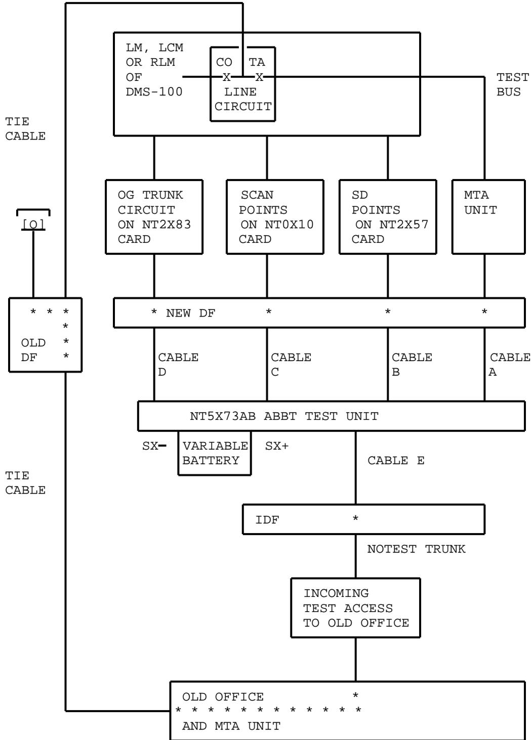
Fig. 1 - General Test Equipment Arrangement for ABBT
