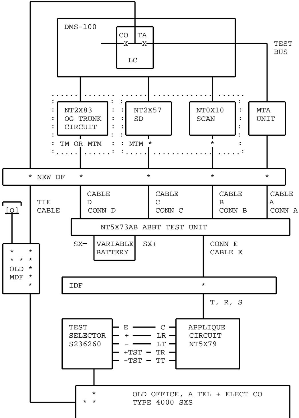
Fig. 10 - ABBT Connections for A TEL + ELECT CO Type 4000 SXS
