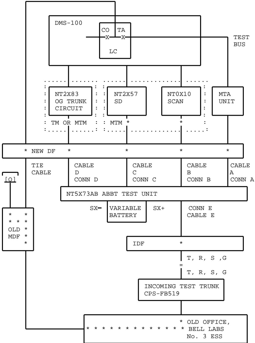
Fig. 16 - ABBT Connections for Bell Laboratories No. 3 ESS
