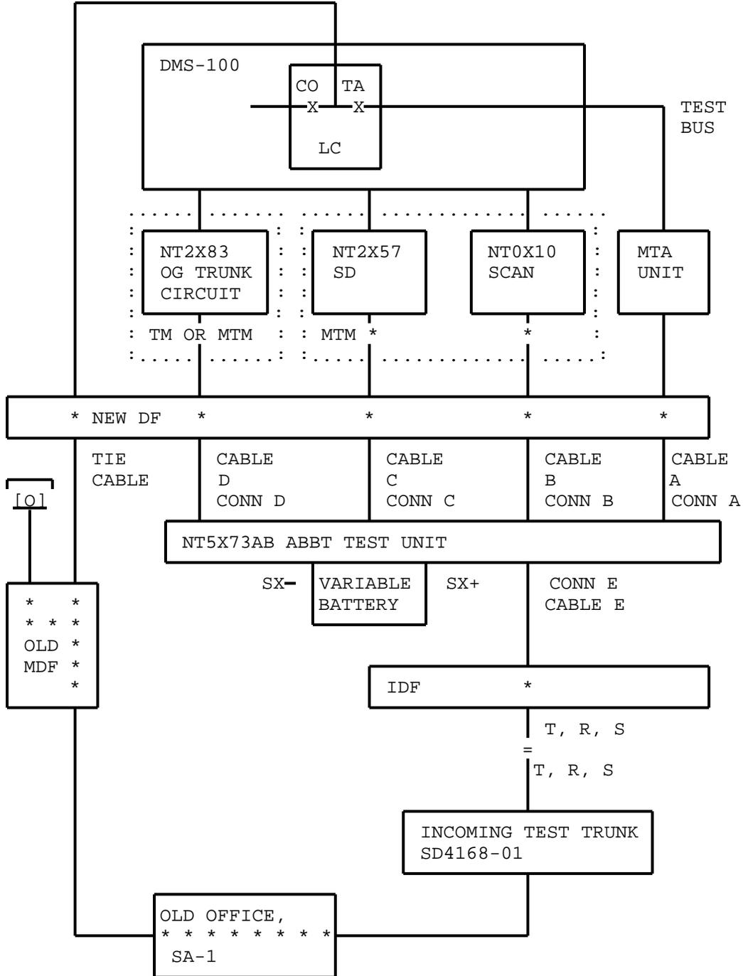
Fig. 28 - ABBT Connections for NTL SA-1 Switches
