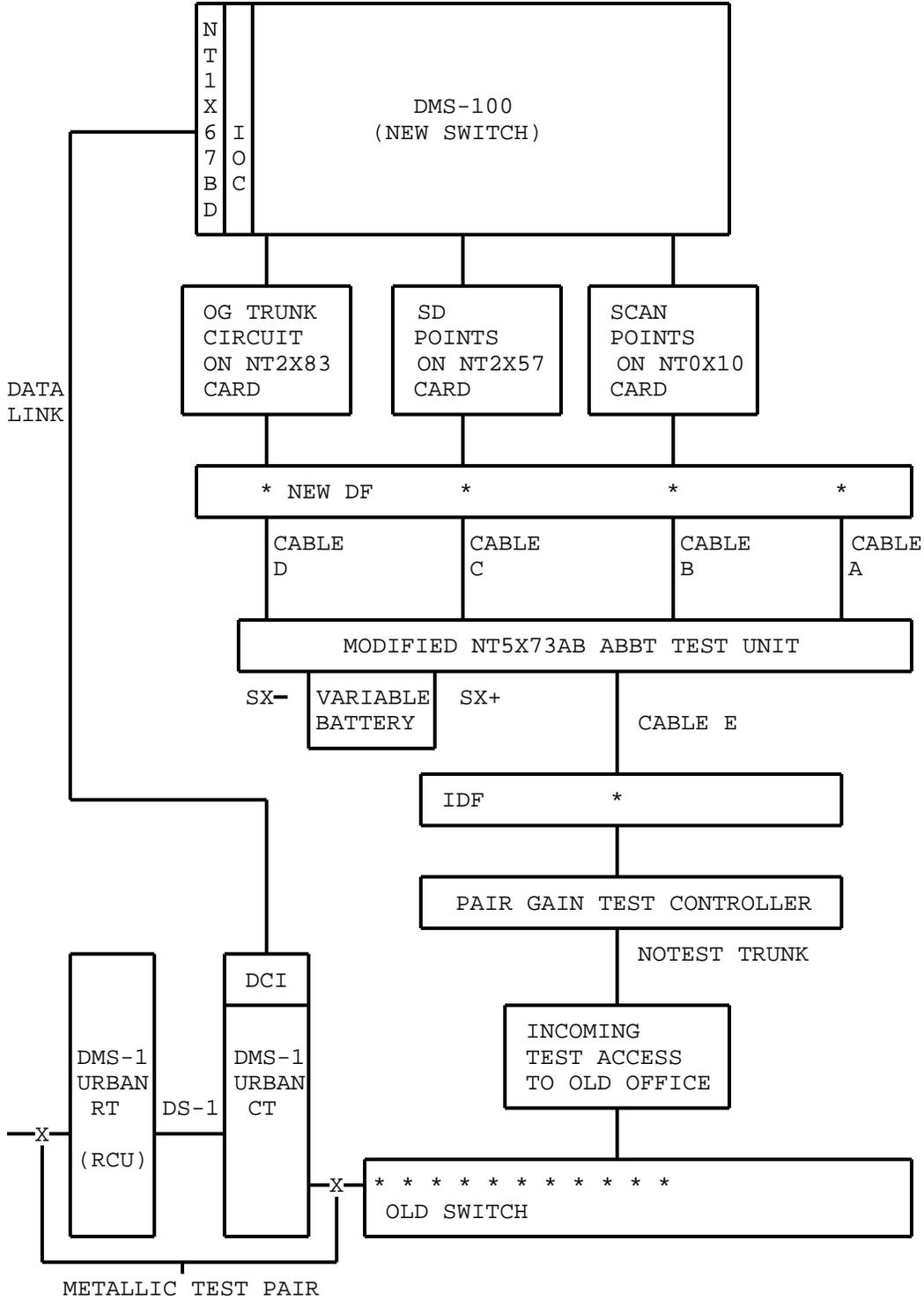
Fig. 37 - ABBT Configuration for RCU Lines With LTA
