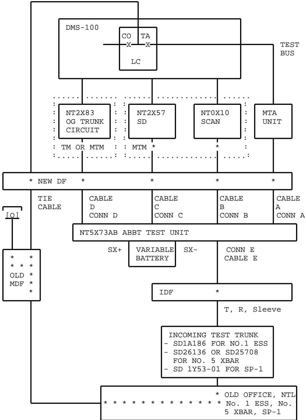
Fig. 27 - ABBT Connections for NTL No. 1 ESS, No. 5 XBAR, SP-1
