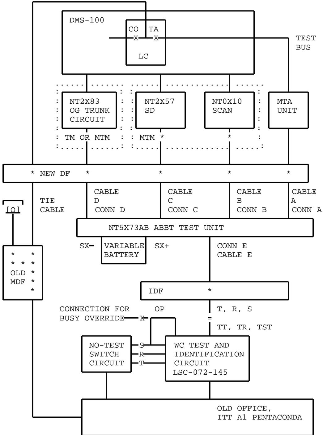
Fig. 19 - ABBT Connections for ITT A1 Pentaconda Switches
