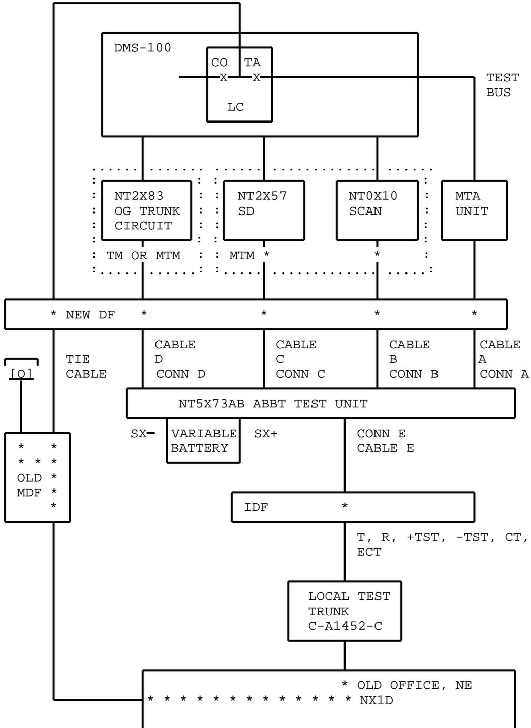
Fig. 24 - ABBT Connections for NE NX1D Switches
