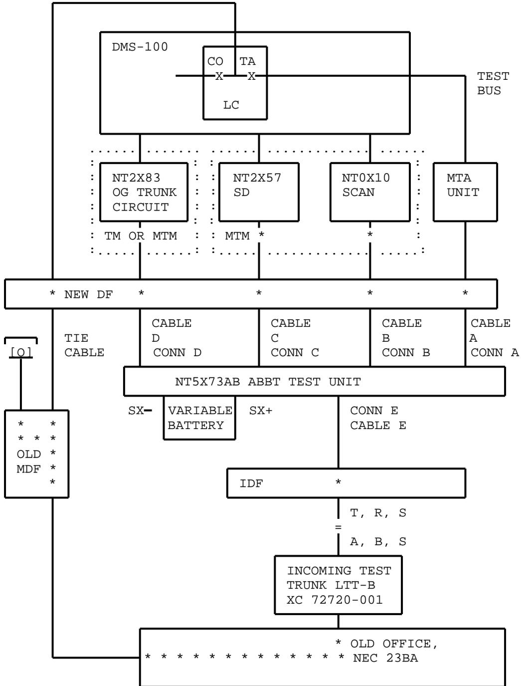
Fig. 23 - ABBT Connections for NEC 23BA Switches
