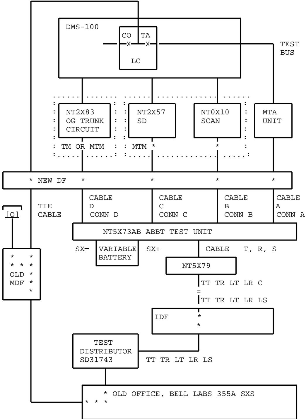
Fig. 15 - ABBT Connections for Bell Laboratories No. 355A SXS
