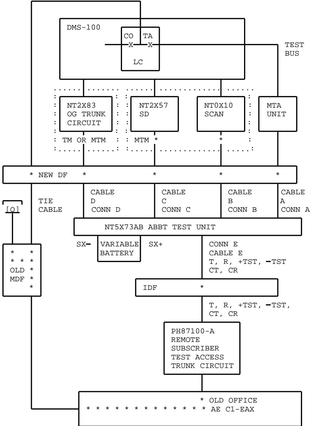
Fig. 12 - ABBT Connections for AE C1-EAX Switches
