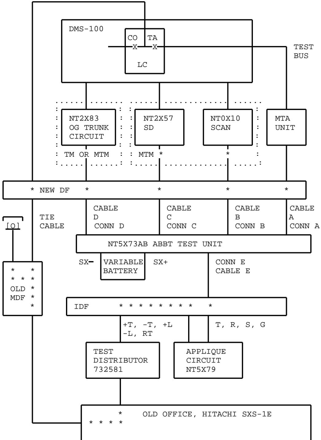
Fig. 18 - ABBT Connections for Hitachi SXS-1E Switches
