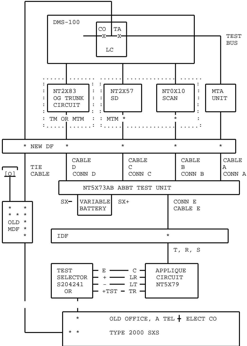
Fig. 9 - ABBT Connections for A TEL + ELECT CO TYPE 2000 SXS
