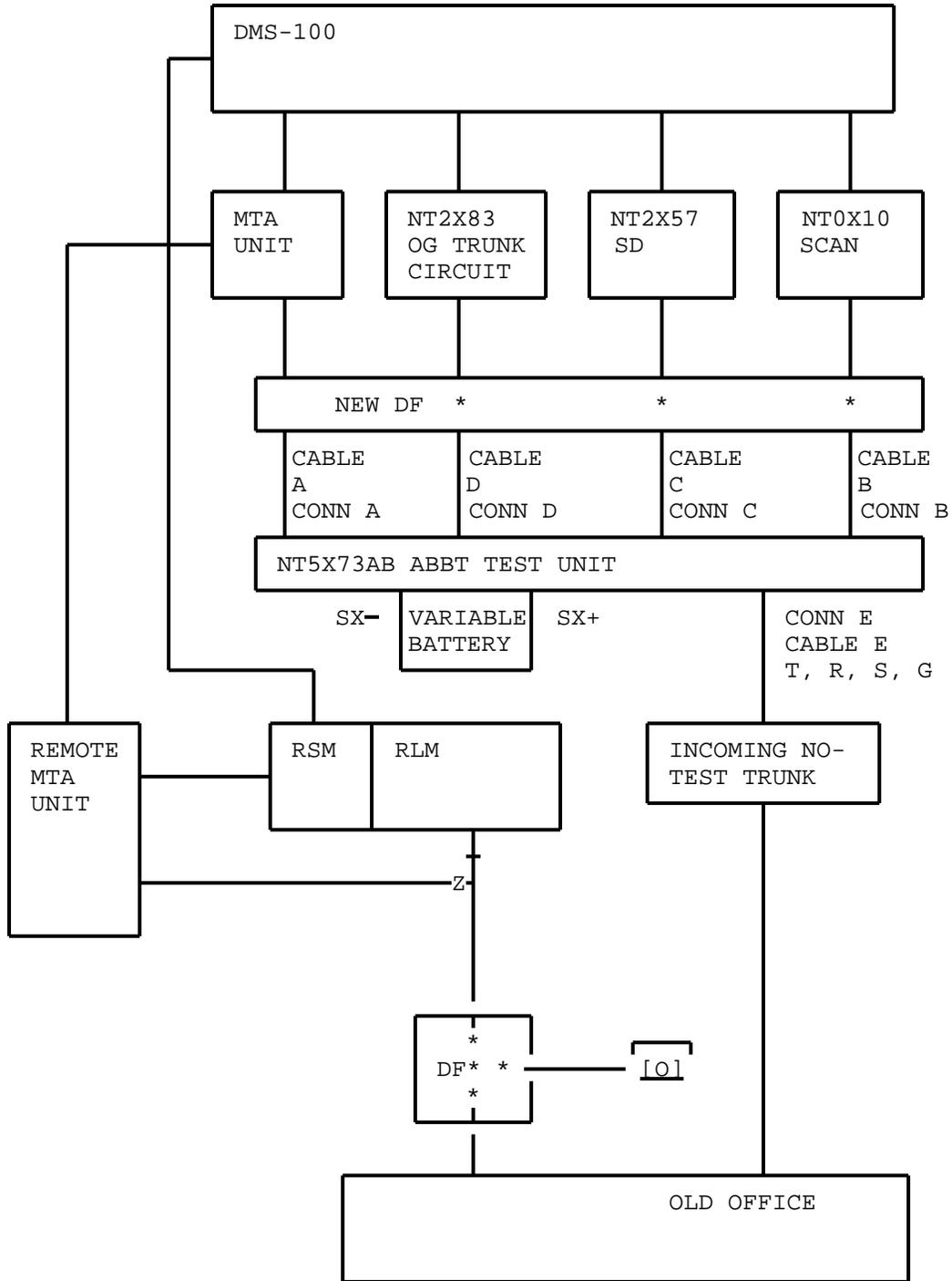
Fig. 34 - ABBT Connections for RLM Within Metallic Range
