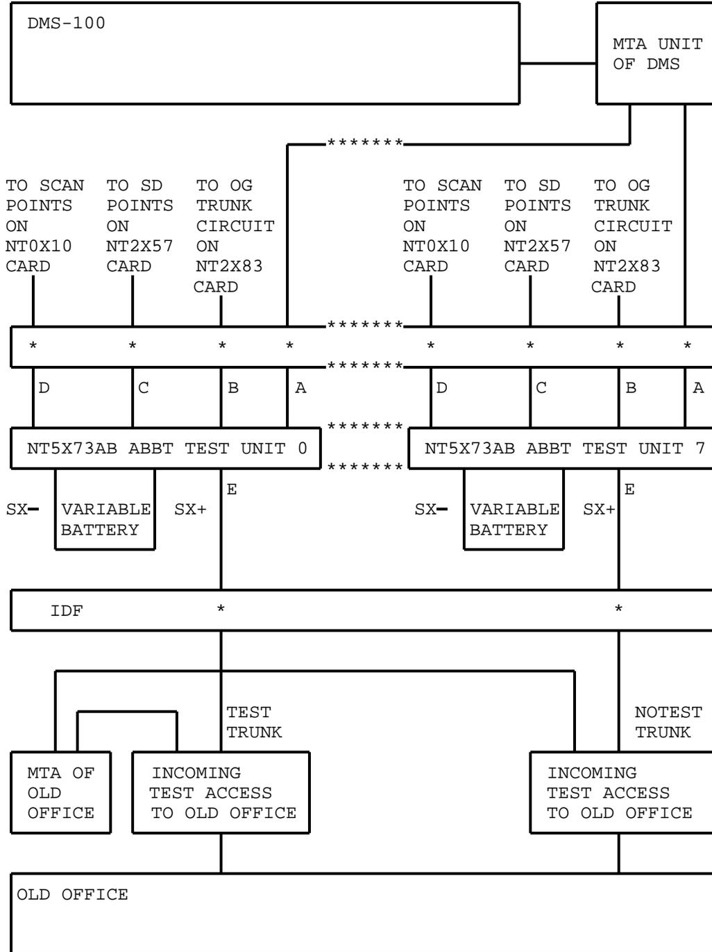
Fig. 5 - General Test Equipment Arrangement for Performing ABBT with more than one NT5X73AB Test Unit
