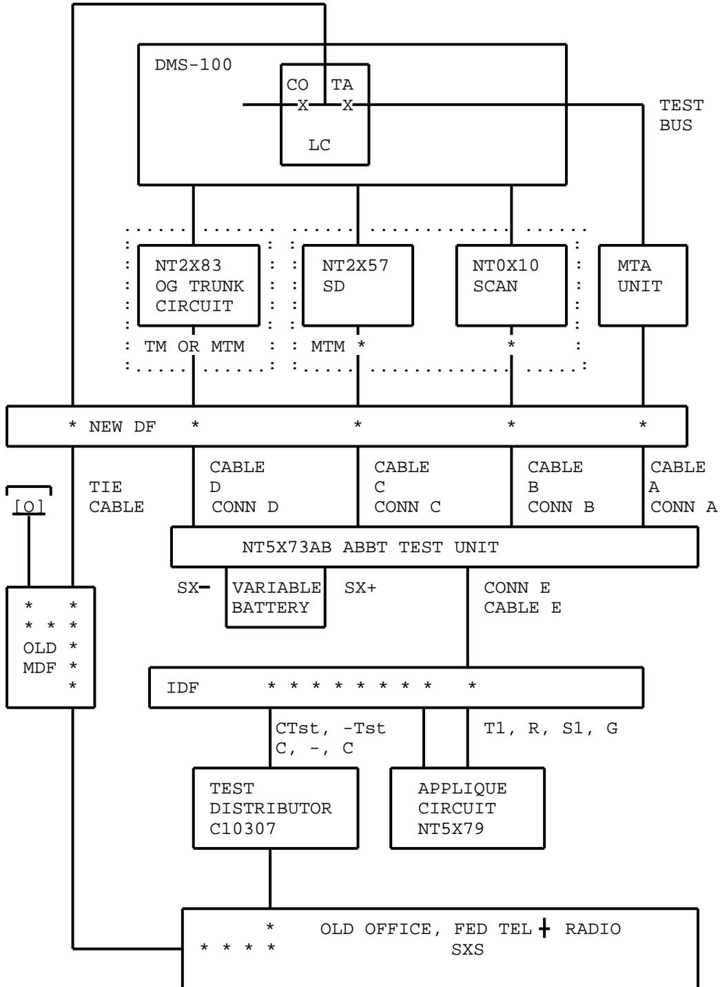
Fig. 17 - ABBT Connections for FED TEL + RADIO SXS Switches
