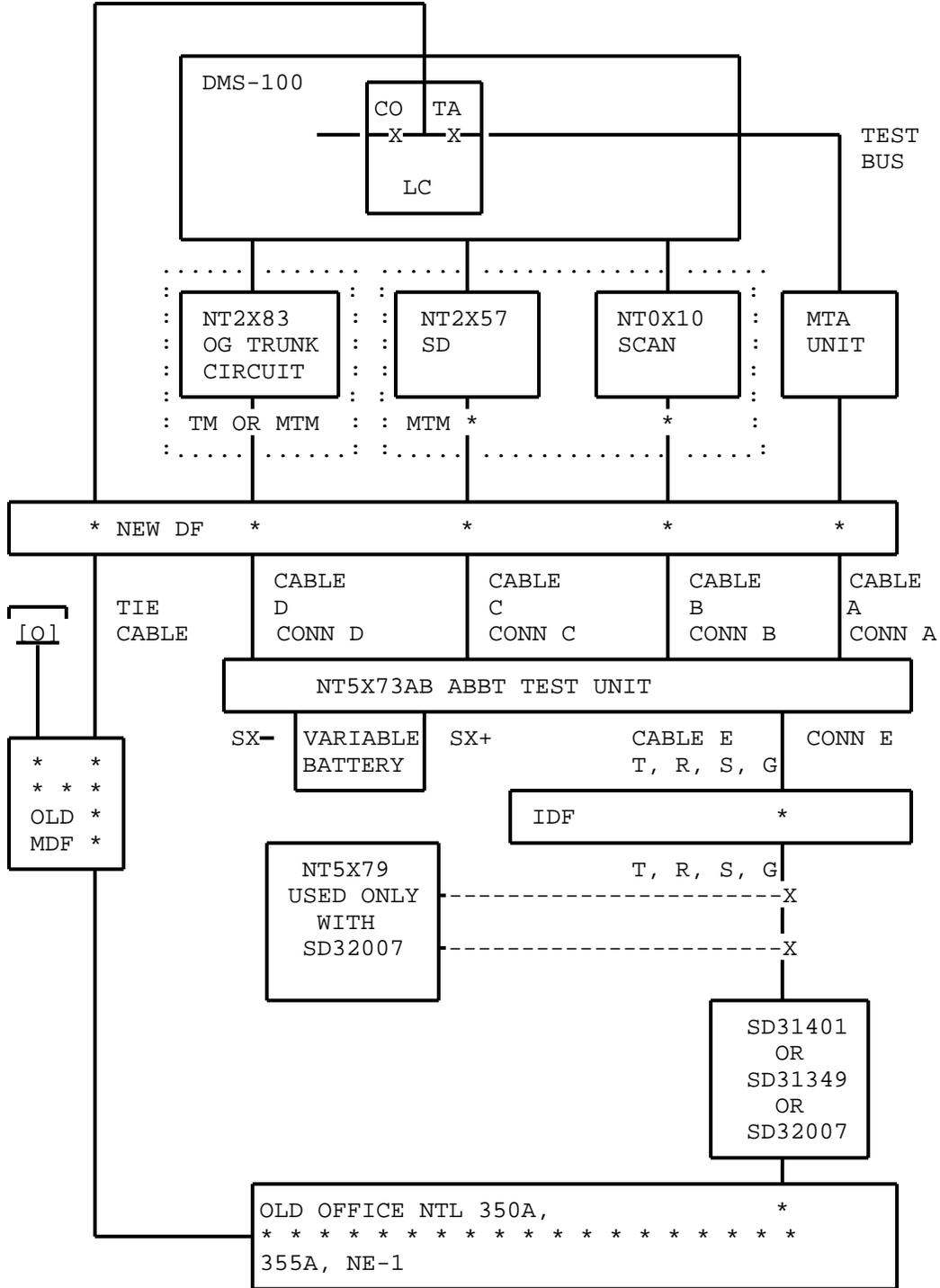
Fig. 30 - ABBT Connections for NTL 350A, 355A, NE-1
