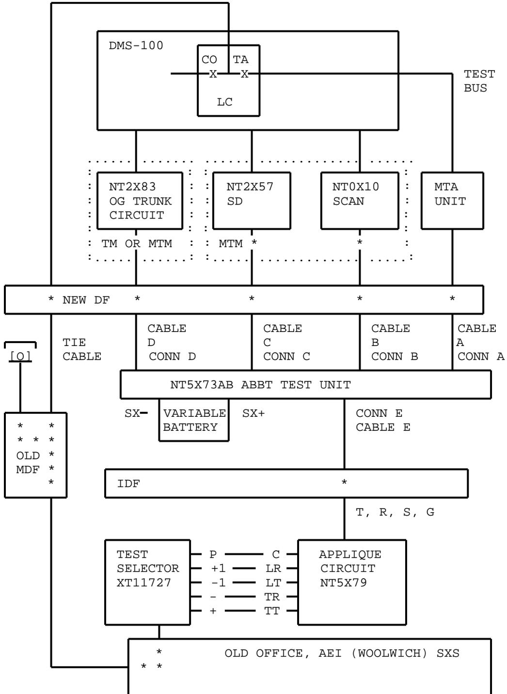
Fig. 8 - ABBT Connections for AEI (Woolwich) SXS Switches
