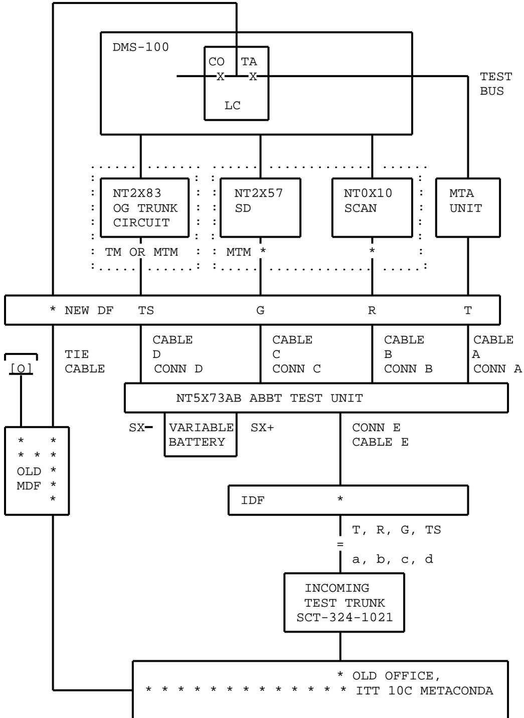
Fig. 20 - ABBT Connections for ITT 10C Metaconda Switches
