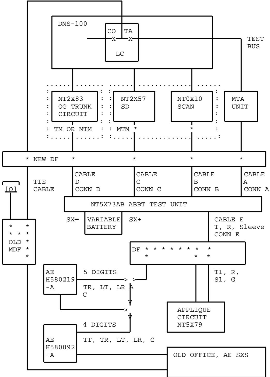
Fig. 11 - ABBT Connections For AE SXS Switches
