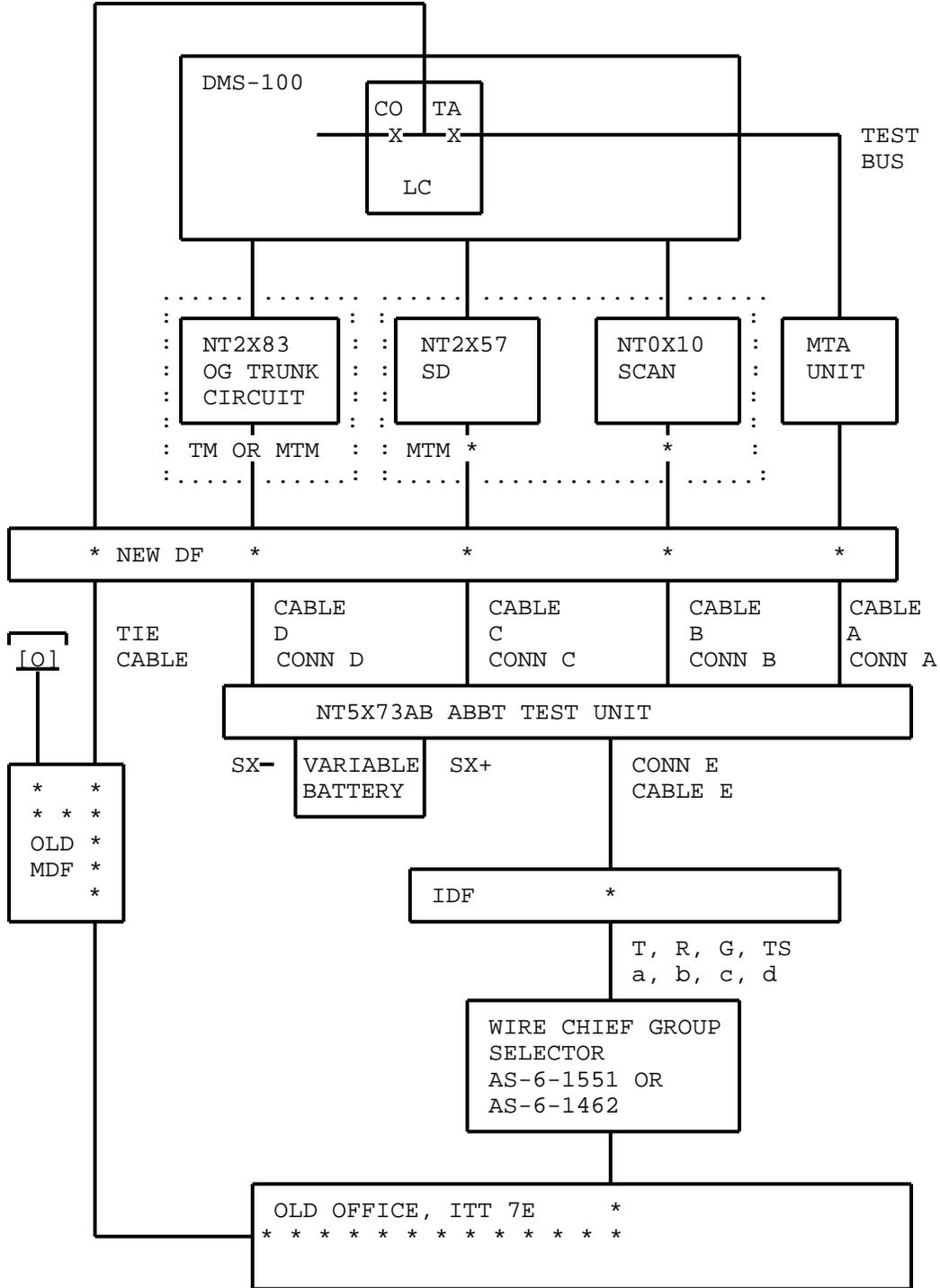
Fig. 21 - ABBT Connections for ITT 7E (Belgium) Switches
