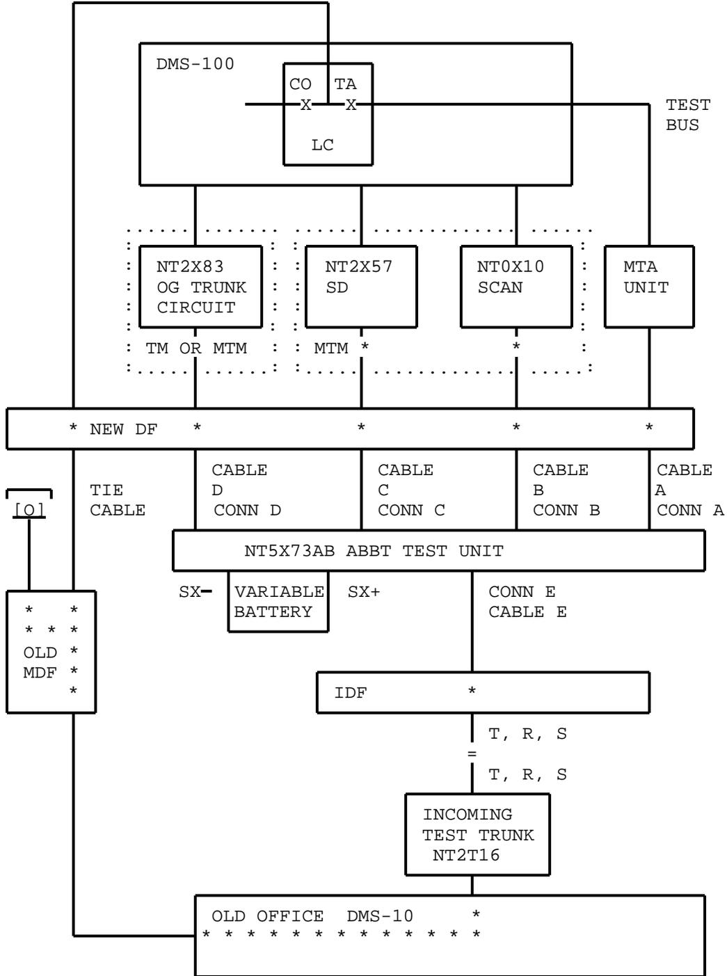
Fig. 25 - ABBT Connections for NTL DMS-10 Switches
