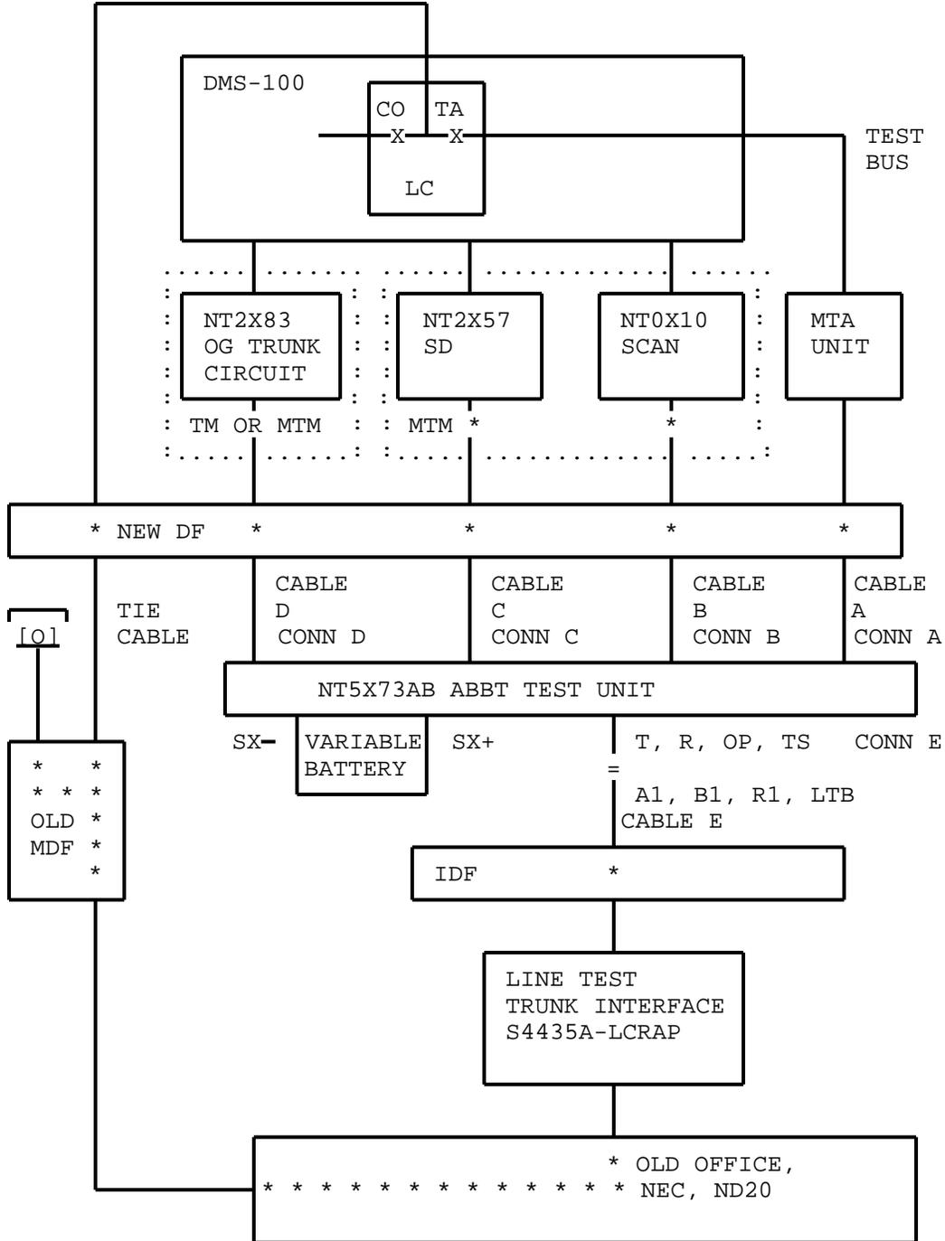
Fig. 22 - ABBT Connections for NEC ND20 Switches
