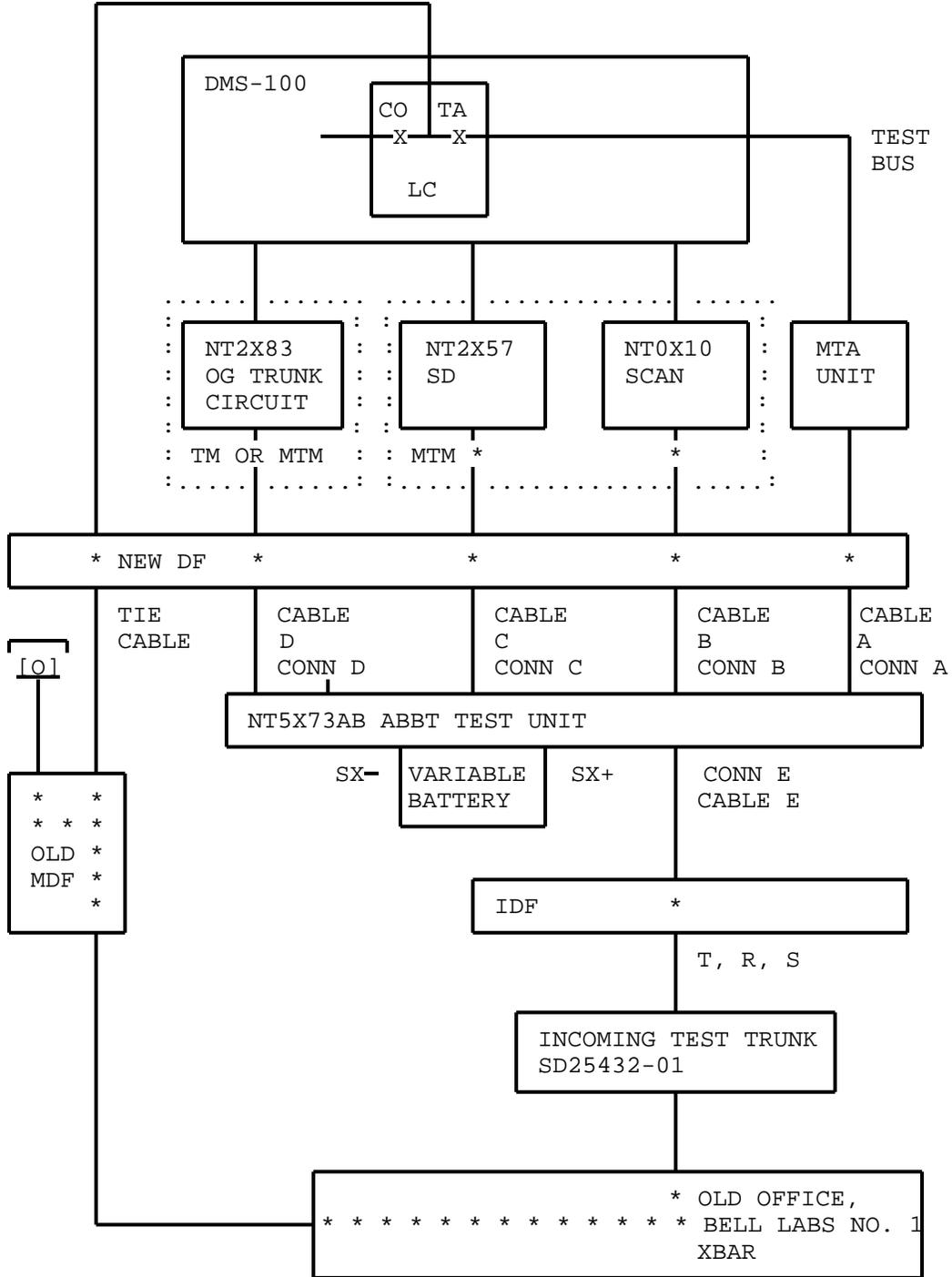
Fig. 14 - ABBT Connections for Bell Laboratories No.1 XBAR
