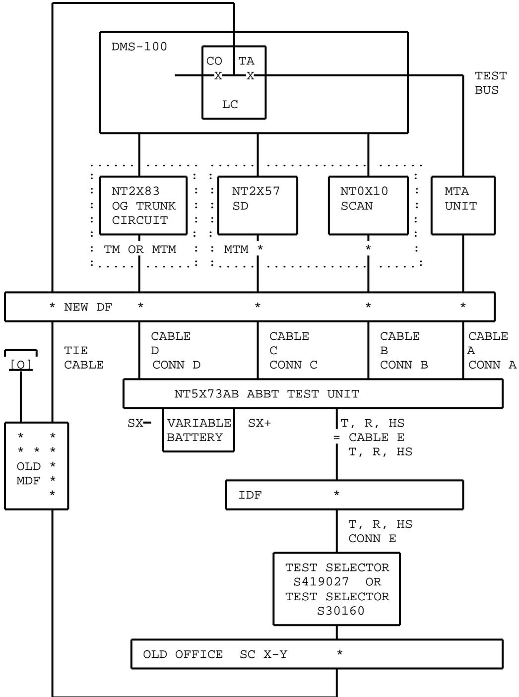
Fig. 31 - ABBT Connections for SC X-Y Switches
