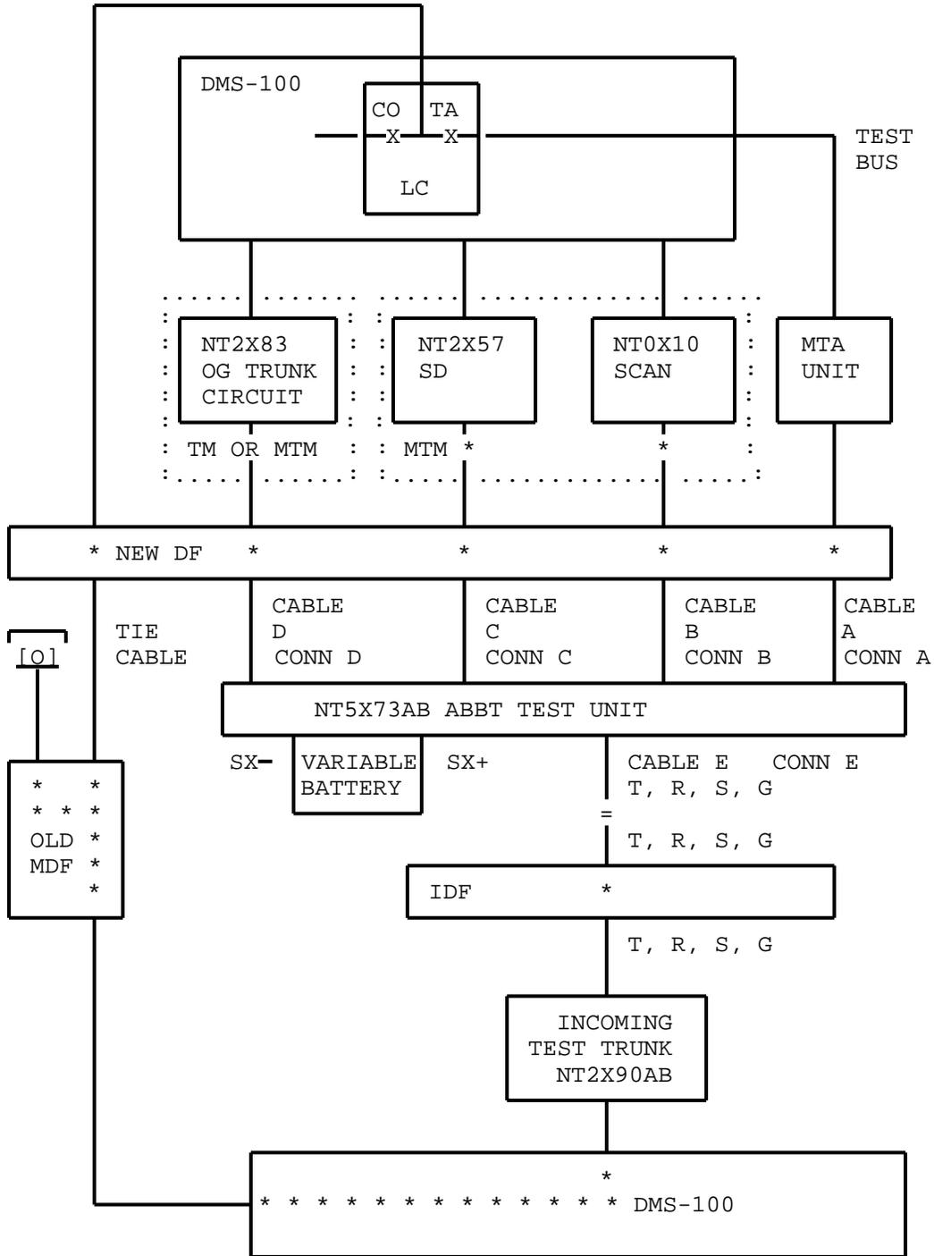
Fig. 26 - ABBT Connections for NTL DMS-100 Switches
