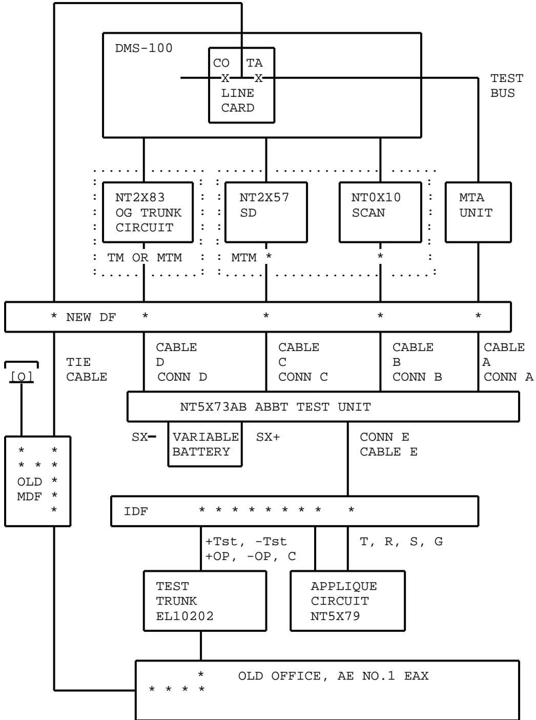
Fig. 13 - ABBT Connections for AE No.1 EAX Switches
