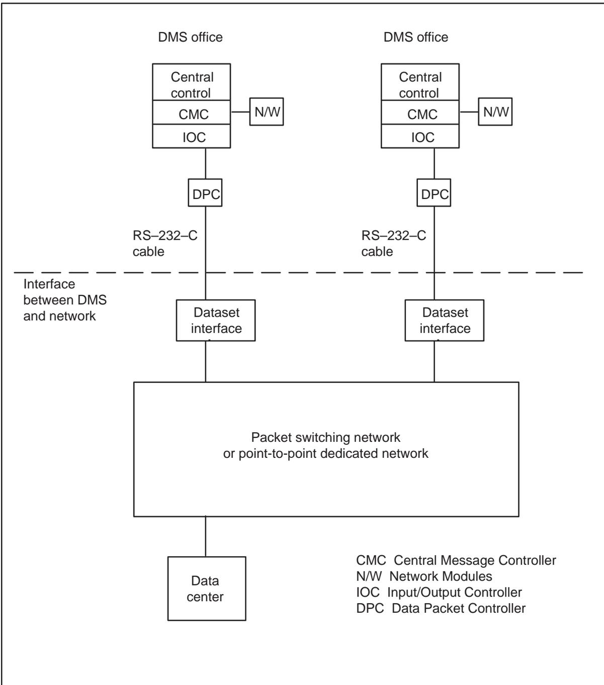
Each DPC (NT1X67BB or NT1X67DB) is on the input/output controller (IOC) shelf of the DMS central control (CC). The central message controller (CMC) of the CC interprets messages it receives from the DPC
