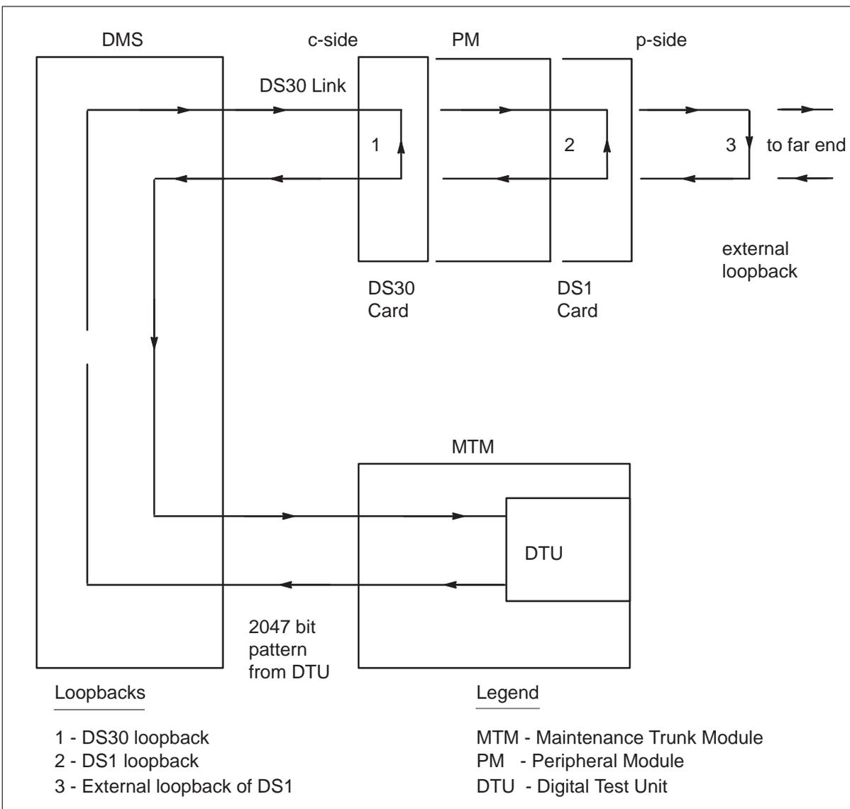
The DS30 loopback is at the c-side of the peripheral module (PM) and can be defined for a specific channel (trunk) without affecting other channels on the DS30 link. When a trunk is tested on a Remote Cluster Controller (RCC), the actual loopback is on the DS30 card on the LTC.
