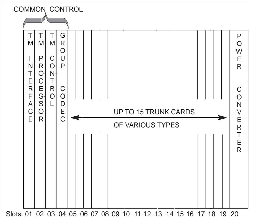
Shelves with AIM conform to present ISM and RMM shelf designs. Mount the AIM controller card (NTFX46AA) in any even-numbered slot (6 through 16) in MTM shelves. If you use card B (NTFX48AA), the card occupies the odd-numbered slot to the left side.
