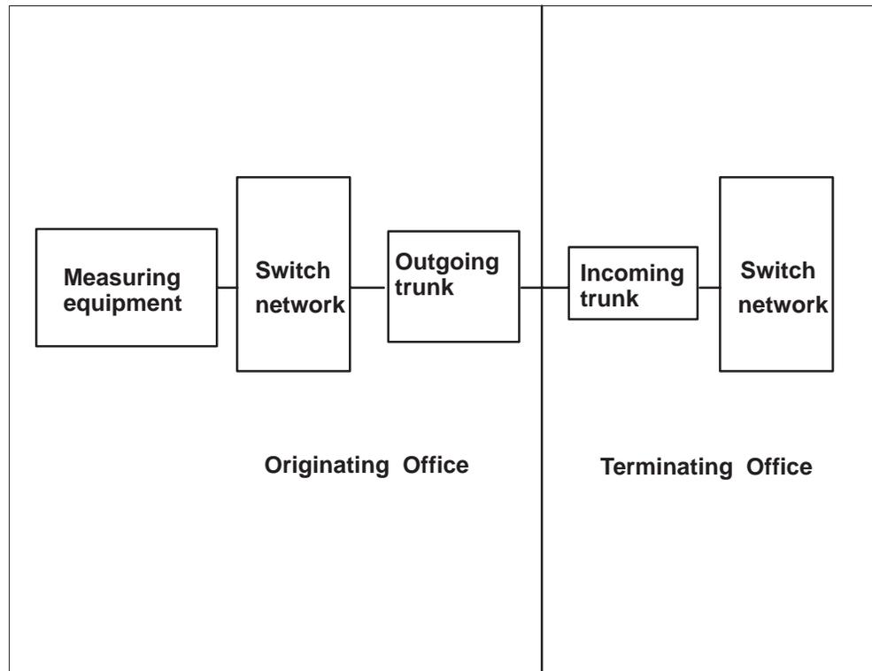
When a DMS-100 office terminates a synchronous test line test, the sequence is as follows:
