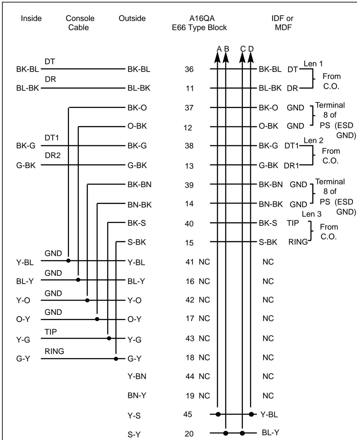
**Note: 1** There are no violet wires in an A16QA type cable; therefore, loops are not required.
