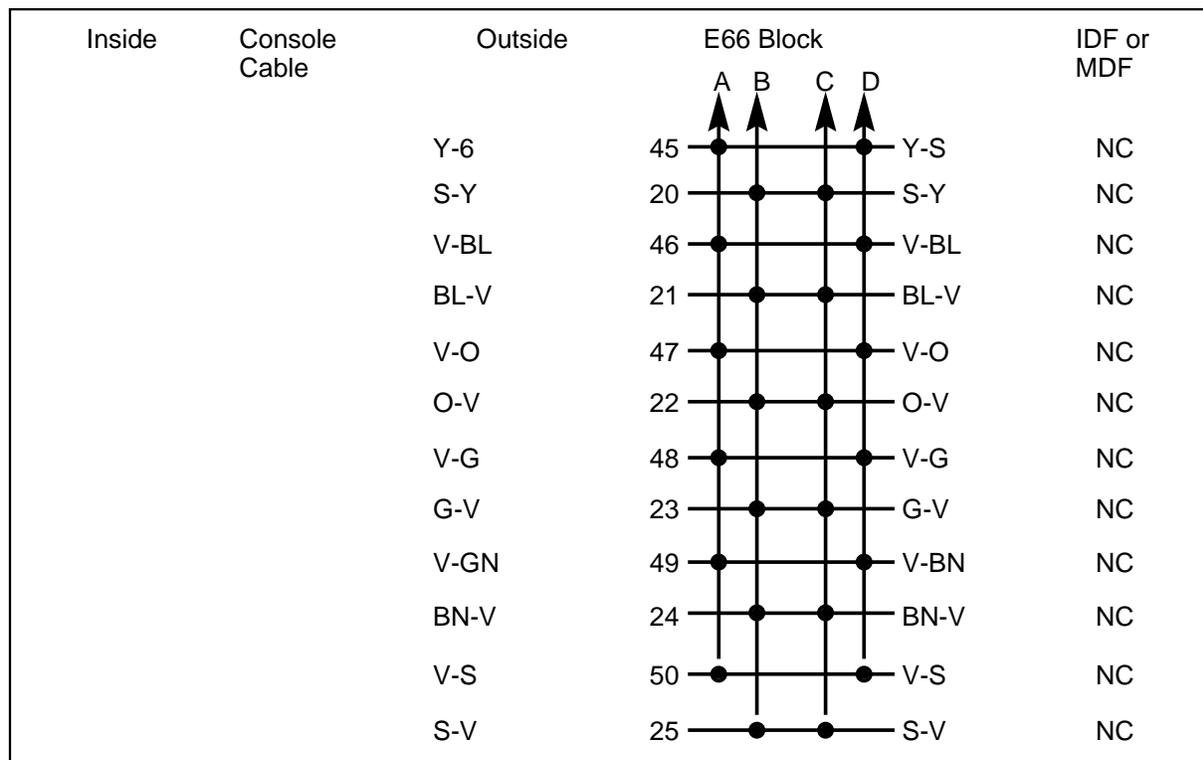
**Note:** Open-ended cable leads may pick up RFI or impulse noise. We strongly recommend, therefore, that all non-functional leads be looped to ground or -48V on both ends as shown. An E66 block or equivalent allows a convenient method of looping non-functional leads at the console; loop these leads at IDF or MDF as shown.
