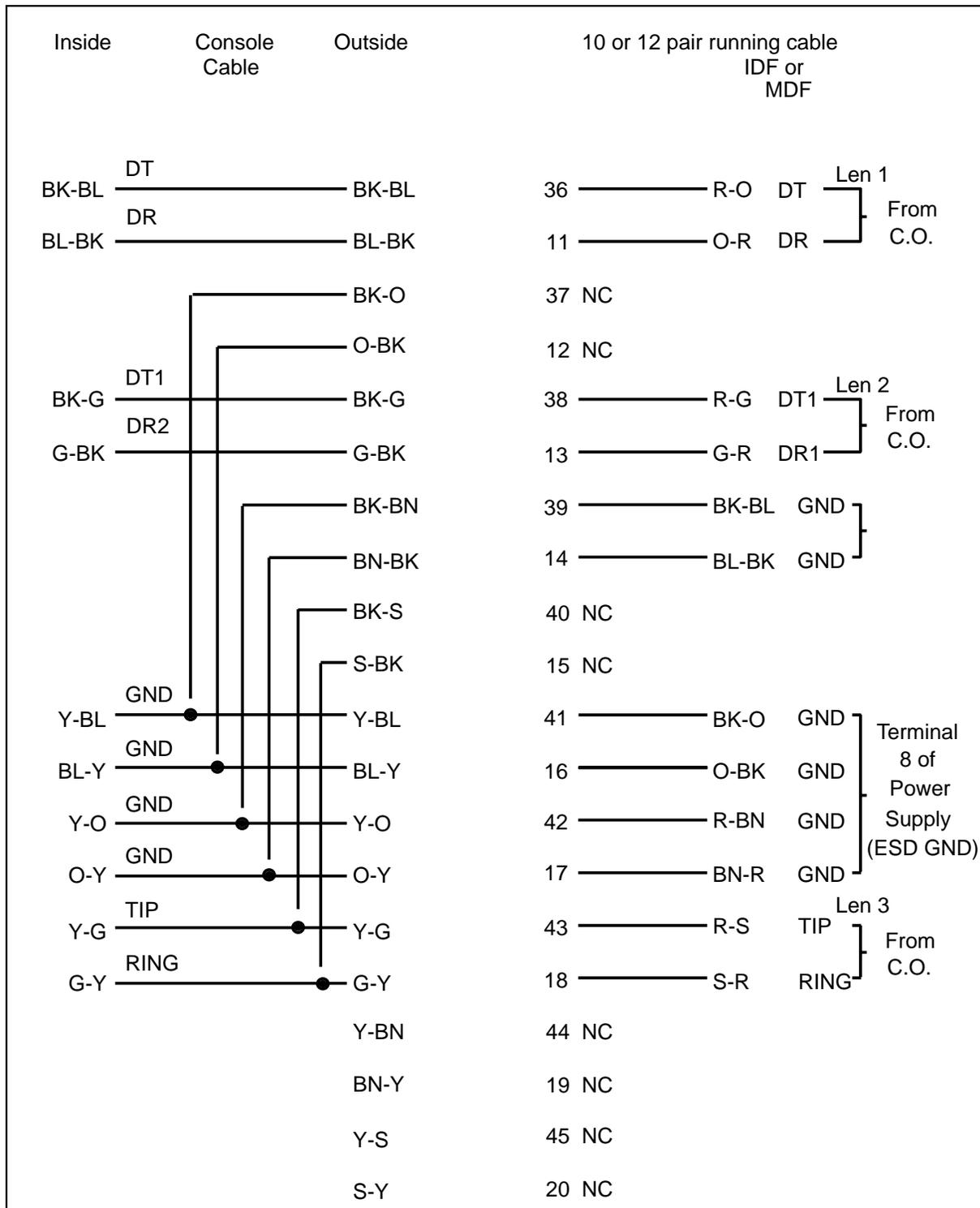
**Note: 1** Connectivity shown is for 12-pair cables. For 10-pair cabling, omit BK-BL pair and BK-O pairs. All others are as shown.
