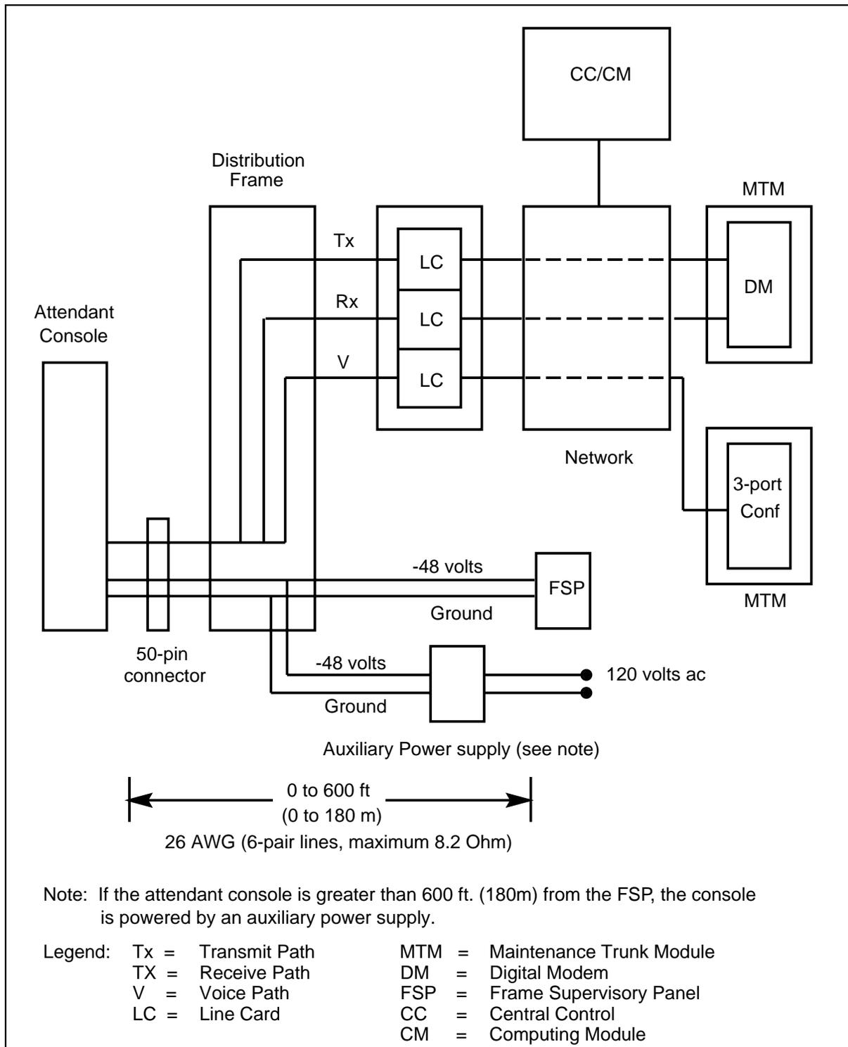
Each console requires a digital modem (Dmodem) circuit. Two circuit packs, NT3X02AA and NT3X03AA, used together, provide four Dmodem circuits. Provision only one Dmodem card per MTM.
