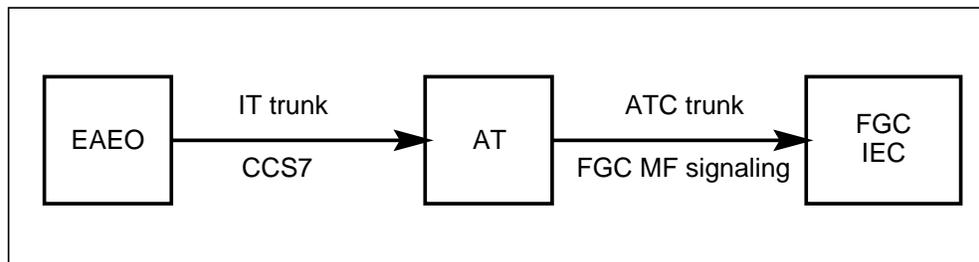
The translations datafill required to terminate an FGC call to an AT over a CCS7 IT trunk are the same as those required to terminate a similar call over an MF IT trunk.
