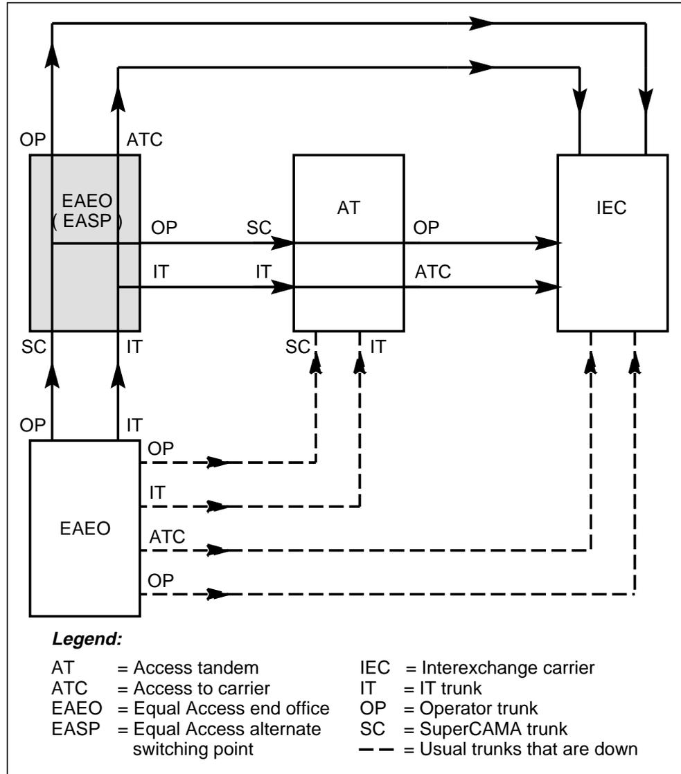
There are two types of FGC calls: operator and IT. An FGC IT call enters the EASP on an IT trunk. The call can leave the EASP in one of the two following ways:
