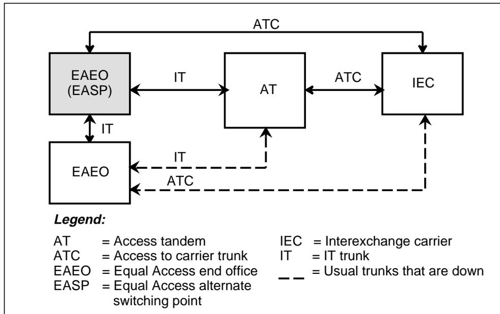
If the direct IT trunks between the EAEO and the AT are down, an FGD call can still be routed through the EASP. In this case, the FGD call leaves the EAEO on an IT trunk and also enters the EASP on an IT trunk. The trunk connection between the EASP and the AT is also IT to IT. When the FGD call leaves the AT for the IEC, the call leaves on an ATC trunk.
