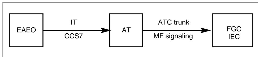
Figure 4-11 shows interworking for FGC inband signaling to CCS7. This configuration is required for call originations that terminate to an FGD IEC via the AT. The facilities between the EAEO and the AT are IT or SC trunk groups supporting traditional inband signaling. The facilities between the AT and the FGD carrier are ATC trunk groups supporting CCS7.
