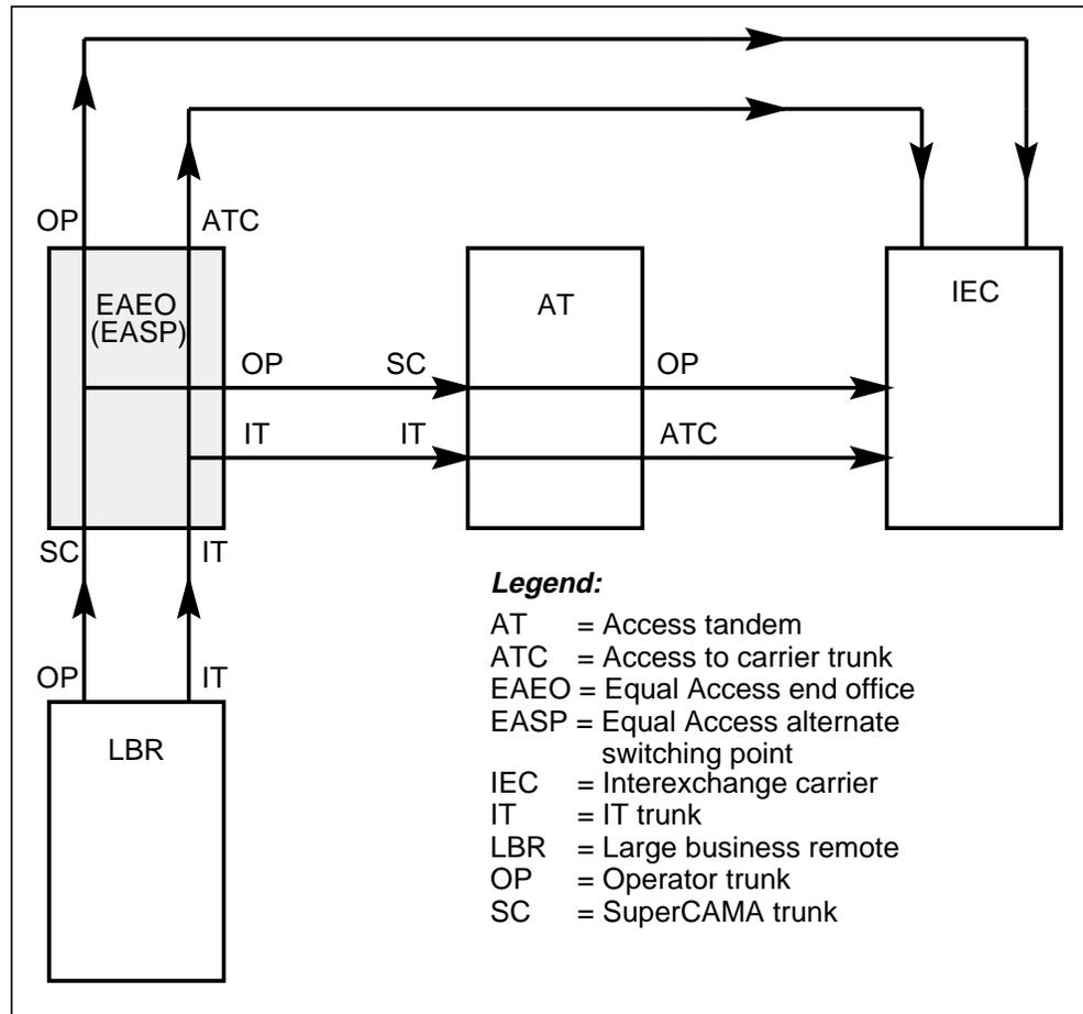
All FGC operator and IT calls originating in an LBR are passed through an EASP before going through an AT or directly to an IEC. An FGC IT call enters the EASP on an IT trunk. The call can leave the EASP in one of the two following ways:
