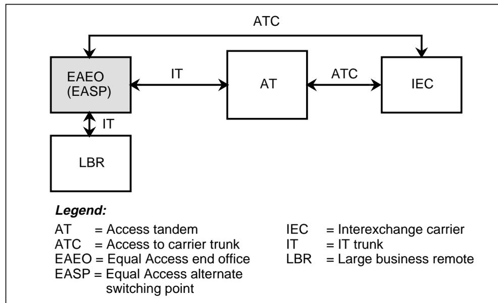
FGD calls that originate in an LBR pass through an EASP before going through an AT or directly to an IEC.
