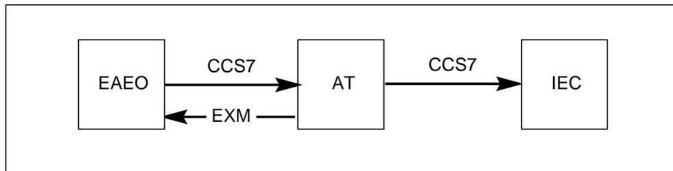
For the other call configurations implemented by this feature, the trunk group number in the originating AMA records is determined in the existing manner; the common language location identifier (CLLI) of the outgoing trunk from the EAEO is used as an index in table CLLI to get the trunk group number.
