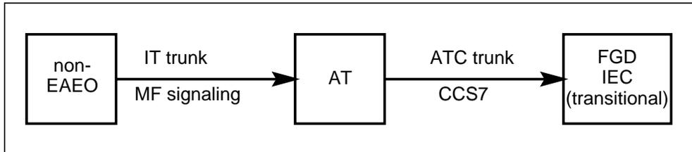
Figure 4-9 shows interworking for EAP MF-to-CCS7. This configuration is required for 950-WXXX call originations from an EAEO that terminate to an FGD IEC via the AT. The facilities between the EAEO and the AT are IT or SC trunk groups supporting EAP inband signaling. The facilities between the AT and the FGD IEC are ATC trunk groups supporting CCS7. Enhancements are provided by this feature in the AT to support the EAP MF-to-CCS7 interworking.
