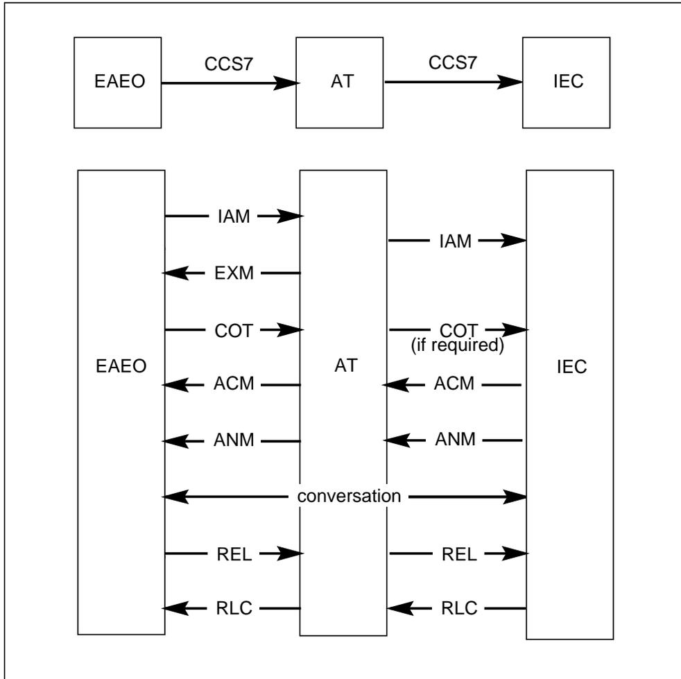
The IAM received at the AT must include the optional transit network selection (TNS) parameter. The parameter contains four octets of data, three of which represent the binary-coded-decimal (BCD) equivalent of the Equal Access CAC. The fourth octet indicates the Equal Access circuit code, which is analogous to the 0ZZ or 1N/N'X digits outputted on MF IECs. The TNS parameter (with the country code on international calls) indicates the outgoing IEC to be selected by the AT.
