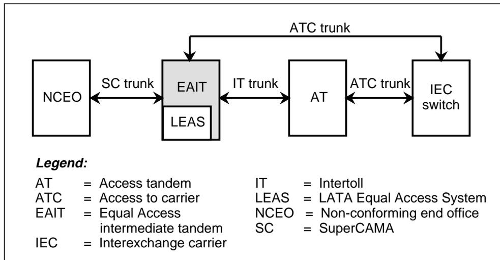
With this feature package, non-OA calls incoming to the EAIT over SC trunks that are recognized as LEAS calls will be tandemmed to an AT over IT trunks using FGD signaling. If the carrier has a point of presence at the EAIT, the calls can be sent directly to the carrier over ATC trunks. Operator traffic will be routed as done with LEAS.
