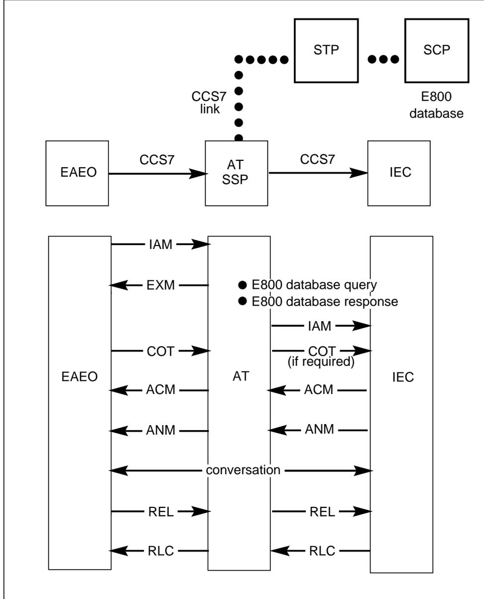
An EXM is always sent to the EAEO when the the AT launches the query to the E800 database. When the database response from the E800 SCP is received at the AT, the call is completed based on the decoded routing information. The CCS7 messages returned to the EAEO depend on the type of facility on which the call is terminating. In this case the terminating facility is a CCS7 IEC or IEC.
