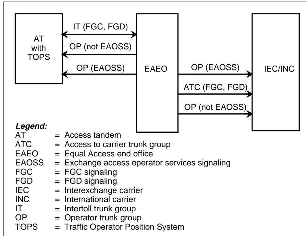
Any or all of the following types of traffic can be combined on an operator trunk group and signaled with EAOSS:
