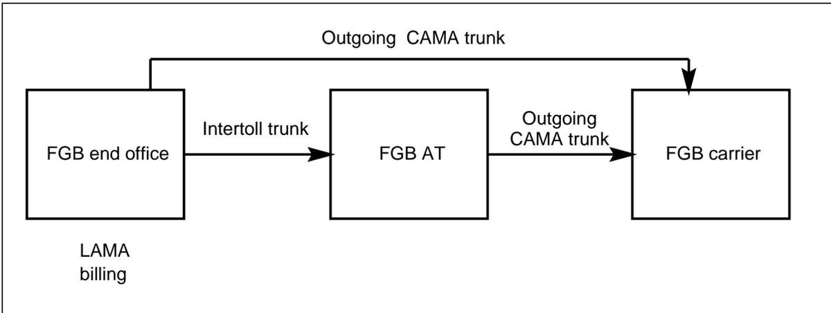
The FGB selector must be used in the end office for LAMA billing to work properly. The FGB selector is also recommended in the following cases:
