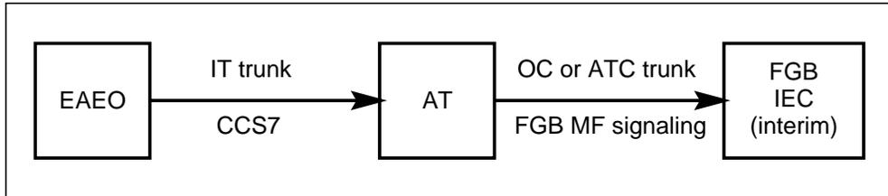
Figure 4-8 shows traditional MF-to-CCS7 interworking. This configuration is required for 950-WXXX call originations from a non-EAEO that terminate to an FGD IEC via the AT. The facilities between the non-EAEO and the AT are IT trunk groups supporting traditional inband signaling. The facilities between the the AT and the FGD IEC are ATC trunk groups supporting CCS7. Enhancements are provided by this feature in the AT to support the traditional inband signaling-to-CCS7 interworking.
