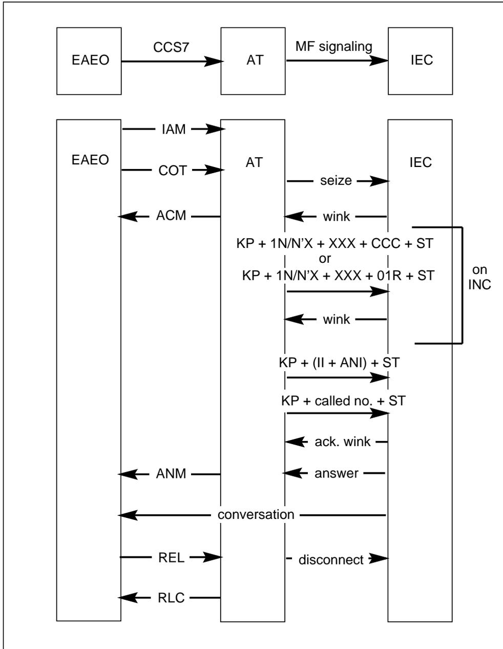
The AT seizes the outgoing circuit and waits for a wink. If the IAM contains an indication that a continuity check is performed on the incoming circuit, the AT does not wait until the continuity message (COT) is received with a “continuity check successful” indication before seizing the IEC.
