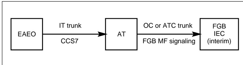
The translations datafill required to terminate a 950-XXXX call to an AT over a CCS7 IT trunk are the same as those required to terminate a similar call over an MF IT trunk.
