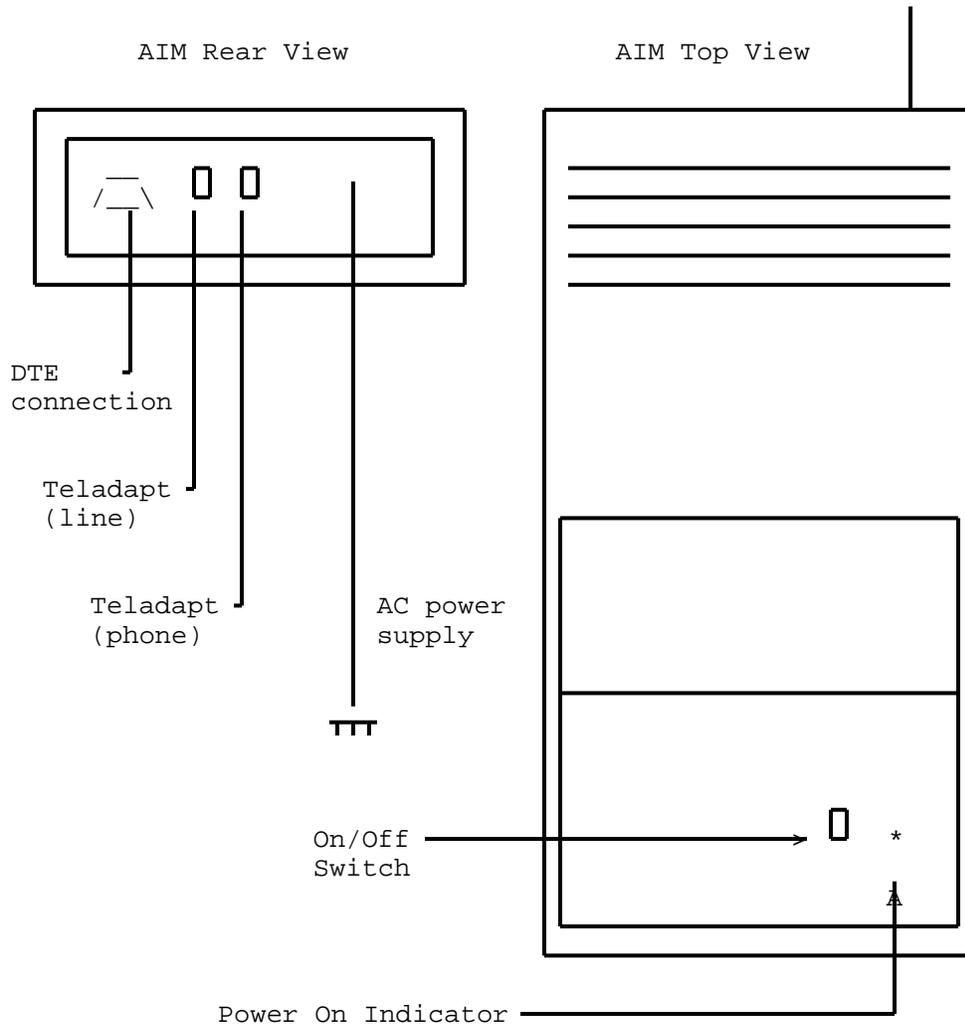
Fig. 1 - QMT9A Asynchronous Interface Module - Rear and Top View
