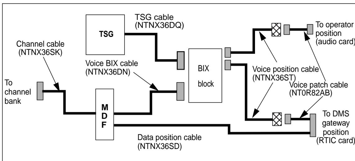
Figure 20. Voice and data cables from position to channel bank (Ethernet)
