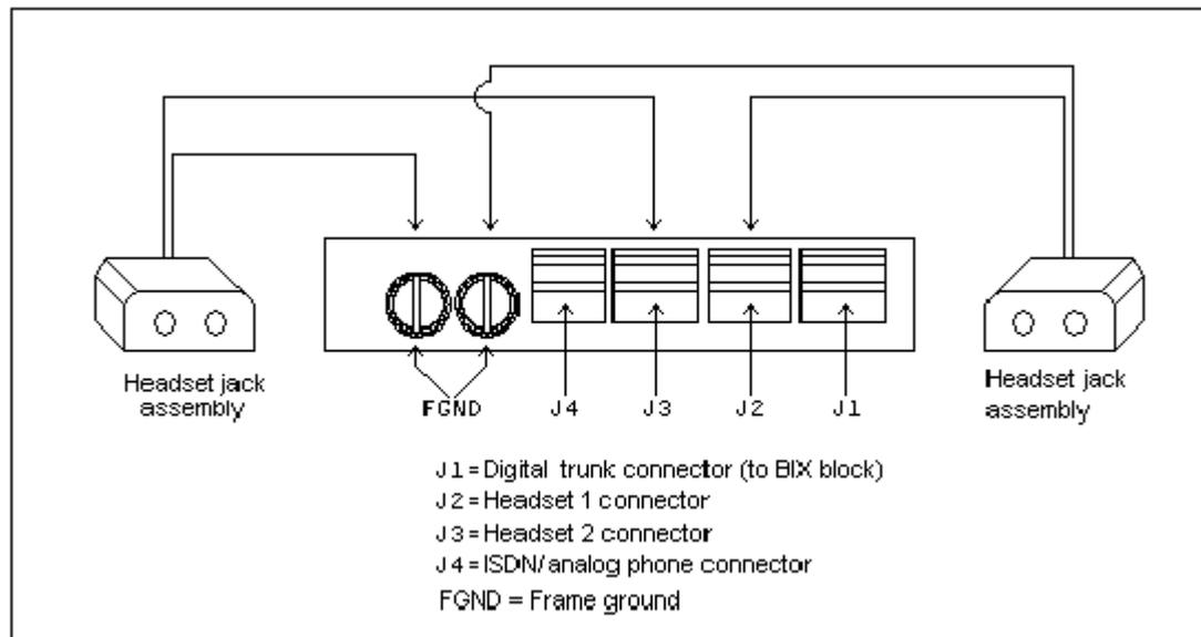
**Figure 12. Headset cable connections to PCI audio card - NTNX52CC**
