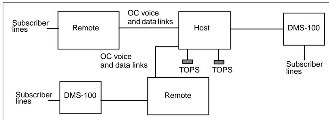
**Figure 23. OC system architecture**
