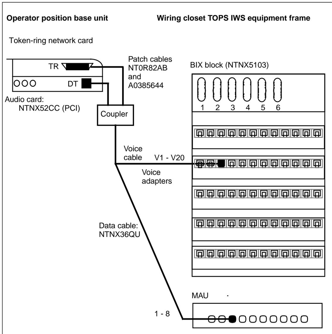
Figure 18. Audio card and token-ring connections to frame
