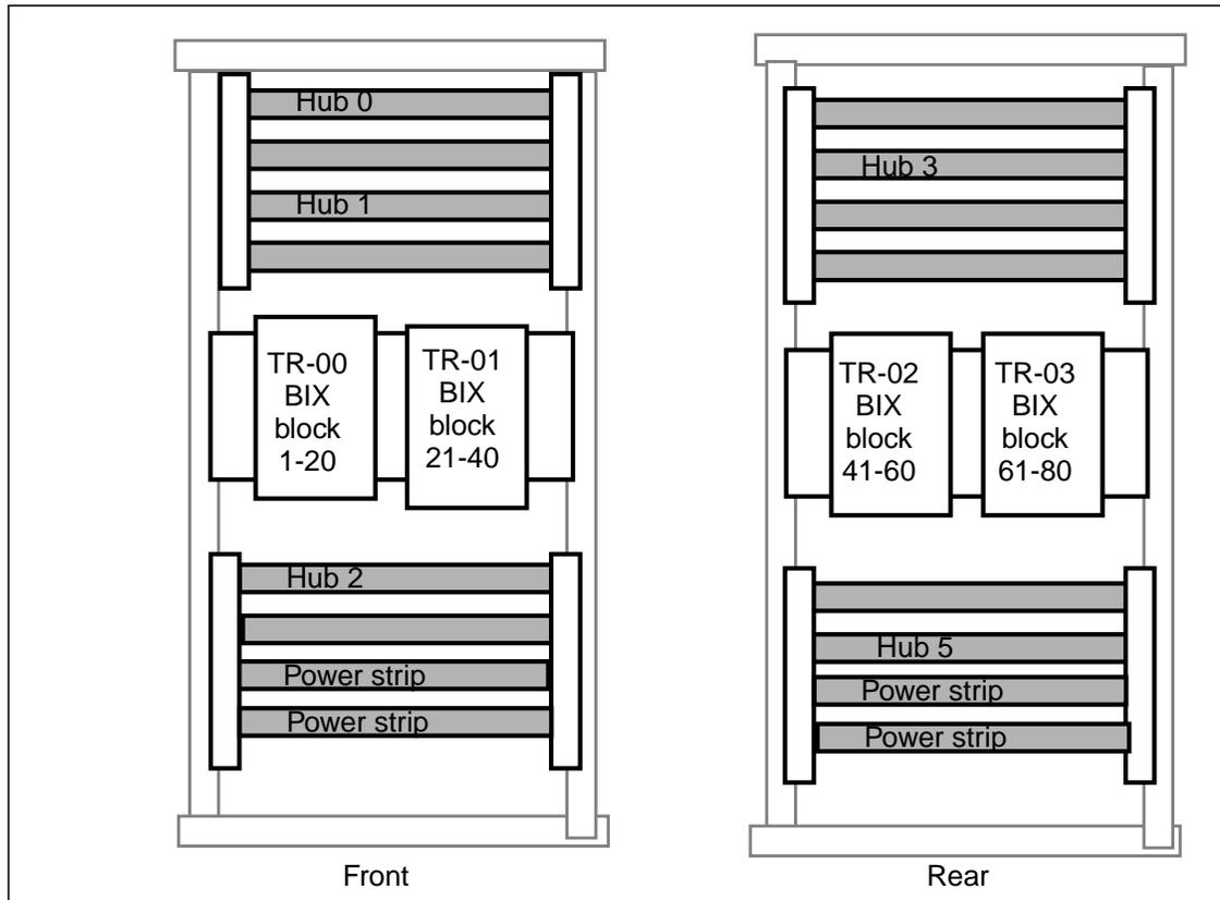
Figure 14. Wiring closet equipment with Ethernet hubs and BIX blocks
