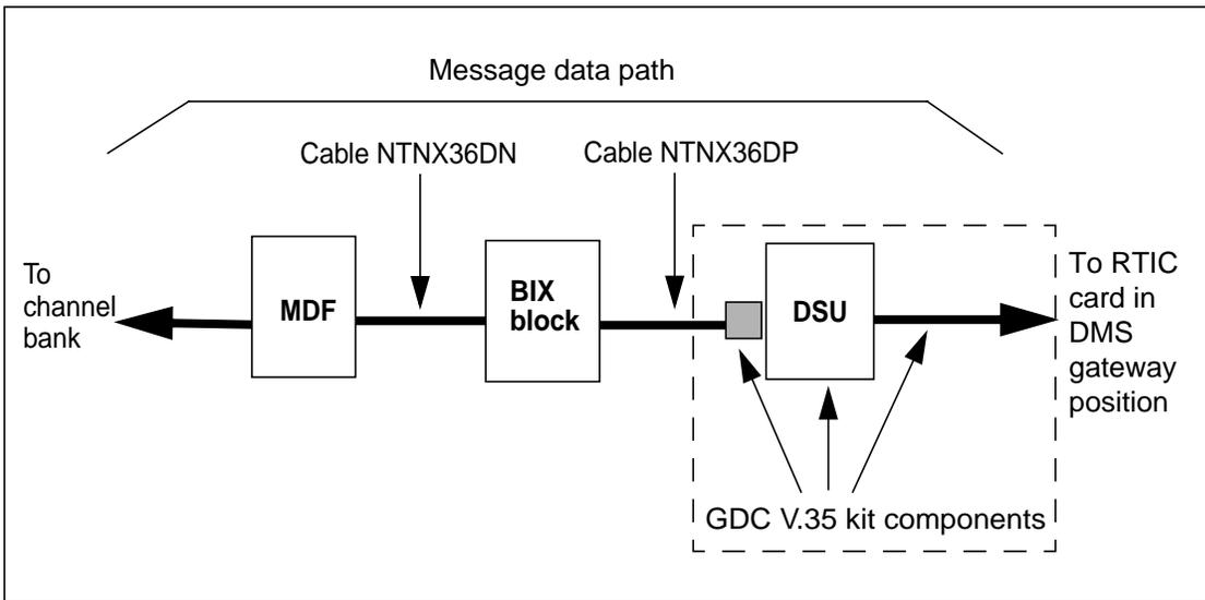
Figure 22. V.35 hardware for message data path
