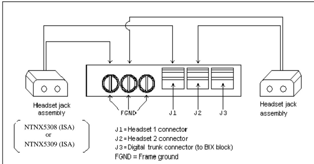
Figure 13. Headset cable connections to the ISA audio card - NTNX52BC
