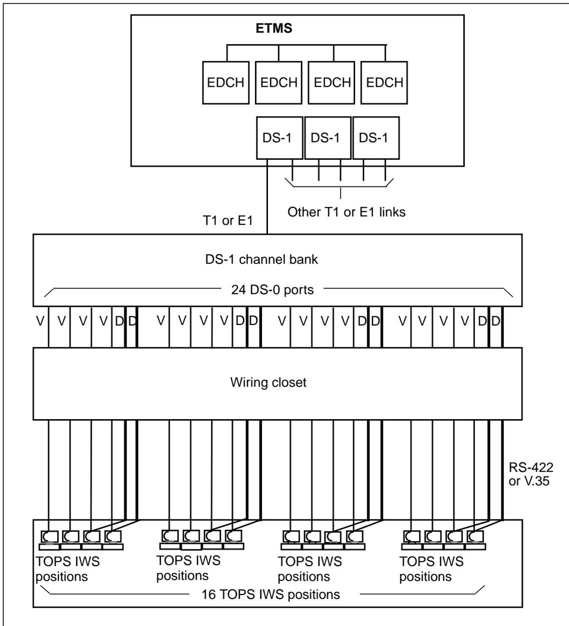
**Figure 4. ETMS and TOPS IWS interface**
