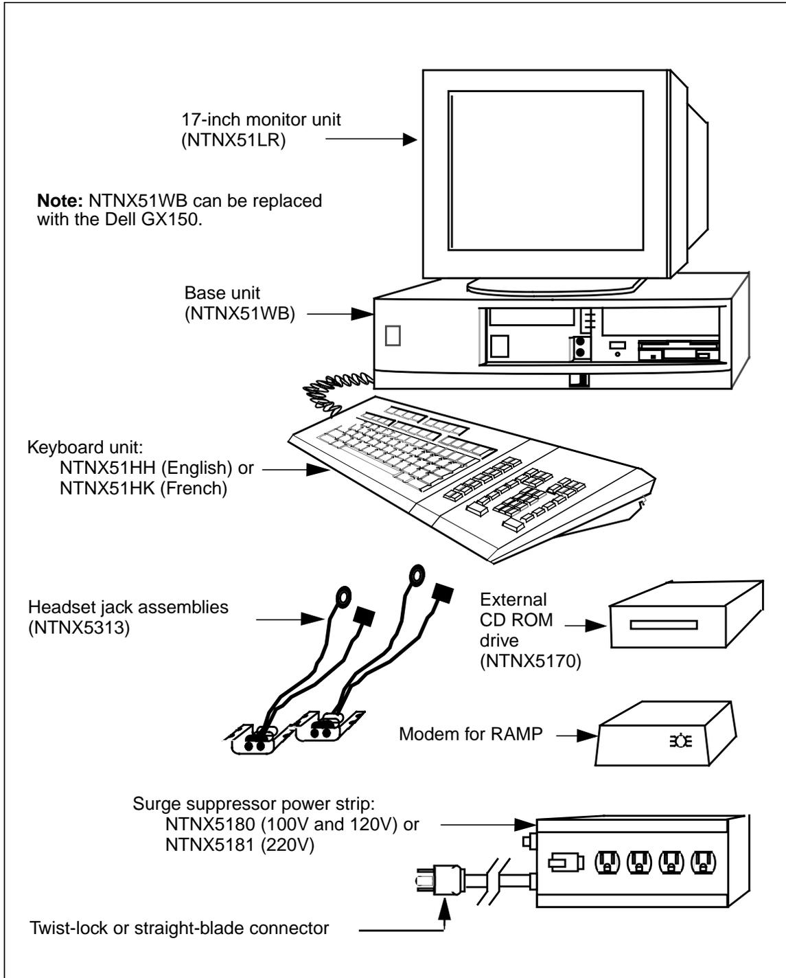
Figure 6. Operator position equipment
