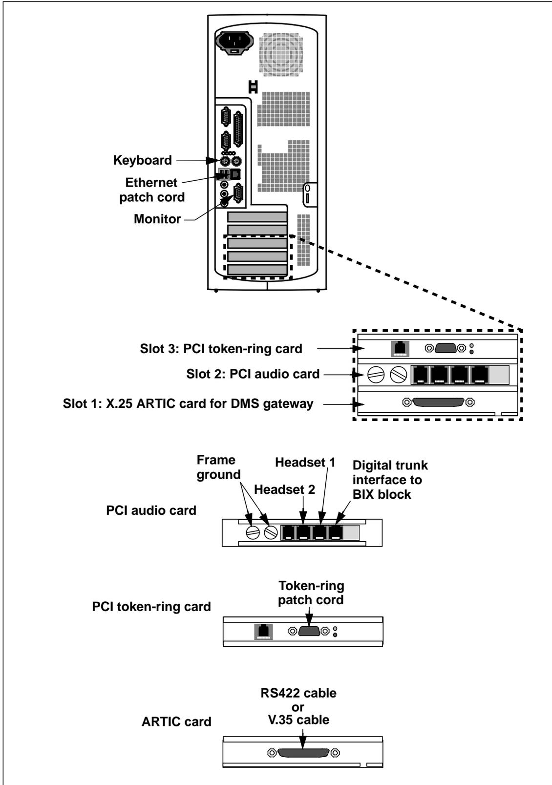
Figure 9. Base unit circuit cards for Dell GX150
