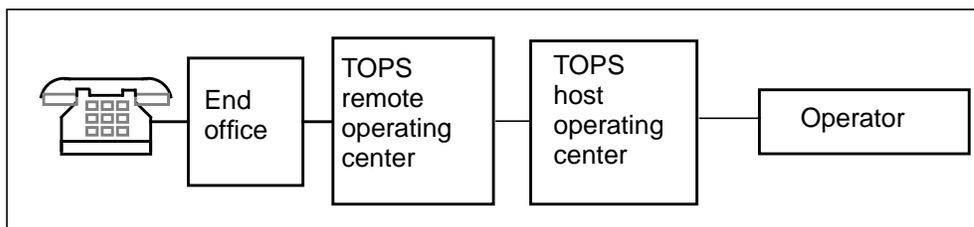
**Figure 3. Host and remote configuration**
