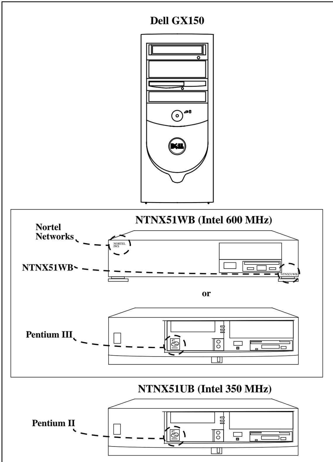
FIGURE 5. Examples of IWS Base Units for IWS Release 17.0
