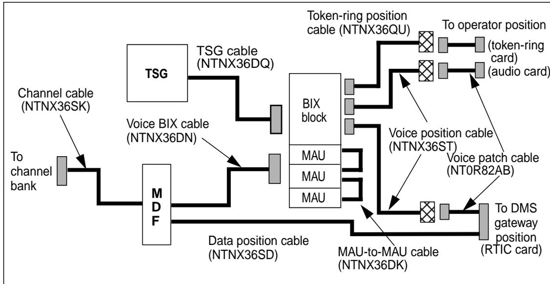
Figure 21. Voice and data cables from position to channel bank (token ring)
