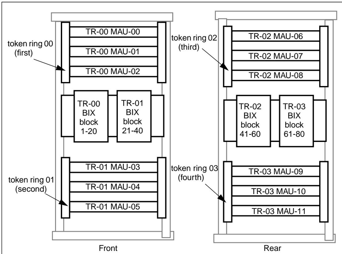
Figure 16. Wiring closet equipment with BIX block
