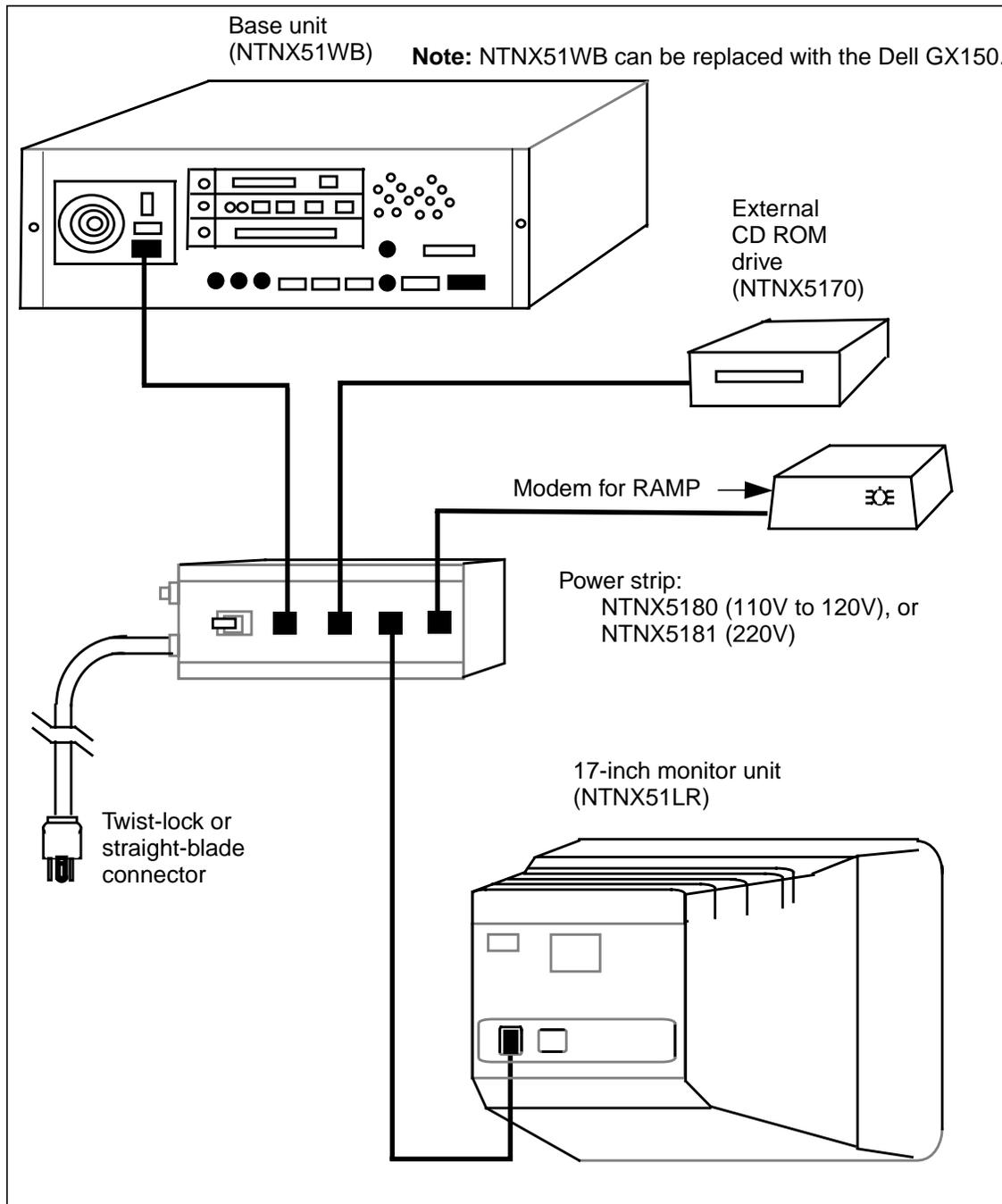
Figure 11. Operator position power
