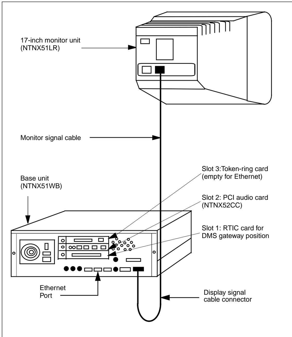
Figure 7. Monitor cable connection to base unit for NTNX51WB
