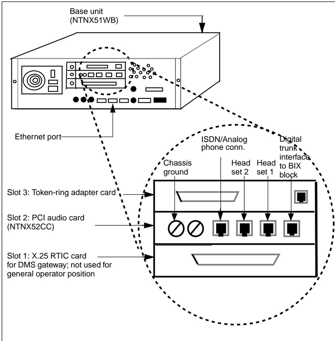
Figure 10. Base unit circuit cards for NTNX51WB
