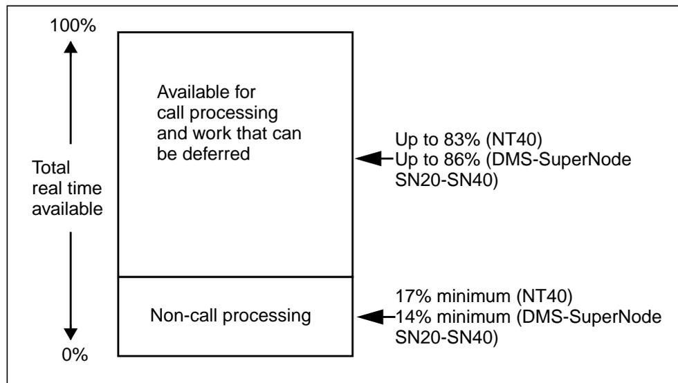
**Figure 31. CPU real-time availability for call processing**
