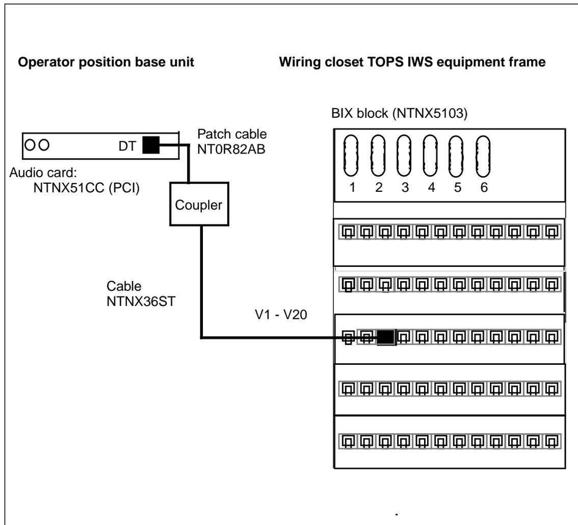
Figure 15. Audio card connections to frame
