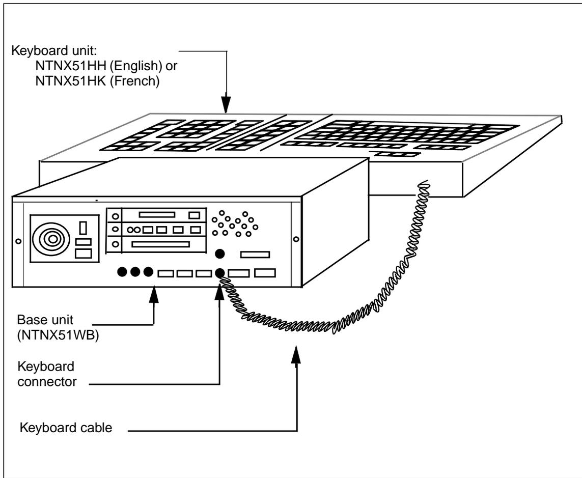
**Figure 8. Keyboard cable connection to base unit for NTN51WB**
