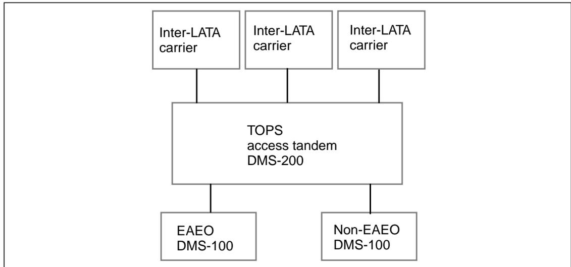
**Figure 24. DMS-based EA configuration**
