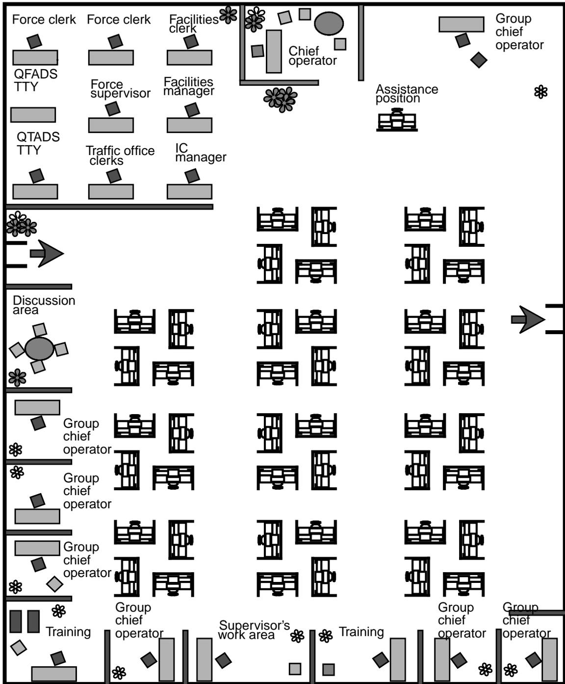
Figure 30. Example of a TOPS IWS multitraffic office
