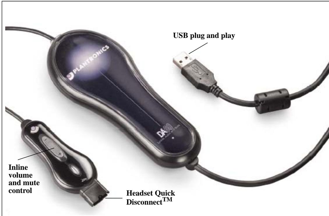
**FIGURE 2. Plantronics DA60 USB-to-headset adapter**
