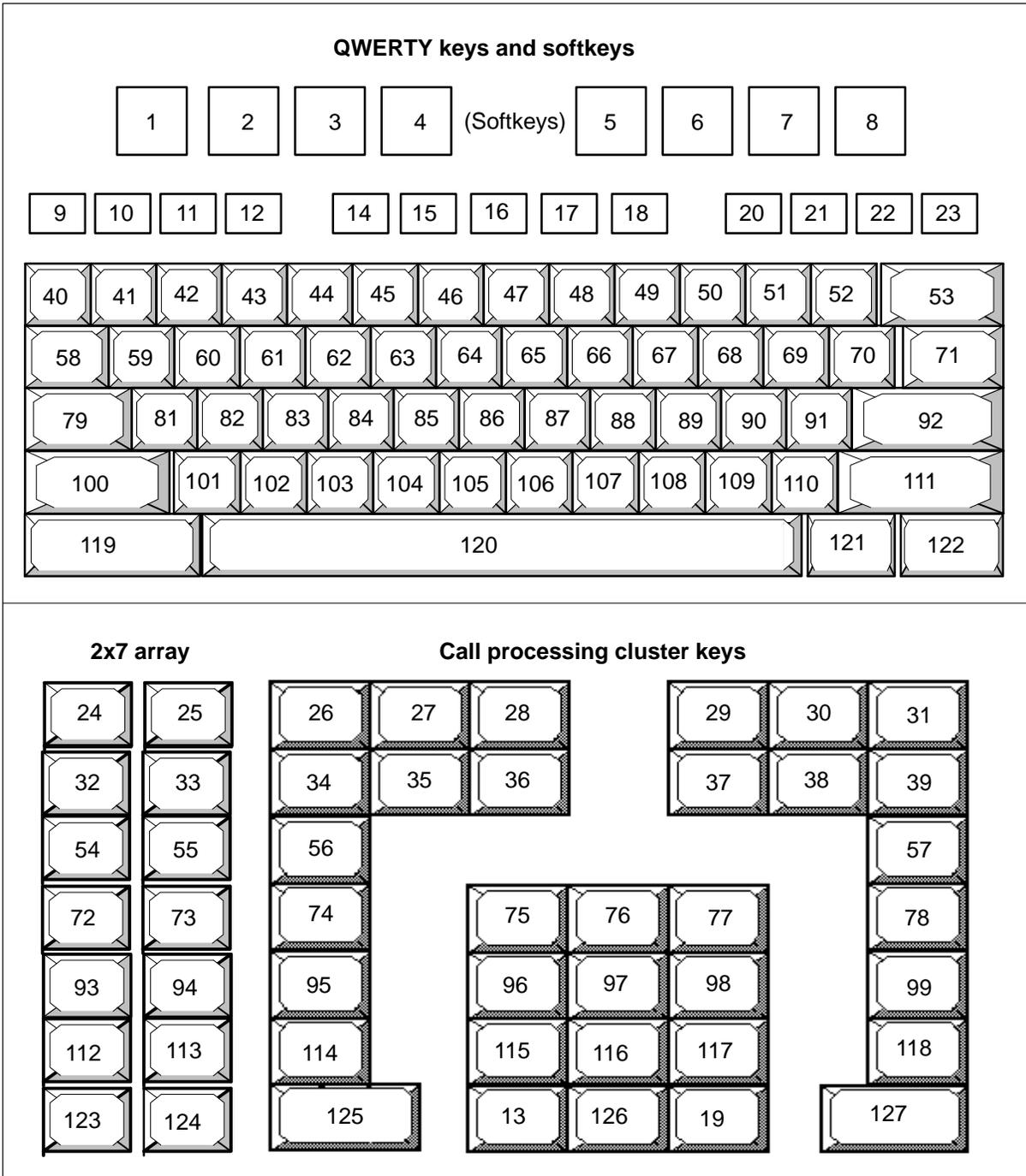
The first of eight menus for defining the keyboard (eight screens of default settings for CCI DA and IBM DA) is displayed by selecting choice 4 on the Define position settings menu. The three columns associated with each key in the Define keyboard menus identify the function of the key alone as well as in combination with the SHIFT key or ALT key.
