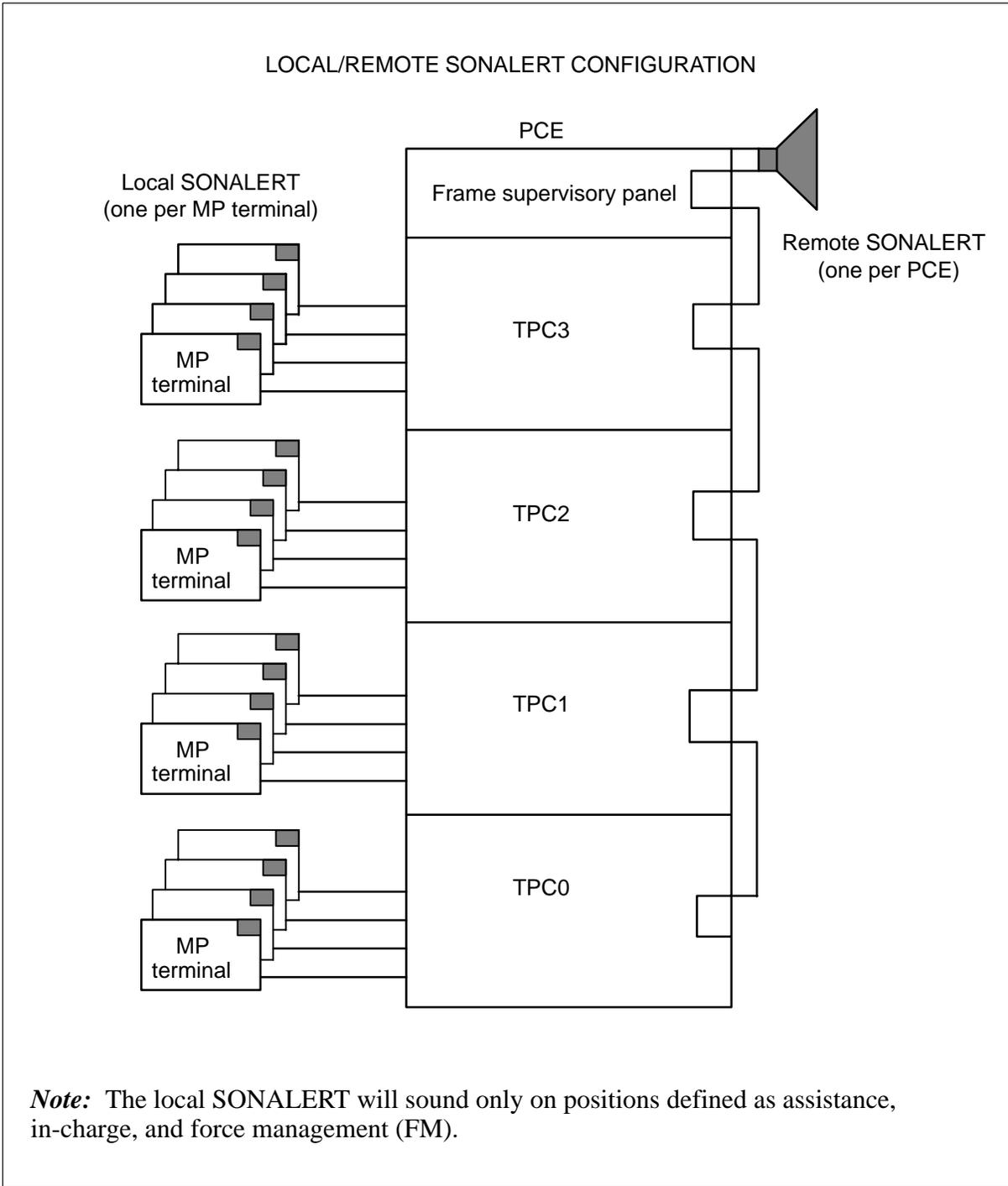
The capability to perform maintenance on the local and the remote SONALERT is provided through the SONALERT menu screen. Select choice 5 (integrated) or 8 (standalone) from the TAMI main menu to display the SONALART menu.
