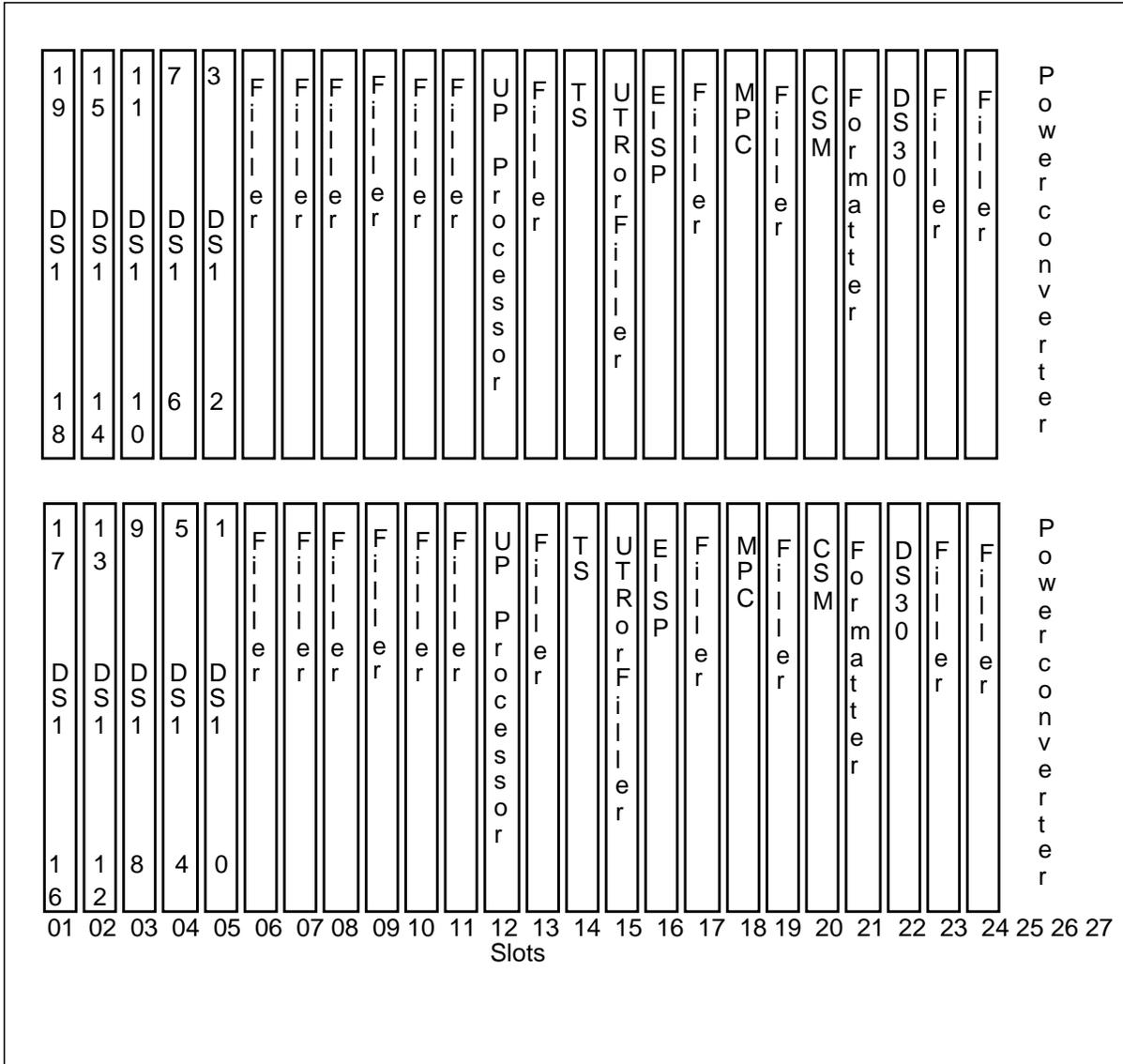
The following table shows the XMS-based peripheral module (XPM) circuit card list.
