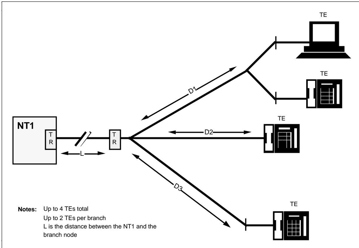
3. Polarity integrity should generally be maintained on all S/T-bus wiring, including all wiring, cross-connects, and teladapt cables (non-reversal) between the NT1 and all its associated TEs. Although not strictly required for point-to-point applications, it is recommended that the same practice be followed.
