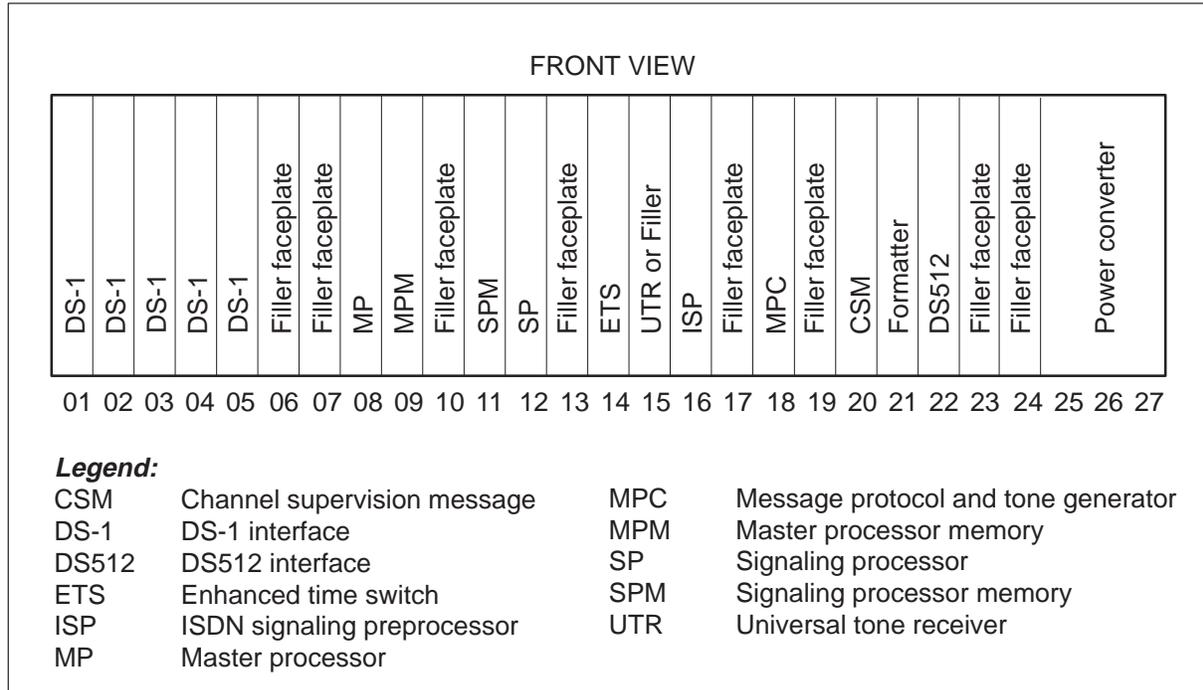
Figure 2-7 DTC7 shelf layout for DWS in an XPM configuration
