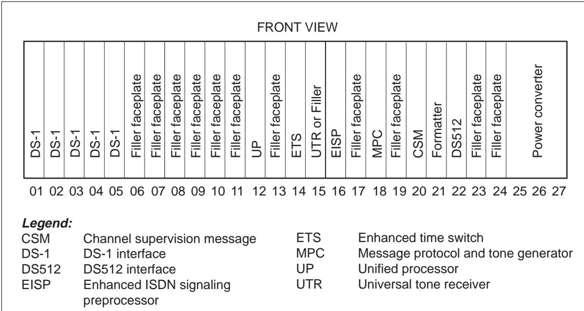
Figure 2-5 DTC7 shelf layout for DWS in an XPM PLUS configuration
