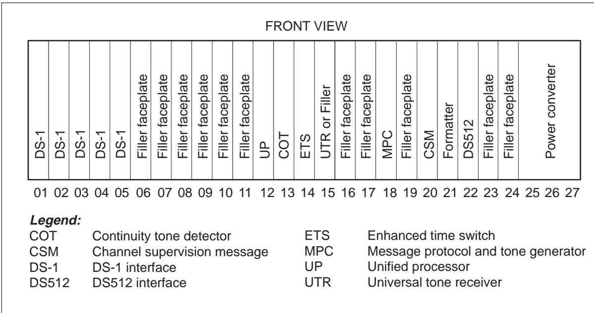
Figure 2-6 DTCI shelf layout for DWS in an XPM configuration
