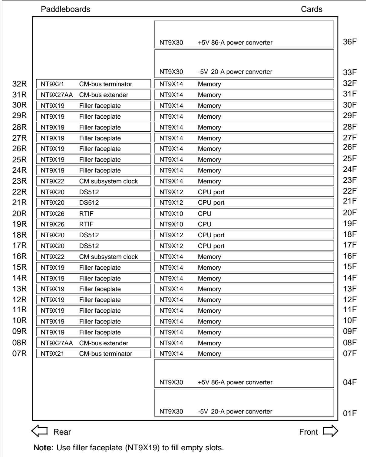
Figure 1-10 Example of a Series 50 to 70 SuperNode SE CM/SLM shelf layout
