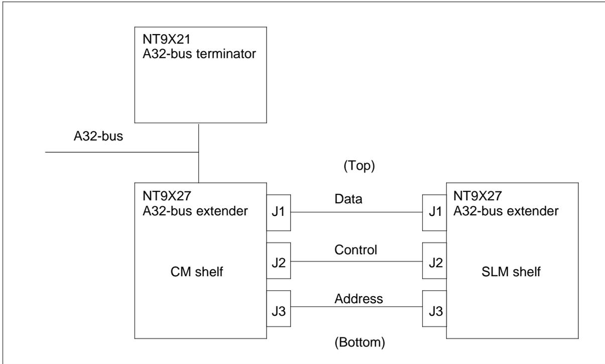
The CM can use the following NT9X27 bus extender paddle boards:
