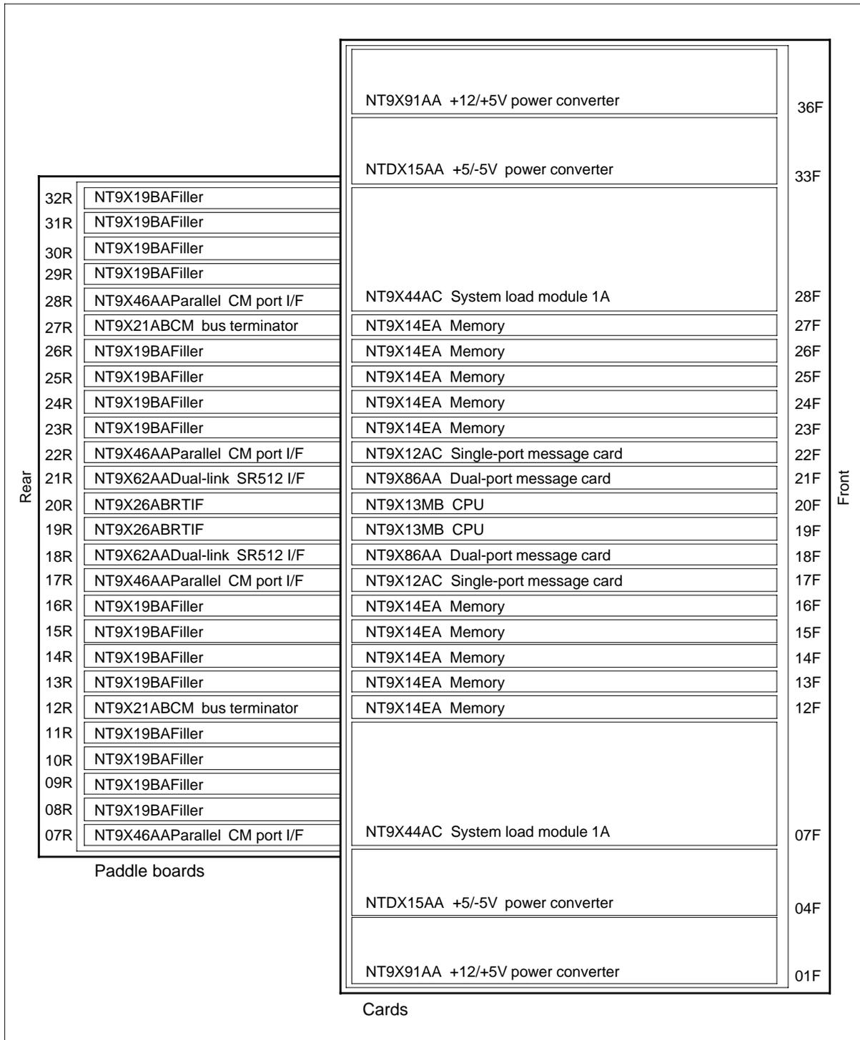
Figure 1-9 Example of a Series 50 to 70 SuperNode CM/SLM shelf layout
