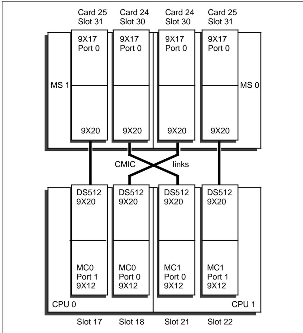
Figure 1-6 SuperNode SE CM-to-MS port connection diagram
