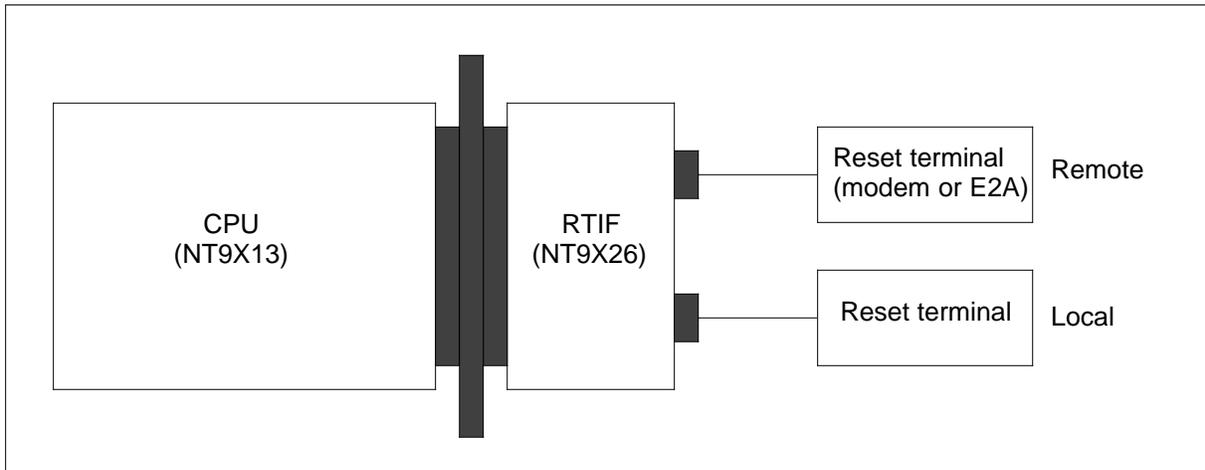
The NT9X26 card contains the OOB link interface that collects OOB reset code bits. The system assembles the bits and sends them to the CPU of the RTIF. This CPU determines the type of reset to perform. The RTIF contains a CPU, RAM, and EPROM. The OOB link between modules allows the CM to reset other nodes.
