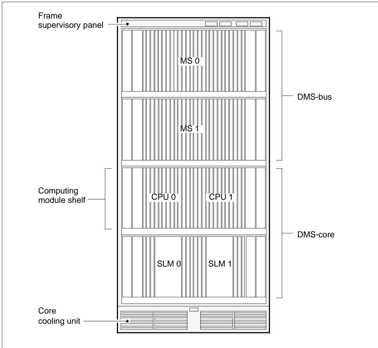
Figure 1-4 SuperNode SE SCC cabinet layout
