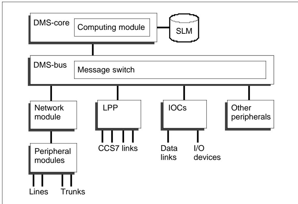
Figure 1-2 SuperNode SE system architecture
