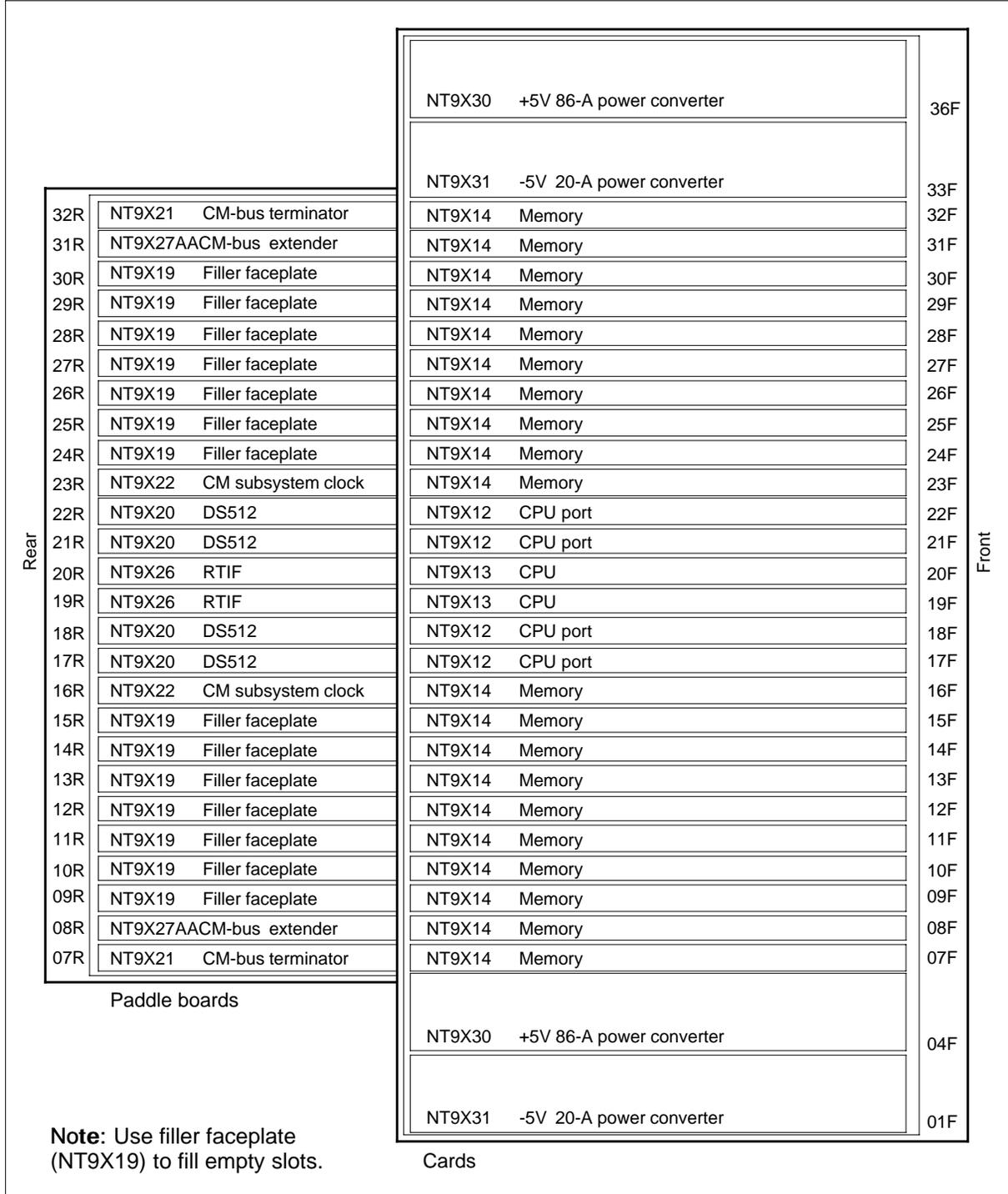
Figure 1-8 Example of a Series 20 to 40 SuperNode SE CM/SLM shelf layout
