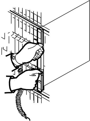
A line drawing showing a person's hands interacting with a rack-mounted card. The left hand is shown pushing the top edge of a card into a shelf. The right hand is shown pulling down on a locking lever on the side of the card. A coiled cable is attached to the bottom of the card. A rectangular box is drawn to the right of the card, indicating the area of focus. |
