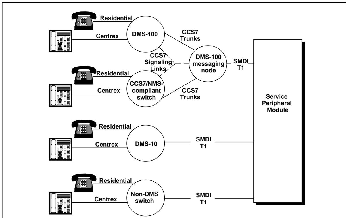
**Note:** Network Message Service (NMS) is an optional network interface for DMS VoiceMail. NMS uses common channel signaling 7 (CCS7) to offer message service to an entire city, or LATA, from a centralized DMS-100 messaging node in the network.
