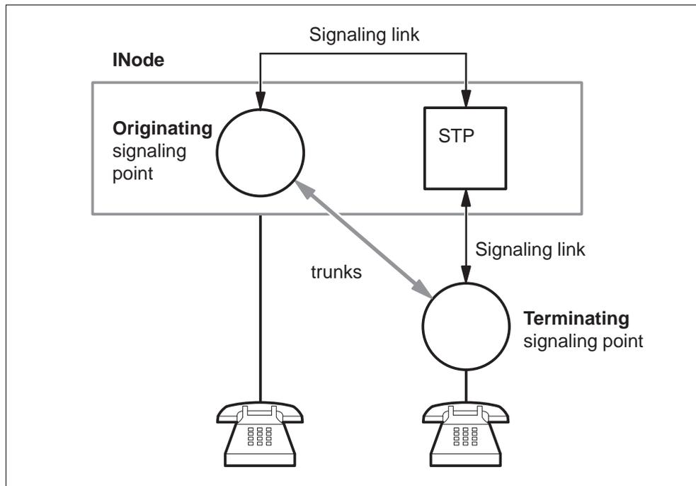
**Note:** The DMS-INode is performing an STP function in this configuration.
