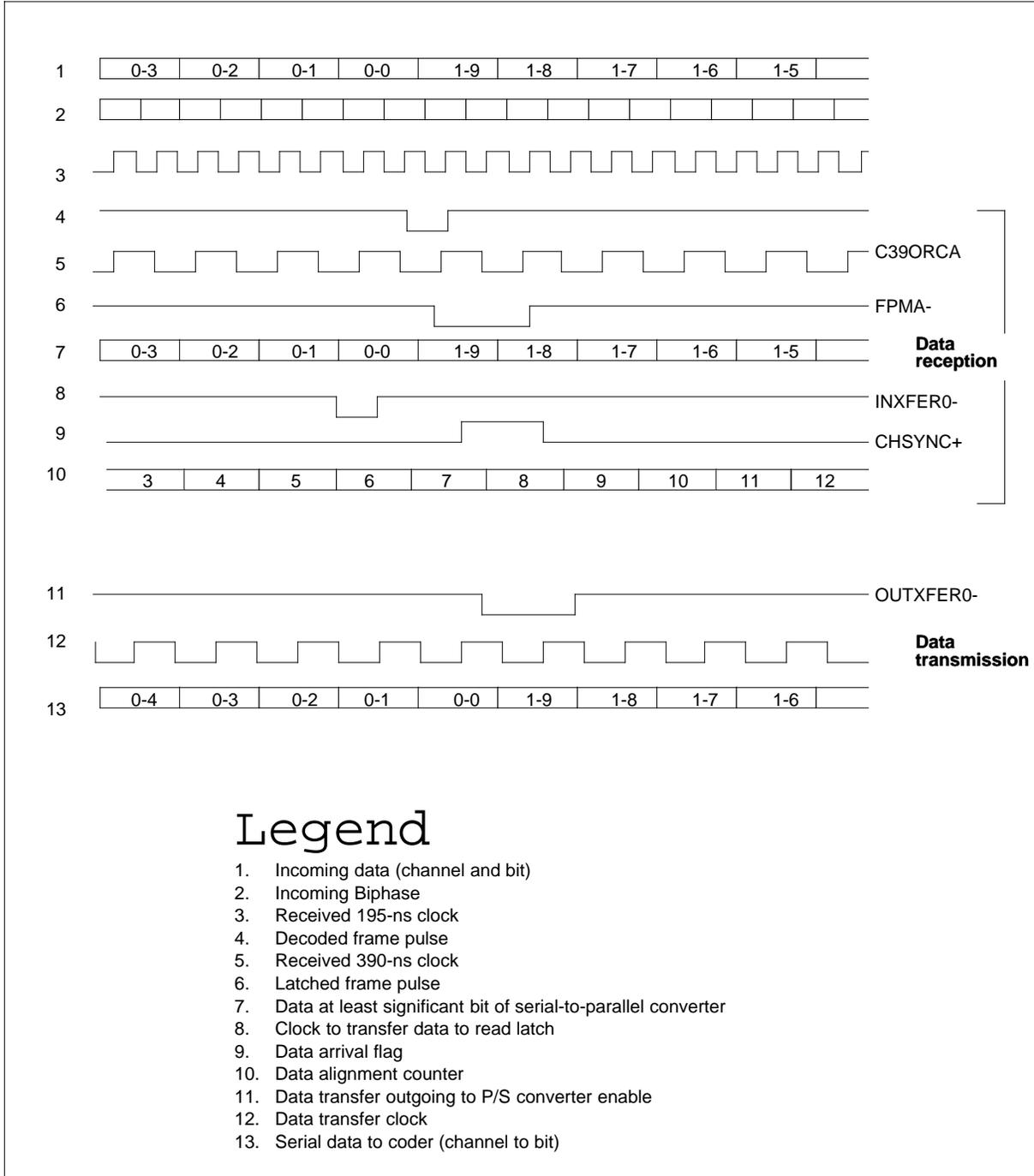
The timing for the parallel port control appears in the following figure.
