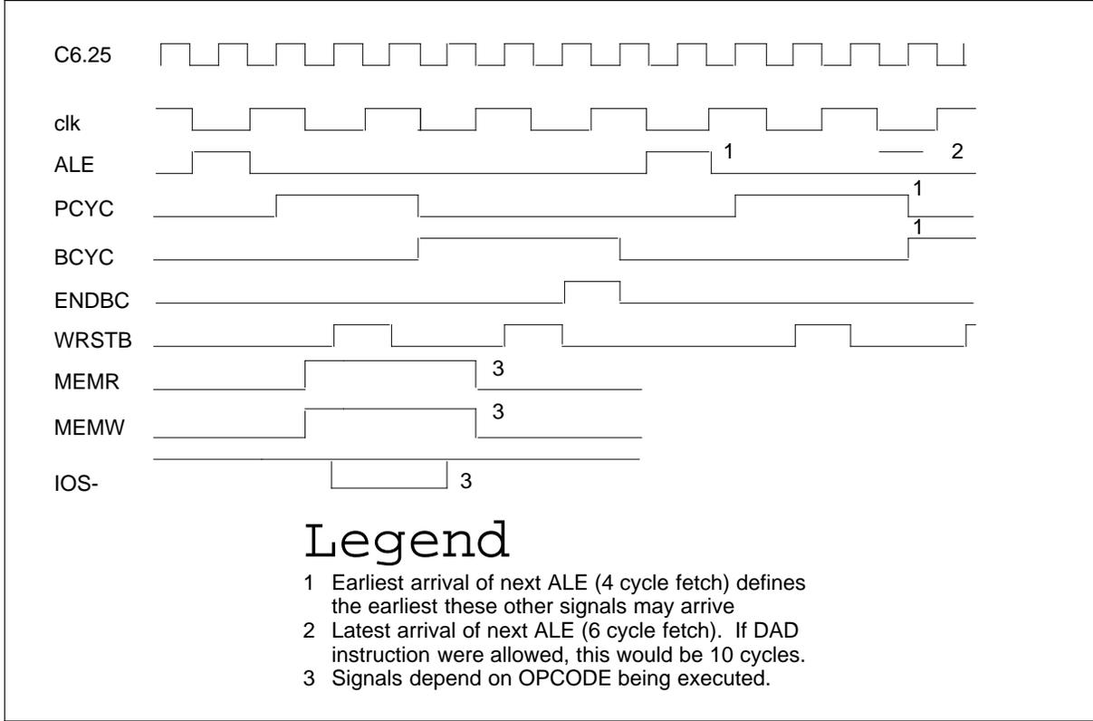
The bus control timing for the NT1X67FA appears in the following figure.
