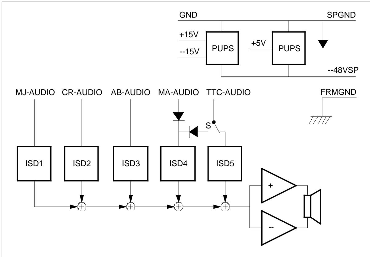
The TTC-AUDIO functional block includes a two-position switch for manual selection of ringer or chime sounds.
