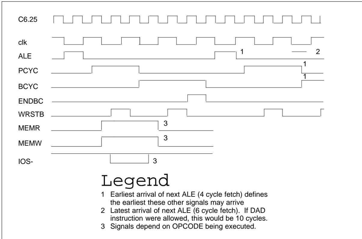
The bus control timing for the NT1X67BD circuit card appears in the following figure.
