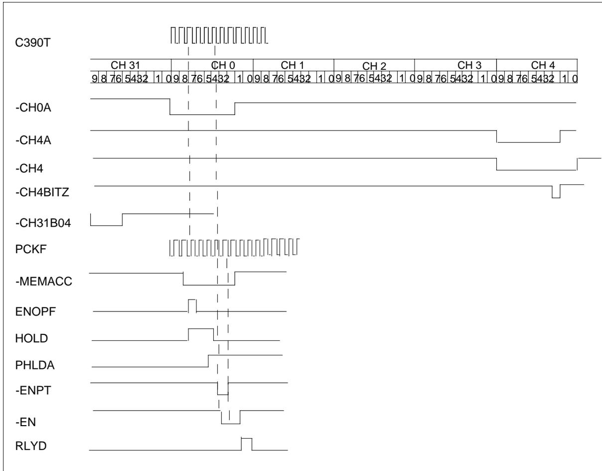
The timing required for the clock switch circuit appears in the following figure.
