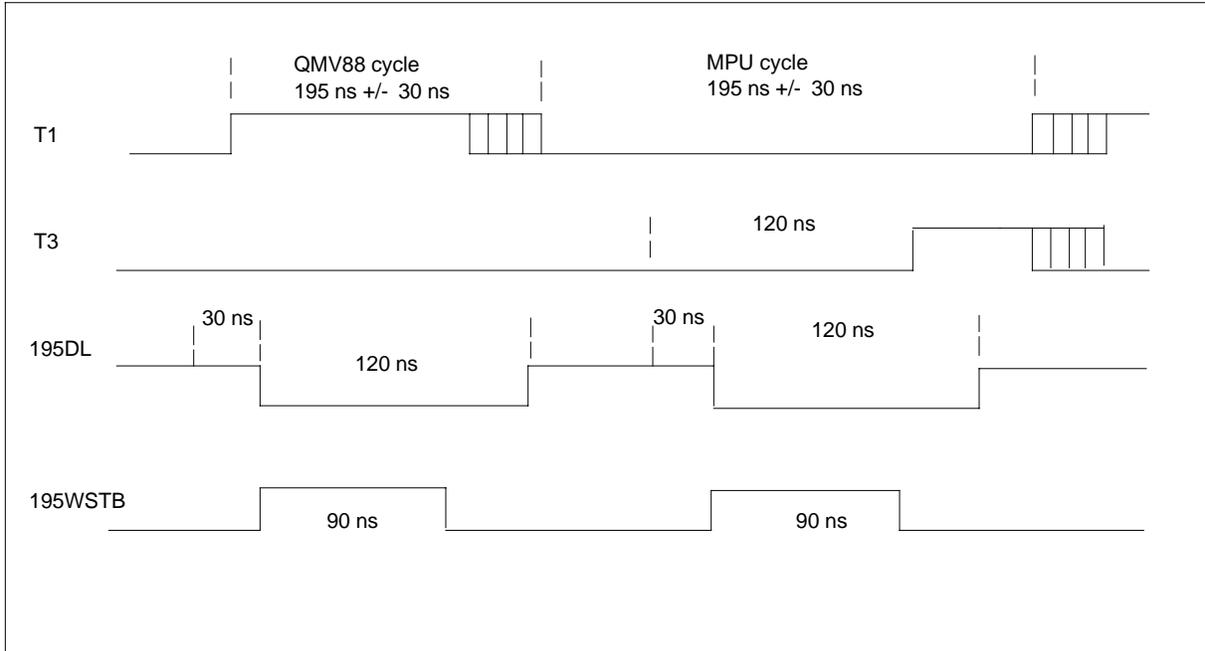
**NT1X80AA PCM\_BUFFER\_DPORT access control timing**
