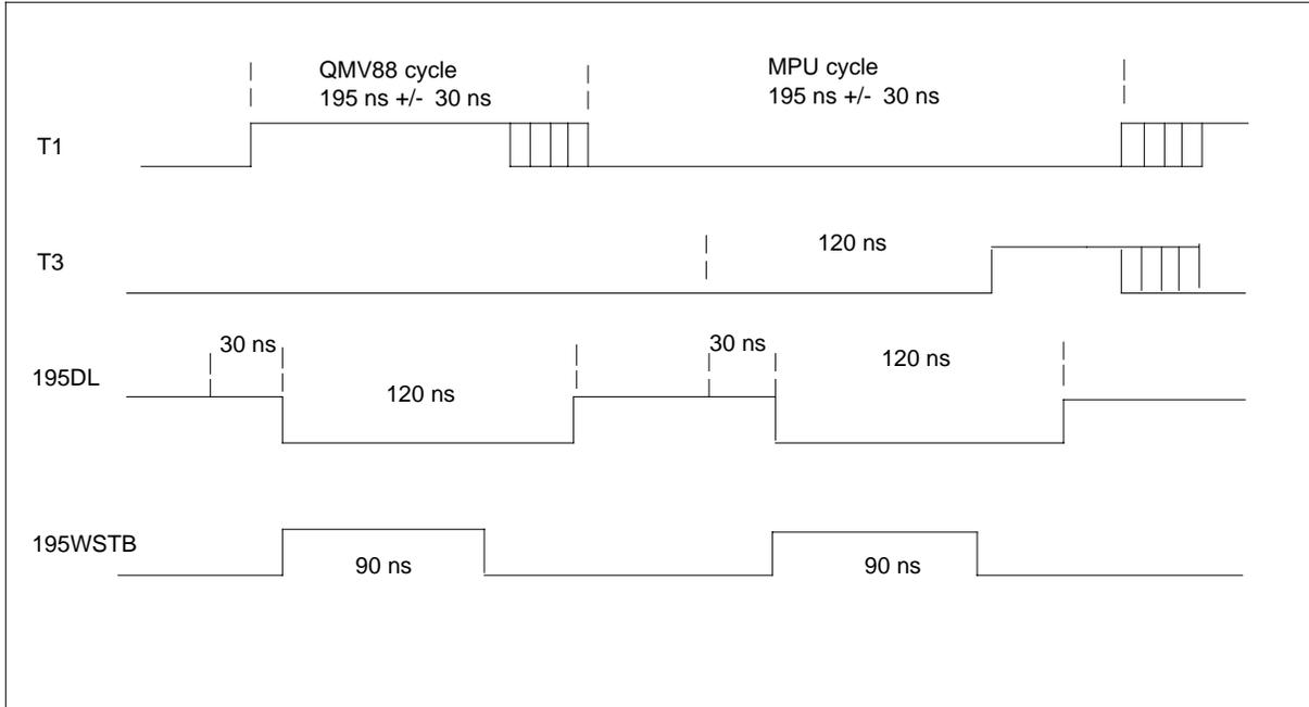
**NTIX80BA PCM\_BUFFER\_DPORT access control timing**
