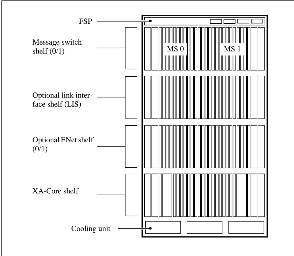
[Figure 5](#) shows the NTLX01CA EXT extension cabinet layout for XA-Core in a DMS SuperNode and DMS SuperNode SE switch.
