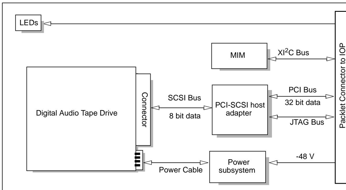
**Note:** In the NTLX07AA the tape drive has a 50-pin connector. In the NTLX07BA the tape drive has a 68-pin connector, and the SCSI bus connects to a 50-pin-to-68-pin converter.
