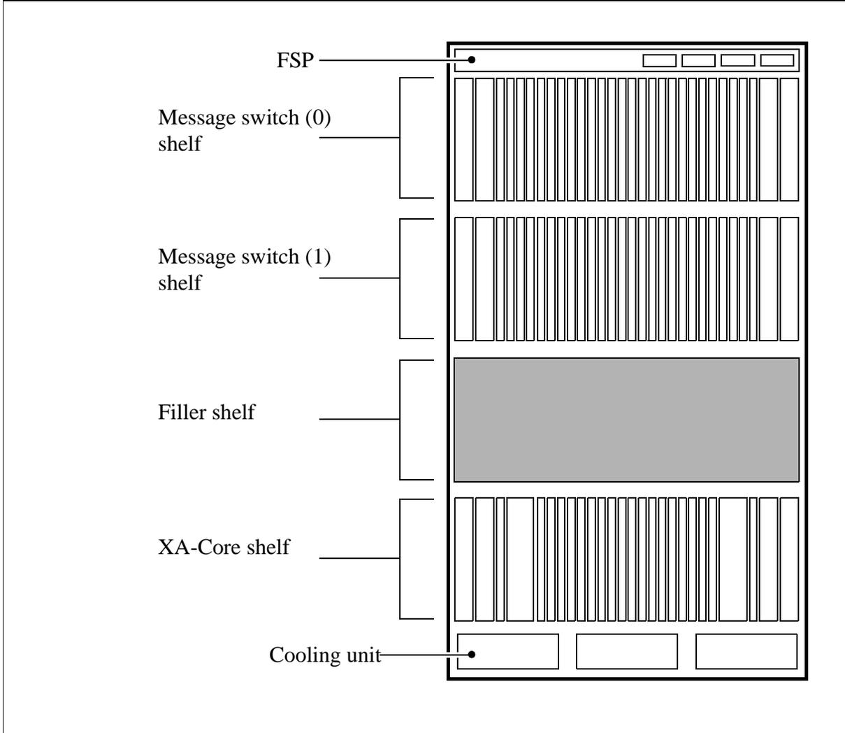
Figure 4 shows the NTLX01BA SNXA cabinet layout for XA-Core for XA-Core in a DMS SuperNode SE switch.
