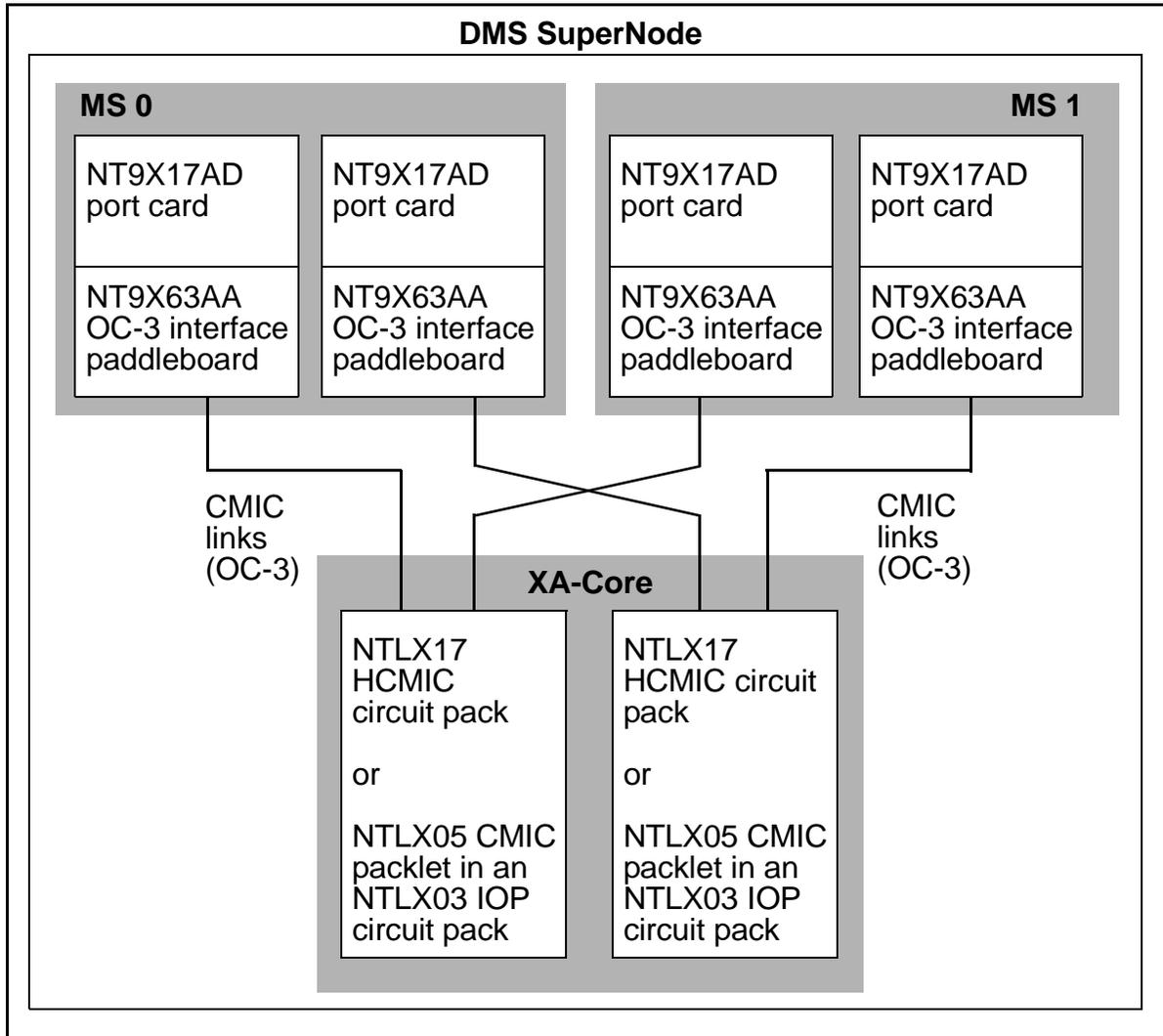
[Figure 7](#) shows the CMIC links for DMS SuperNode SE.
