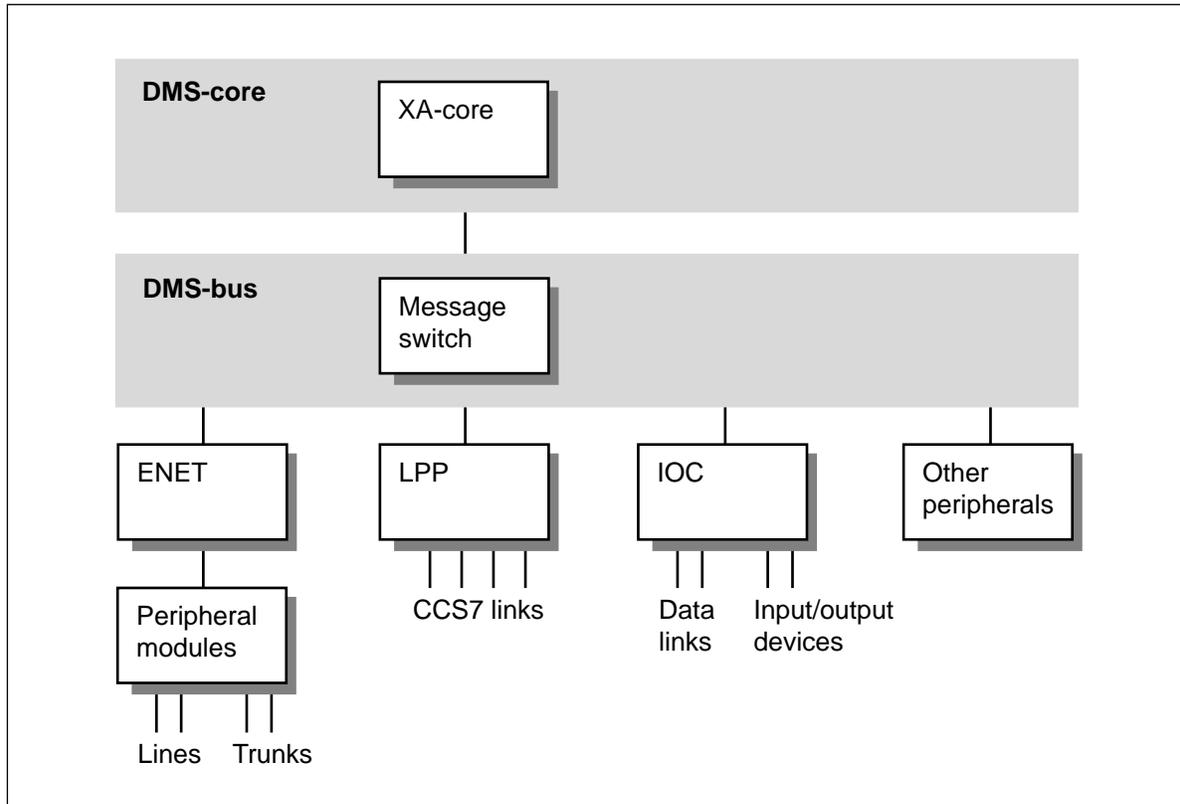
The DMS SuperNode SE can also have a 16K ENET and LIU7s. The 16K ENET provides voice and data signal switching for nodes in the DMS SuperNode SE switch. The 16K ENET also provides message routes to the MS. The LIU7 provides CCS7 message processing.
