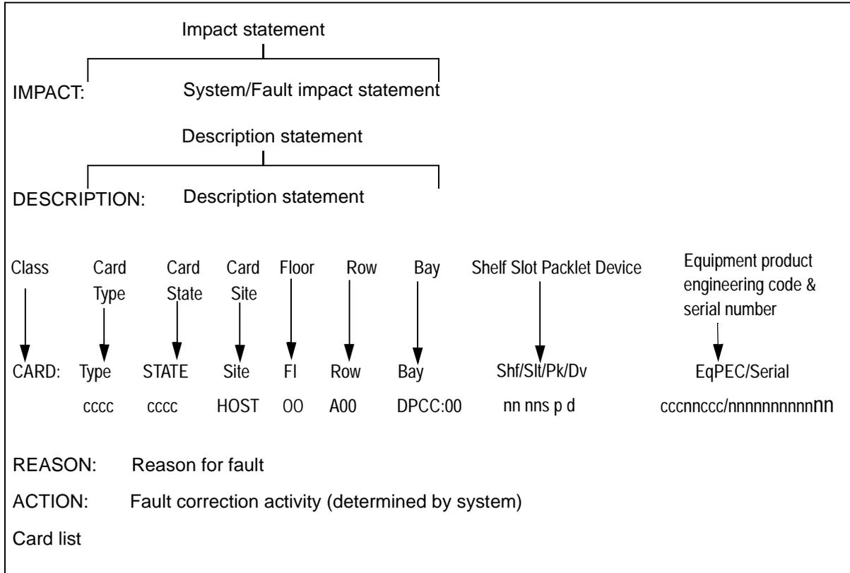
**Figure 0-2 Log body for the XA-Core information log**
