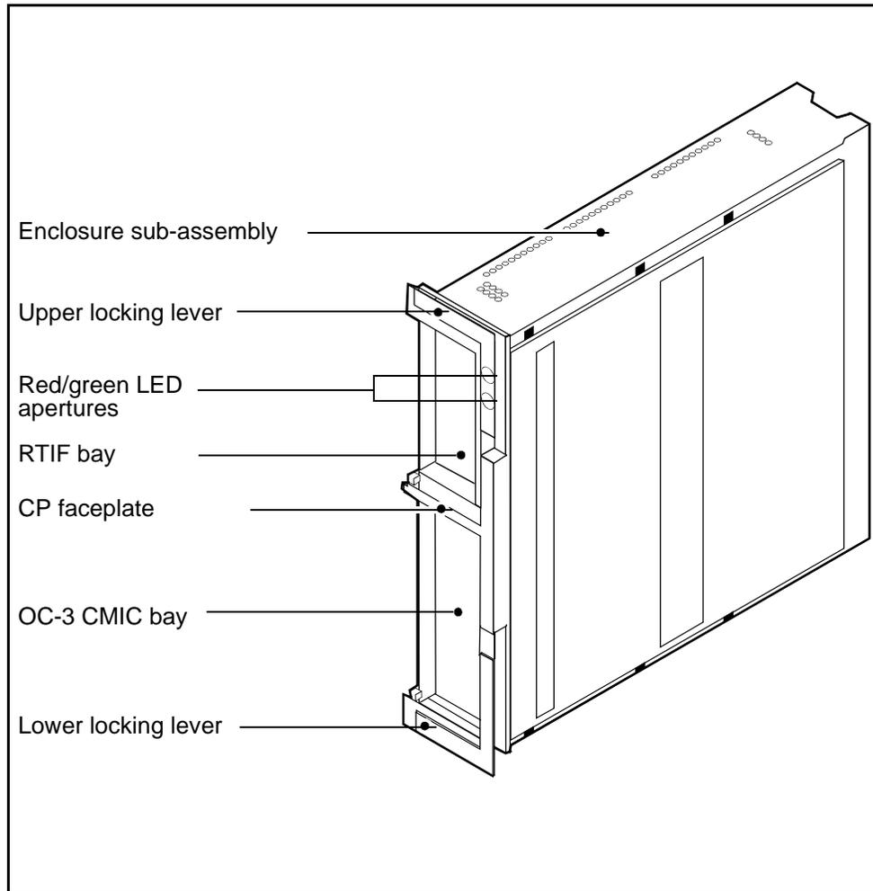
The following figure shows the external configuration of the XA-Core double width input/output processor pack.
