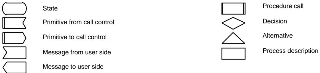
Figure 4-26 Key to Q.931 protocol control SDL diagrams
