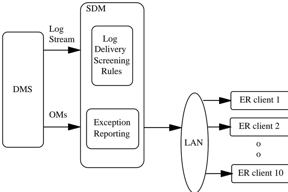
The real time usage for the exception reporting application is bursty and occurs upon the receipt of each log from the SDM as well as time triggered processing activity. The value given below is an average value for a 1 log/second delivery rate from the CM.
