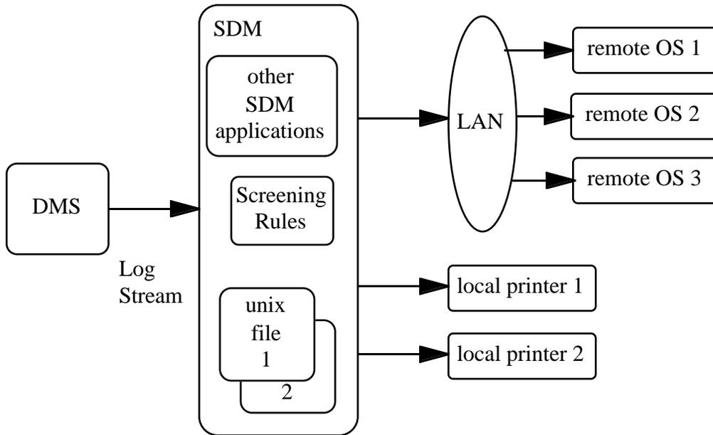
The actual real time usage for high speed logs is bursty and occurs upon the receipt of each log from the CM. The SDM CPU real time usage was measured at a rate of 1 log per second coming from the CM to the SDM and then averaged to reflect a uniform long term SDM real time usage. All the values given below are based data collected with the log delivery application running at 1 log per second.
