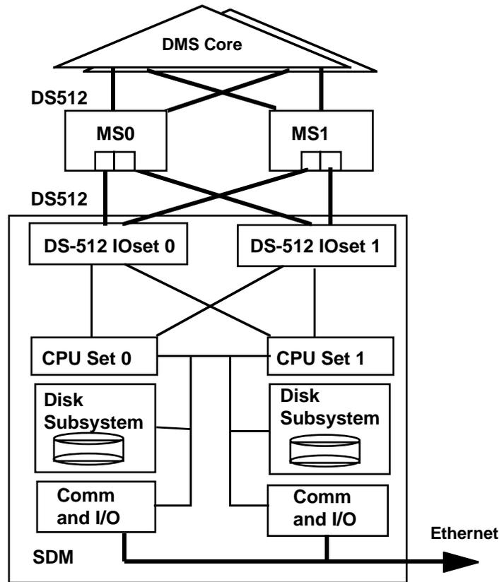
Fault Tolerant SDM/FT Block Diagram
