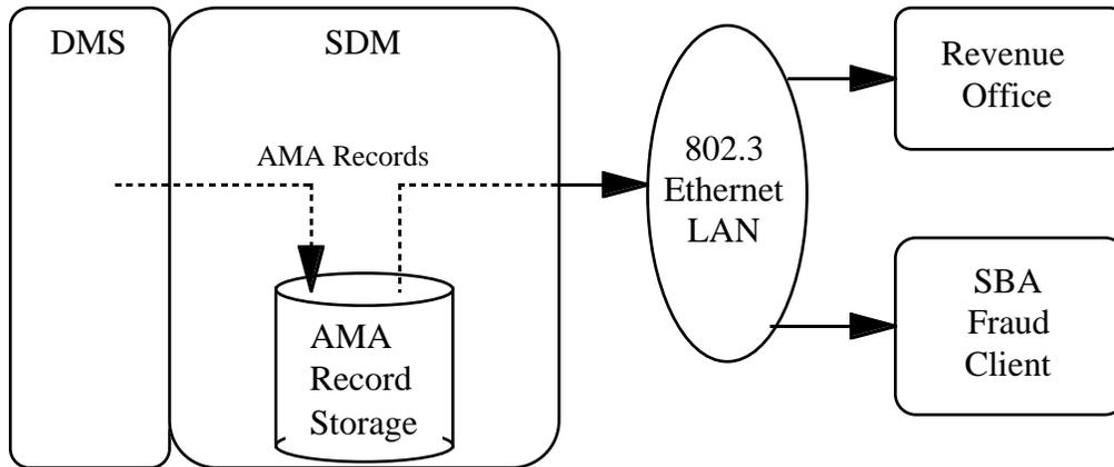
The SBA on SDMNA008 has a throughput capacity limit based on a maximum data rate of 26.7 kilobytes/second or 96.12 megabytes/hour. This capacity limit will increase in SDMNA009 and again in SDMNA011.
